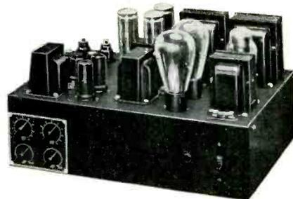
terminals provided on the input terminal connector strip the gain can be decreased from 119.5 db to 79.5 db. This adjustment is provided so that no overload will result in the event that it is desired to use the amplifier on comparatively high-gain inputs.
