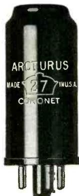
These new tubes have the regular octal 8-prong base. To permit their regular interchange with the corresponding glass tube, modernizers have been developed by Arcturus. These are being supplied with 4, 5, and 6 prong connections for adapting the old socket to an eight-prong socket which will accommodate the metal tube base.
