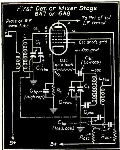
Fig. 2. Superheterodyne mixer stage.
