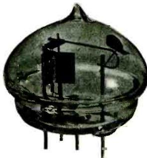
This tube, a filamentary air-cooled triode, is for use by experimenters and amateurs, and is suitable for ultra-high-frequency oscillator and amplifier applications, the frequency limit being 750 megacycles (approx. 0.4 meter).
