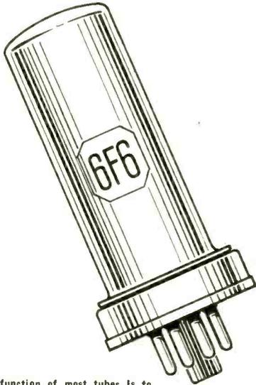
Normally the function of most tubes is to amplify a signal. But when tubes are required to deliver power, such as the 6F6, the amplification may test up and yet the tube may distort badly. Reason . . . weak emission . . . particularly at low frequencies. Such tubes demand both amplification and emission test, now available . . .
