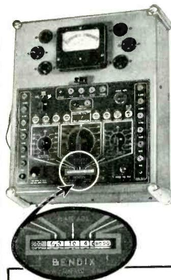
—any portion of the electrical continuity which may be at fault. It has an exclusive Safety Tube-Index Dial which eliminates the danger of blowing out tubes.
