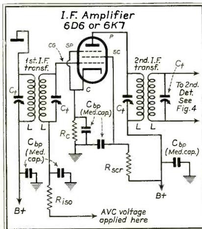
Fig. 3. An i-f amplifier stage.
