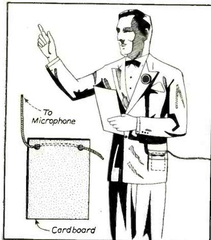
microphone cable and also reduce the pull on the cable.
