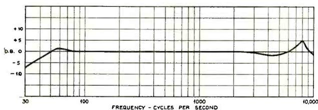
Fig. 2. Overall amplifier response.
