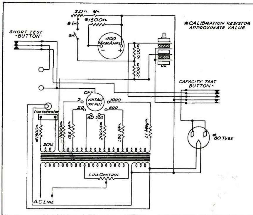
Fig. 4. Triplett 1240 condenser checker circuit.
