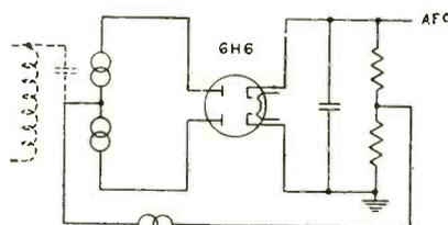
Fig. 2. Placing a-c voltages in series.
