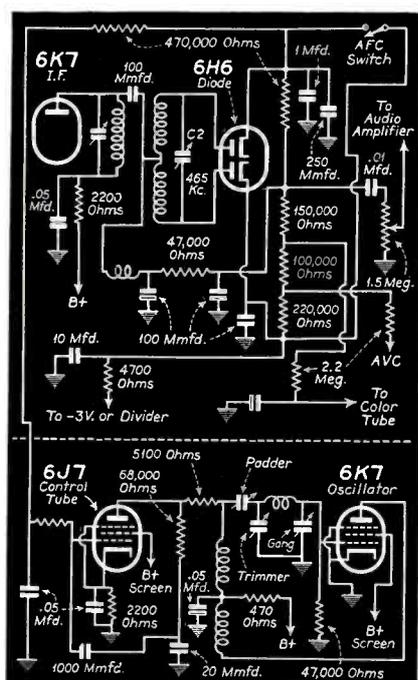
Fig. 1. Complete afc circuit.
