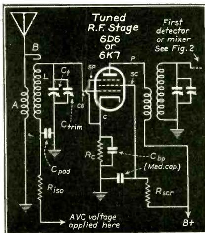
Fig. 1. A typical t-r-f stage.
