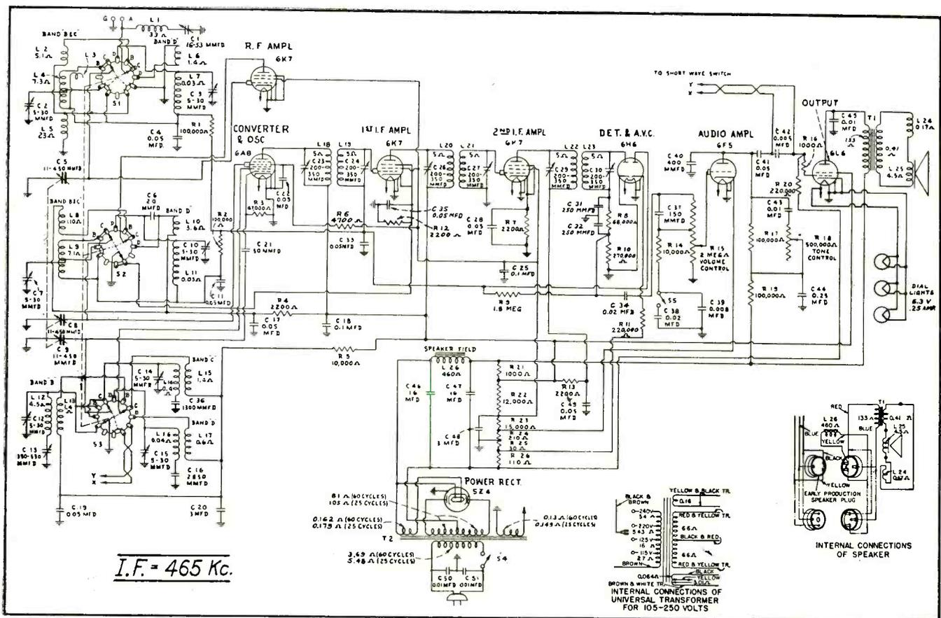
Fig. 1. General Electric E-81 and E-86 circuit.
