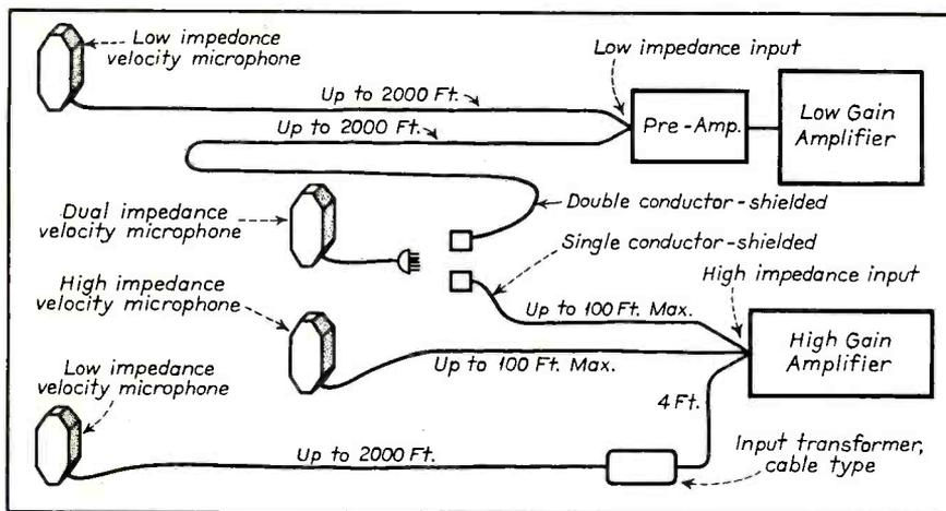
Fig. 5. Velocity microphone connections.
