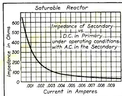
Fig. 2. Change in secondary reactance vs. primary current.
