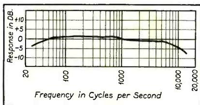
Fig. 1. Response characteristic of velocity microphone.
