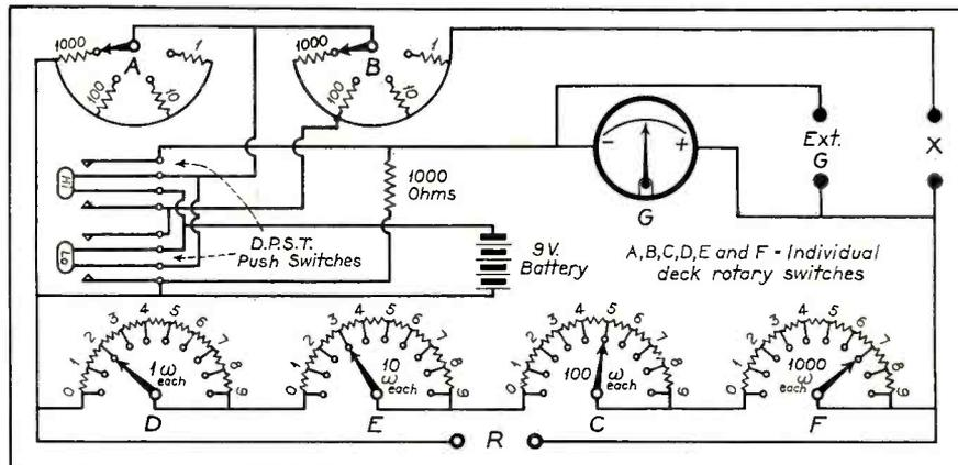
Fig. 2. Wheatstone bridge circuit.
