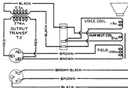
Fig. 4. RCA speaker connections.
