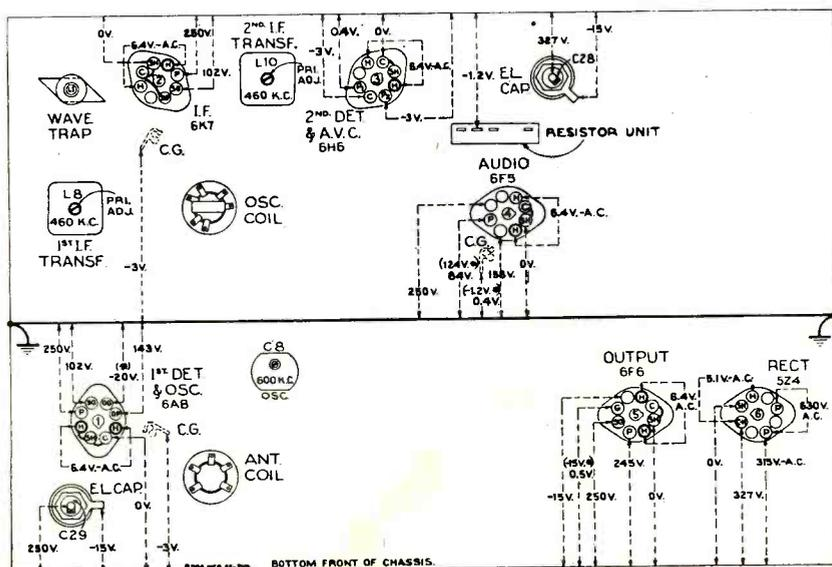
Fig. 2. Socket voltages and trimmer locations.
