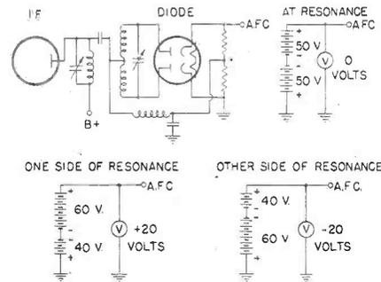
Fig. 6. The a-fc discriminator circuit.
