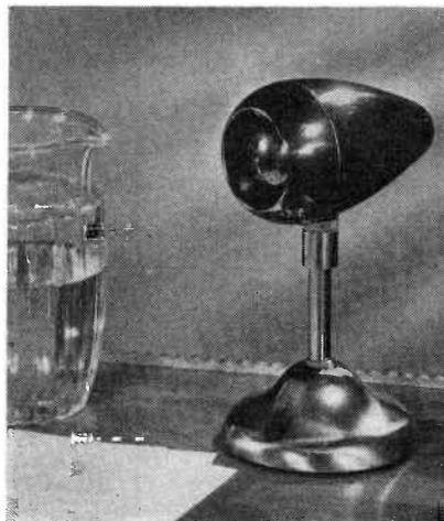
Fig. 2. The bullet microphone.
