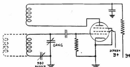
Fig. 2. Conventional oscillator circuit.
