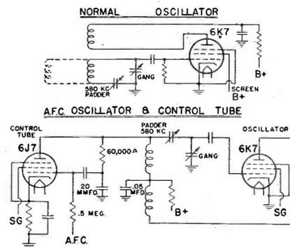
Fig. 4. The afc oscillator circuit.
