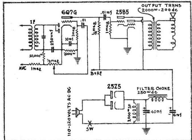
Fig. 7. Schematic diagram of audio amplifier and power supply of set "D" converted for 25B5.
