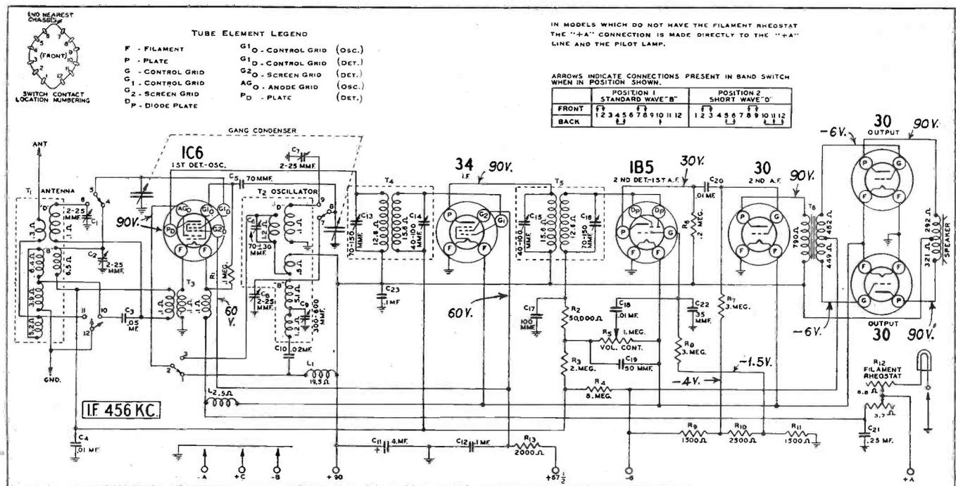
Fig. 1. Wells Gardner 6G circuit diagram.
