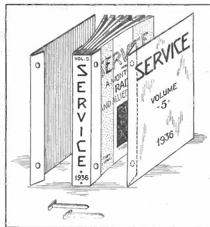
ume may be made in the manner indicated in the accompanying illustration. Two hard covers slightly larger than the magazine are cut from cardboard, fibre or some similar material. On one end of each a narrow strip, about 1/2 inch wide, with holes as indicated, is attached using a flexible binding tape. A third section, wide enough to cover the twelve issues, also has two narrow strips attached.
