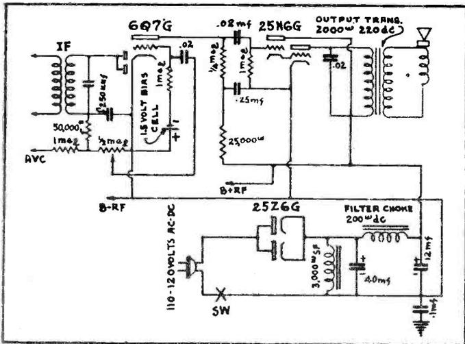
Fig. 5. Schematic diagram of audio amplifier and power supply of set "B" converted for 25B5.
