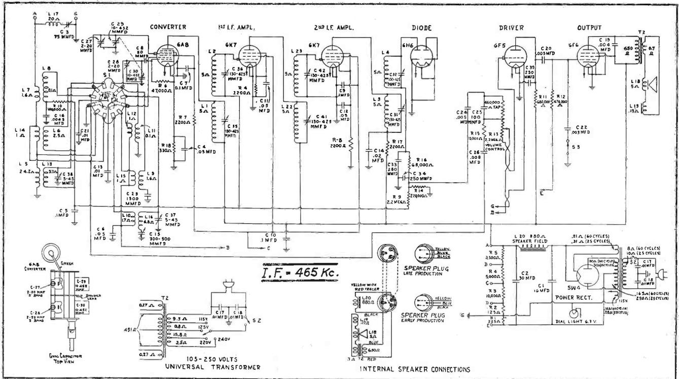
Fig. 1. General Electric E-71, E-72 and E-76 circuit diagram.
