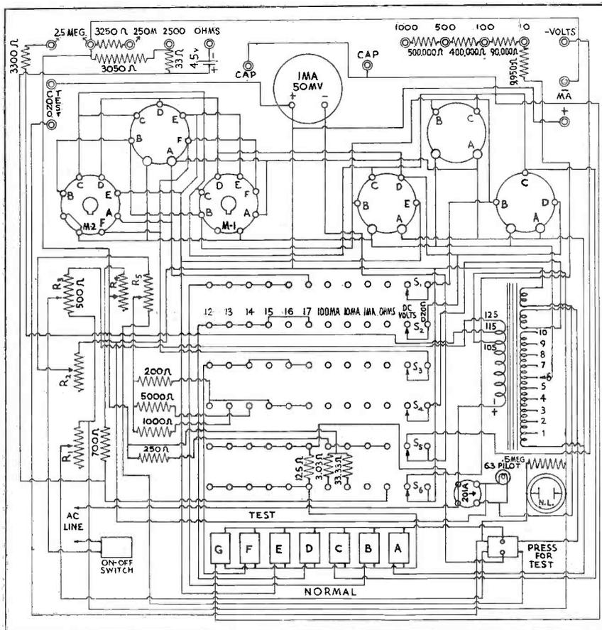
Fig. 1. Precision series 600 Electronometer circuit.
