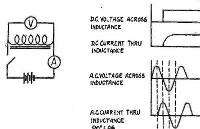
Fig. 3. The current lags the voltage in an inductance.
