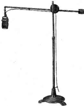
microphone can therefore be placed at any height and at any angle desired. No adjusting screws are required. This action is obtained by using a ball clutch for the vertical adjustment. Such a stand is useful in placing microphones in unusual positions such as for soloists playing at the piano, or whenever quick change in the microphone position is required. Obtainable in chrome or gunmetal finish.
