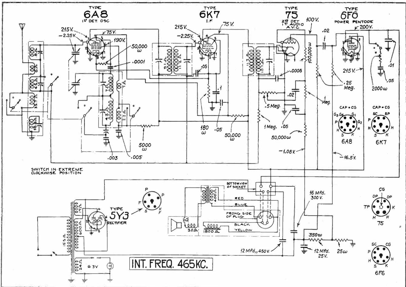
Fig. 1. Bosch 605-605C circuit diagram.
