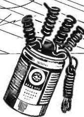
A new CONTINENTAL Carbon main line noise Filtercon, designed to be installed on your supply line at the fuse panel, blocks power line interference before it can spread through the house wiring. This Filtercon, F1005DH, is a heavy-duty inductive and capacitive filter, rated to carry 10 amperes at 110 or 220 volts. In addition to its use as a main line filter it is suitable for blocking noise of large household or store electrical equipment. List price is \$5.00.
