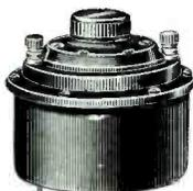
An efficient permanent magnet horn unit requiring no outside excitation. Aluminum nickel steel magnets are used to supply maximum flux density in the air gap. Cast bronze case, completely enclosed, making Unit water tight.
