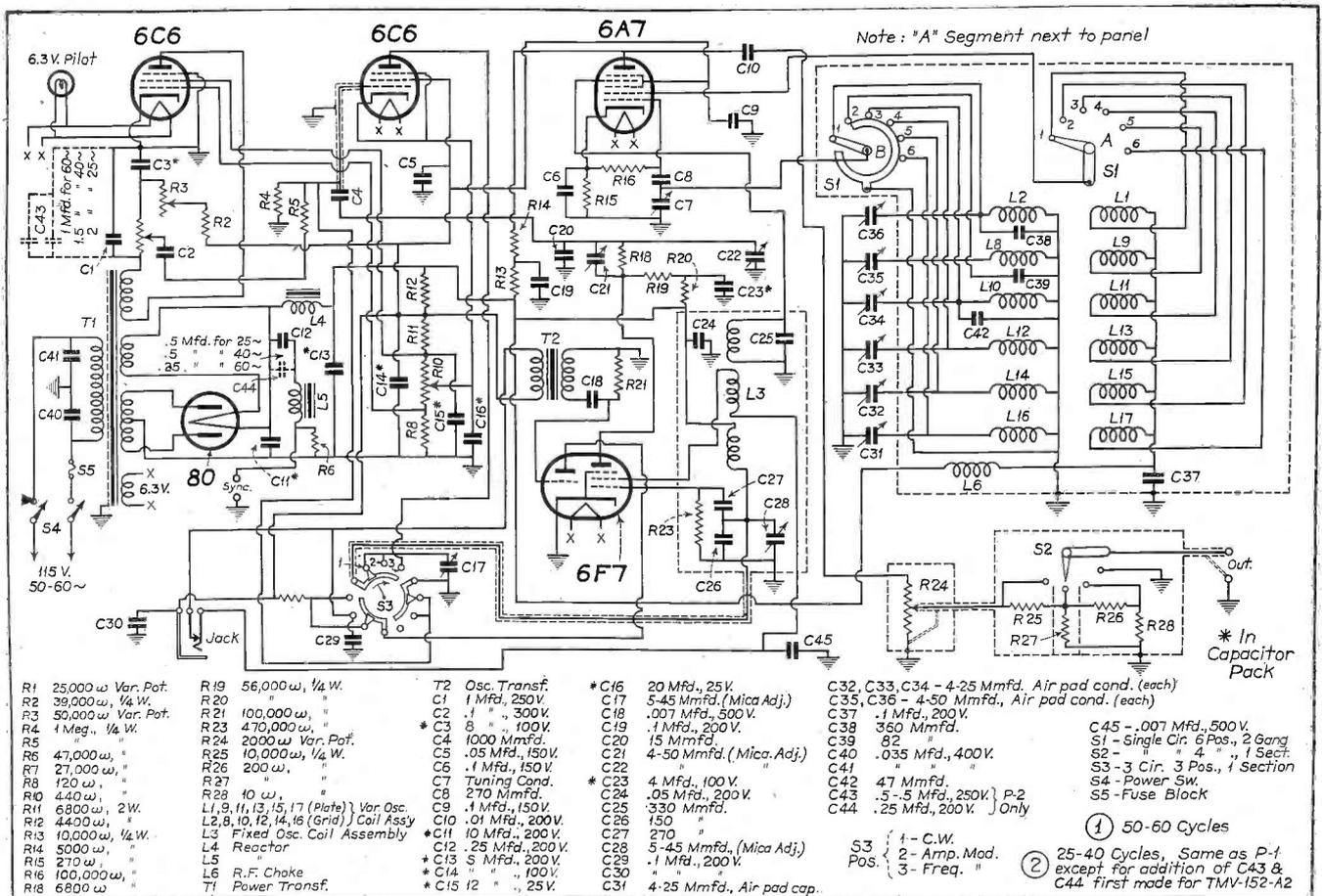
Fig. 6. The RCA model 150 test oscillator circuit diagram.
