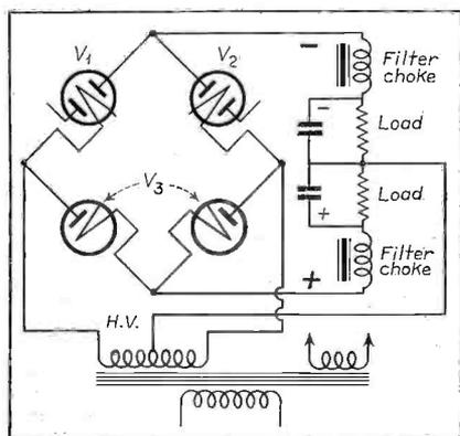
Fig. 1. Stabilized bridge type rectifier system.
