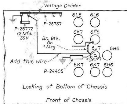
This modification was put in effect at the factory in all 160-P and 180-L receivers, and in all 160-L produced after October 23, 1936.
