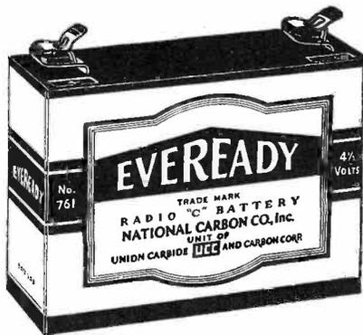
This is a No. 761—4½-volt *General Purpose* Battery. The size and composition of the cells in this battery make it suitable for such purposes as filament current supply for two 2-volt tubes in series, microphone battery, relay battery, and other uses where the No. 771—4½-volt Radio "C" Battery is not recommended.
