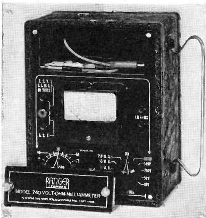
volt; (d-c accuracy 2 per cent, a-c, 5 per cent) 1-10-50-250 d-c milliamperes; 0-300 low ohms; high ohms to 250,000 at 1½ volts. Provision for higher resistance readings by addition of external batteries.
