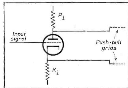
Fig. 4. Direct-coupled signal divider circuit.
