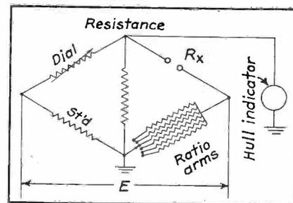
Fig. 6. Resistance measurement with the bridge.
