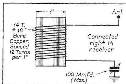
Fig. 1. Series wave trap.
