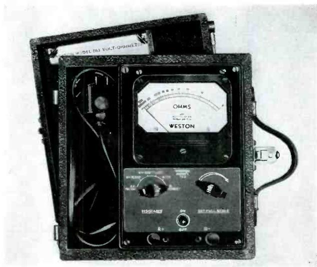
A combination instrument in which a high-sensitivity meter permits measurement of high resistances.
