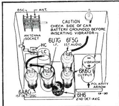
Wells-Gardner C6-A, C6-B chassis layout showing locations of tubes and trimmers.
