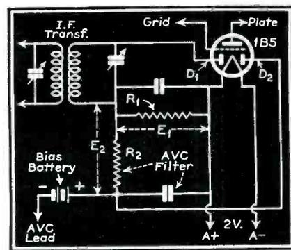
Fig. 4. Delayed avc circuit using the 1B5 type tube.
