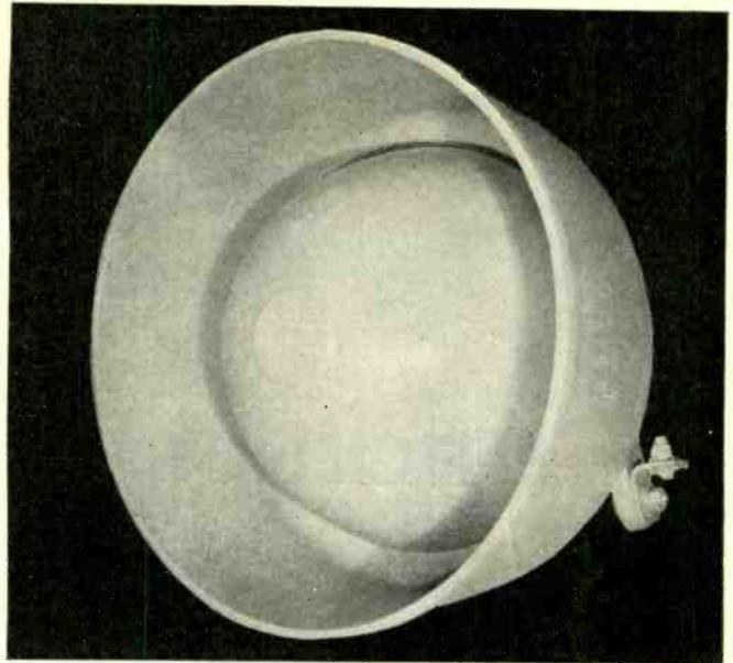
Fig. 3. The Western Electric Bull Horn. The response has been restricted to between 400 and 4000 cycles. A high efficiency dynamic unit works into a reflex horn; 500 watts can be handled at an efficiency of 50 per cent.
