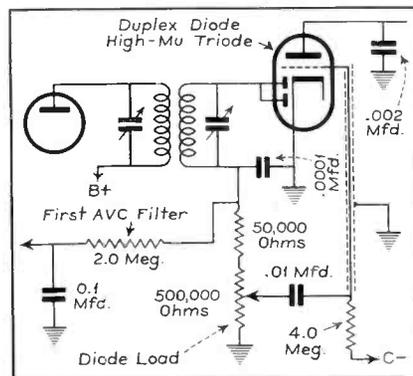
Fig. 2. The diode load circuit of a typical modern receiver, showing the large avc filter resistor and the large first a-f grid load.
