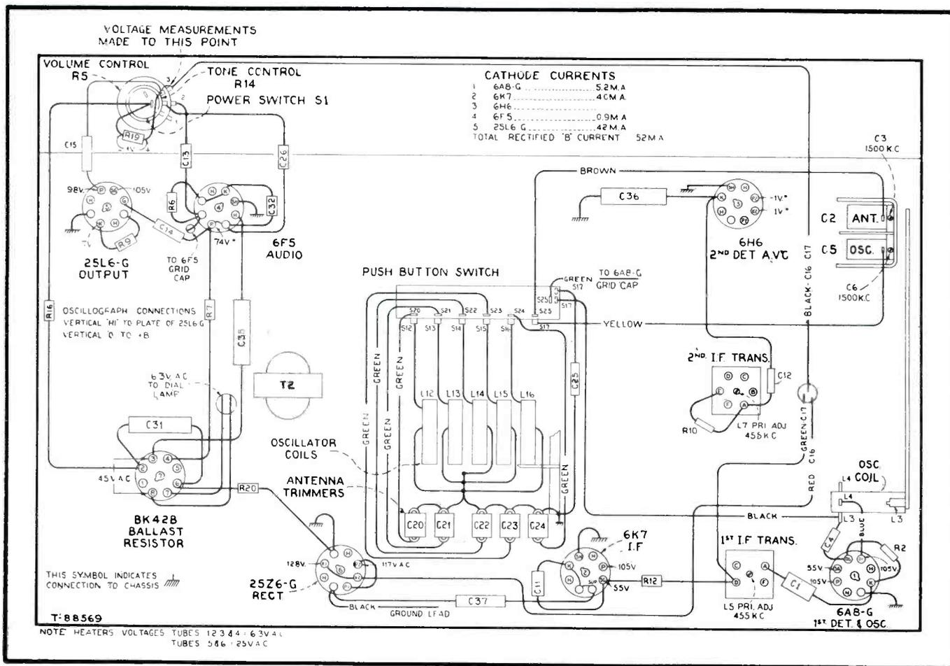
RCA 97X parts layout and chassis wiring. Voltage values measured from the low side of the volume control.
