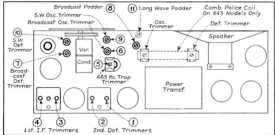
Fig. 2. DeWald 636, 636-S, 636-LW, 636-LW-S, 643, 643-LW parts layout and trimmer locations.
