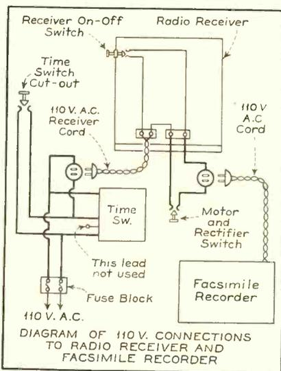
Fig. 4. During daylight and evening hours the time switch can be taken out of the circuit by operating the shunting switch to the on position. Application of power to the receiver is then controlled in normal manner with the regular off-on switch.
