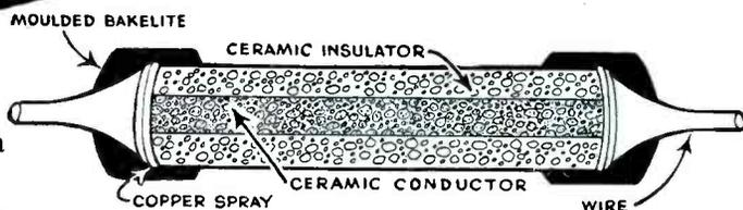
*Baptized in fire at 2500 degrees . . . hard as stone. Center ceramic core, and ceramic jacket fired together to form a single shock-proof unit. Pure copper covers resistor end for wire lead contact.*
