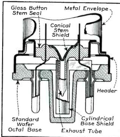
Fig. 1. The new constructional design of the tube base (above) allows the grid lead to be brought out at the base of the tube. The resulting single-ended metal tube employs the familiar octal socket shown to the left. Loktal tubes are also single-ended but are all glass and use the socket shown to the right. The bulb shapes and dimensions are shown below.
