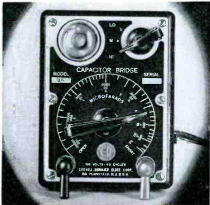
The Cornell-Dubilier type BN capacitor bridge is a compact instrument designed chiefly as a direct reading device for the service bench.
