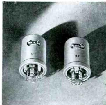
for service work. A new type of mounting is incorporated with base prongs which fit chassis slots and are fastened by twisting. Additional information on these and other Solar capacitors may be obtained directly from Solar.
