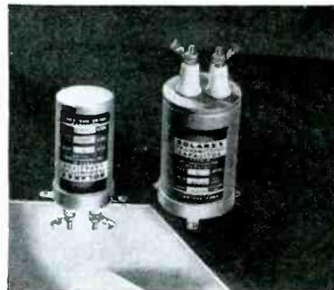
capacitor for general amateur transmitter use. This unit, available in standard values, is built of paper sections which are oil-impregnated under high-vacuum. They are assembled in insulated round metal cans, oil-filled and hermetically sealed. Terminals are porcelain stand-off insulators. Mounting is accomplished by means of detachable rings.
