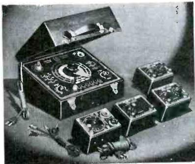
The Cornell-Dubilier capacitor test equipment line includes the Model BF50 capacitor analyzer, the Model BN midget capacitor bridge, and a series of three direct reading capacitor decades, the types CDA, CDB and CDC. The latter are standards of  $\pm 5\%$  and  $3\%$  tolerances. Cornell-Dubilier Electric Corp., S. Plainfield, N. J.
