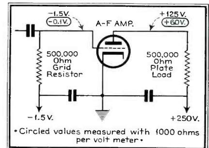
Fig. 2. Older type voltmeters load the circuit heavily and incorrect readings are obtained. With a modern instrument the actual voltages are indicated.
