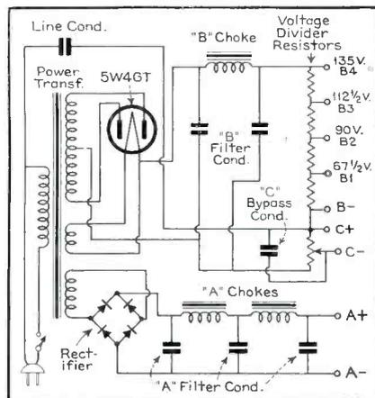
Taps are provided on the Porta Power for various A, B and C voltages.
