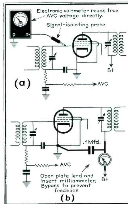
Fig. 1. A modern electronic voltmeter (a) measures the actual control voltage at the grid. Without it the measurement must be made by indirect methods (b).
