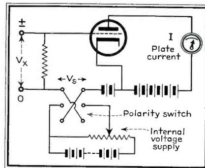
**Fig. 5. In the slideback type voltmeter the plate current meter indicates when the internal and external voltages are equal.**
