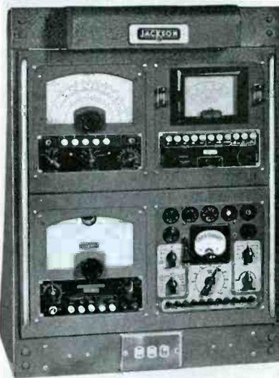
and panel mounting. These units are: Model 640 all-wave oscillator, provides
