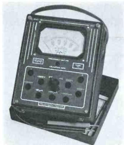
Triplet Model 1280 kilovolt tester. A 25,000-ohms-per-volt instrument with special ranges for voltages up to 10,000 and currents as low as 1 microampere.
