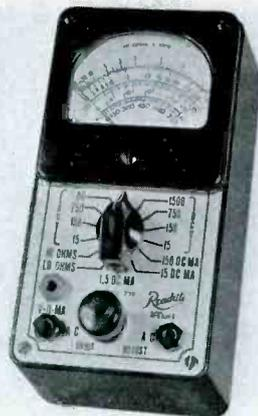
Readrite Model 739 pocket volt-ohm-milliammeter. Has 13 ranges for 4 functions.
