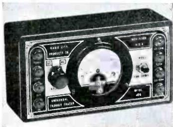
Radio City Products Model 456P general utility meter. An a-c, d-c multi-meter with a 1-ma D'Arsonval movement. Sixteen ranges provided for 5 functions.
