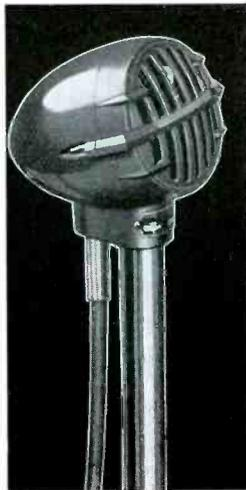
This semi-directional crystal microphone of contemporary design, fills a long standing demand for a really good, low priced microphone for universal use. New, massive cartridge, freely suspended, within housing makes this microphone dead to vibrophonics. Output -52 db. Wide-range (JT-30) and voice-range (JT-40) models. Choice of three finishes.
