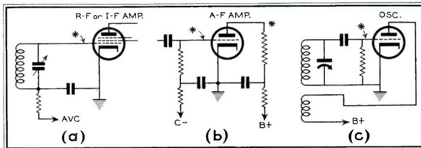
**Fig. 7. With the probe shown in Fig. 8 it is possible to measure the operating voltages in the (typical) circuits shown.**
