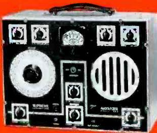
MODEL 562—The need of a fast, simple, inexpensive, but complete dynamic testing instrument prompted the design of the Model 562. With it one probe can be used to localize trouble in any receiver. A built-in voltmeter with an input impedance of 15 megohms allows measurements in grid, A.V.C., A.F.C., or any other circuit without affecting the operation of the set. A built-in speaker offers an audible system of testing which is the simplest and fastest yet devised.
