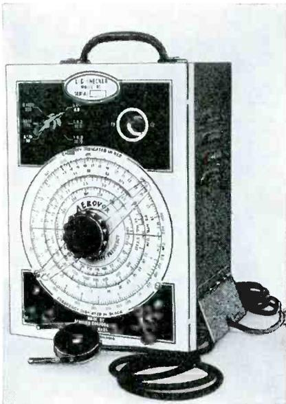
The line cord and loop of the Aerovox 95L-C checker can be housed in a neat compartment on the side of the instrument.
