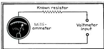
**Fig. 3. Early voltmeters were made by connecting a milliammeter in series with a resistor of known value. The scale was calibrated directly in volts.**
