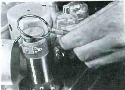
The L-C checker can be used to determine the resonance point of tuned circuits.
