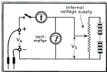
**Fig. 4. The internal voltage of the potentiometer type voltmeter is varied until zero deflection on the galvanometer indicates that it is equal to the external voltage  $V_x$ .**
