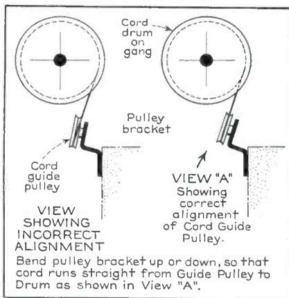
**Correct alignment of the dial-string guide pulley is important for trouble-free operation of the dial drive.**
