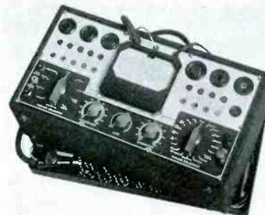
Model 1604 set tester. D-c volts to 2,500, at 25,000-ohms-per-volt, in 6 ranges; a-c volts to 2,500, at 1,000-ohms-per-volt, in 6 ranges; d-c from 50 microamperes (full scale) to 20 amp in 9 ranges; resistance to 20 meg in 5 ranges; capacity and db ranges. Complete tube testing facilities. Lifetime guarantee. Triplet Electrical Instrument Co., Bluffton, Ohio.
