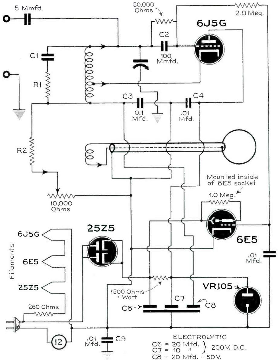
**A type 6E5 visual indicator tube is used as a grid-dip indicator in the L-C checker.**
