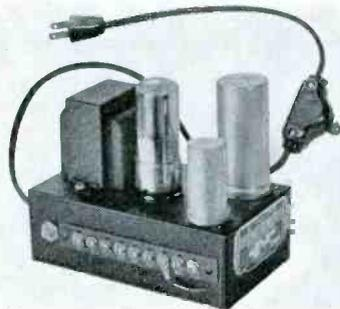
The GTC Model L Porta Power supplies power for 2-volt sets from the 60-cycle a-c power lines.
