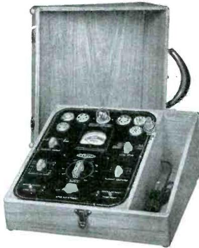
tube testing facilities. In addition, Christmas tree bulbs, pilot lights and plug-in resistors may be checked. Consolidated Wire & Associated Corps., 518 S. Peoria St., Chicago.
