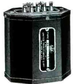
**VT-1**—This Varitone is incorporated with a universal audio transformer. Two primaries are provided. One is suitable for working from a single or double button microphone a low impedance pickup, or a line; the other primary is designed to work out of the plate of a tube or from a high impedance pickup. The secondary winding is centertapped and is equally suitable for working into one or two grids. Net price..... **\$5.10**
