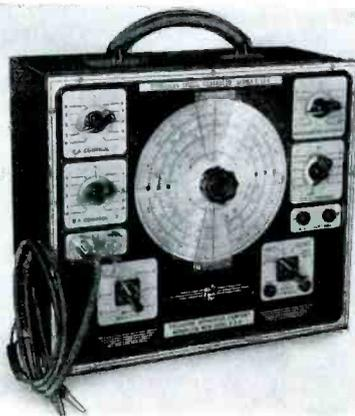
Precision Series E200 signal generator. Incorporates avc substitution method for mc in 6 bands, modulated or unmc in 6 bands, r-f or modulated.
