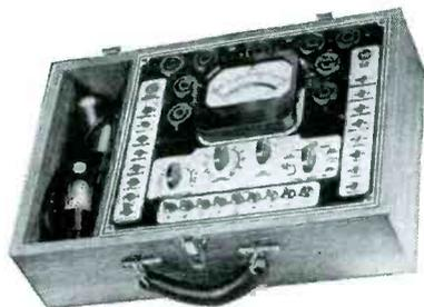
Model 774 Checkmaster. Provides complete tube checking facilities as well as voltage measurements to 1,000 volts, in both a-c and d-c, in 5 ranges; output measurements to 1,000 volts, a-c, in 6 ranges; direct current measurements to 100 ma in 3 ranges; and resistance measurements to 10 meg in 4 ranges. Equipped for use with Weston 666-1B socket selectors and test leads. Weston Electrical Instrument Corp., Newark, N. J.
