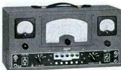
Jackson Model 660 dynamic signal analyzer. Designed for quantitative as well as qualitative measurements of r-f and a-f signals at any point in the receiver.
