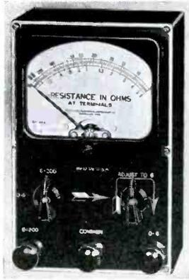
Hickok low-range ohmeter. Has 2 ranges: 0 to 6 ohms and 6 to 200 ohms. Since resistance of leads must be considered on these low ranges readings are specified as at the meter terminals.
