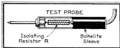
**Fig. 8. The isolating resistor placed close to the probe point prevents the capacitance of the test leads and voltmeter input circuit from reacting on the circuit under test.**
