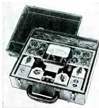
Model 801 combination tube and set tester. Has complete tube testing facilities. Provides, in addition, 26 ranges for set testing. These are: 4 ranges, to 1,000 volts, in a-c and d-c volts at 1,000-ohms-per-volt; 5 direct-current ranges to 10 amp; 4 ohm-meter ranges to 10 meg, plus 5-ohm center-scale range; db and output ranges. Radio City Products Co., 88 Park Place, New York City.
