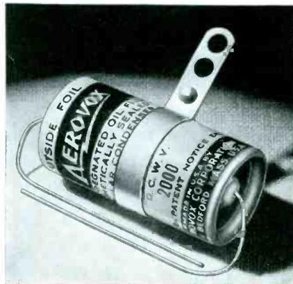
nished-paper jacket with spun-over ends, and a center mounting strap. Available in 400 v, 600 v, 1,000 v and 2,000 v ratings in capacities from 0.006 to 0.5 mfd. Aerovox Corp., New Bedford, Mass.
