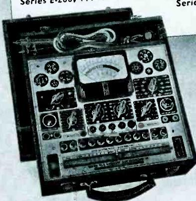
★ Series 954 Combination Dynamic Mutual Conductance Type Tube Tester and 20,000 ohms per VOLT Multi-Range AC-DC Set Tester
