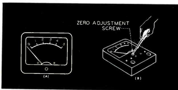
Fig. 2. How to correct for "zero shift." If the pointer is "off zero" (A) all readings will be in error. The pointer should be set exactly to zero by carefully adjusting the "zero adjusting" screw (B).
