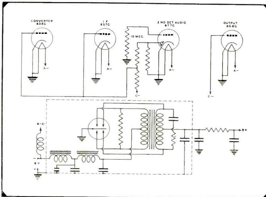
Fig. 3. Vibrator with driving coil across transformer primary.
