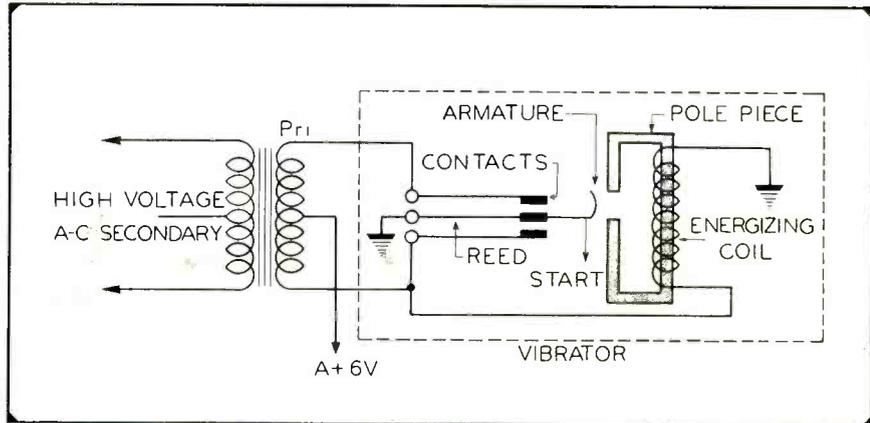
Fig. 1. Vibrator built around a U-shaped frame.
