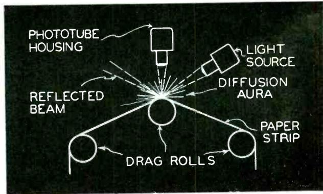
Fig. 4. The indirect or reflection method used in photo-control systems.
