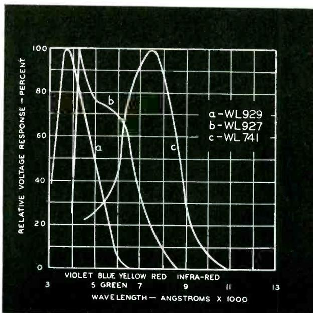
Fig. 7. A graph of the spectra to which phototubes are responsive. It will be noted that the spectral response of each tube overlaps that of the others shown. For most reliable operation, a tube having a peak in color sensitivity nearest that desired must be selected for color detection application. Incidentally, the wavelength of orange is around 6,200 angstroms.
