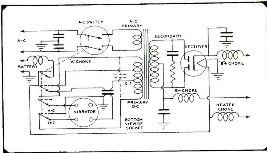
were lighter, smaller, quieter, longer lived and were free of adjustments and external unwanted vibration. Cases were made of die castings, or shells of aluminum or zinc, fitted with a base for plug-in mounting. Sound and vibration absorbers used either rubber or felt. With felt, the contacts had to be covered with a wrapping to keep the lint from the felt from interfering with the contacts.
