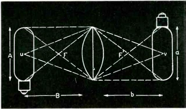
Fig. 3. How any lens can be constructed to possess two foci,  $F$  and  $F'$  at equal distances from the lens surface.  $F$  to center line is the focal length in one direction.
