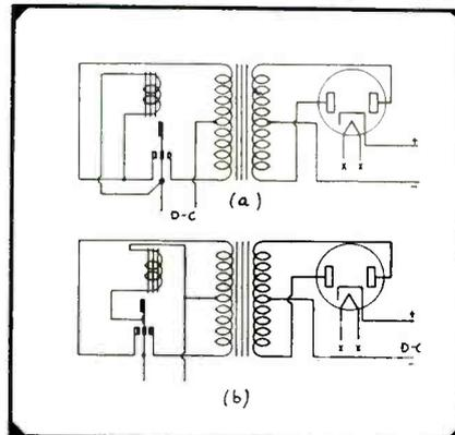
eration independent of load current for both starting and proper swing, increasing the life and efficiency many times over. Fig. 3 shows this type of vibrator with the driving coil across the transformer primary and both input and output filters. Other features will be discussed later. The shunt coil may be connected in other ways, as shown in Fig. 1 and Fig. 2 (a) and (b). Let us consider Fig. 1.
