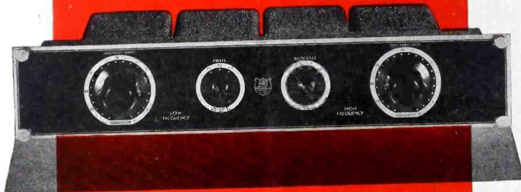
**3AX** . . . THE 'UNIVERSAL EQUALIZER' FOR BROADCAST AND RECORDING SERVICE. PROVIDES ADJUSTABLE EQUALIZATION AT 25, 50, OR 100 CYCLES FOR LOW END; AND AT 4000, 6000, 8000, OR 10,000 CYCLES AT HIGH END. CALIBRATED CONTROLS READ DIRECTLY IN DB EQUALIZATION AND FREQUENCY SETTING. THE INSERTION LOSS EFFECTED BY THE EQUALIZER IS COMPENSATED THROUGH SPECIAL COMPENSATING PADS, SO THAT IT IS CONSTANT REGARDLESS OF SETTING. RAPID CHANGE IN TONE COLOR CAN BE OBTAINED WITH NEGLIGIBLE CHANGE IN VOLUME.
