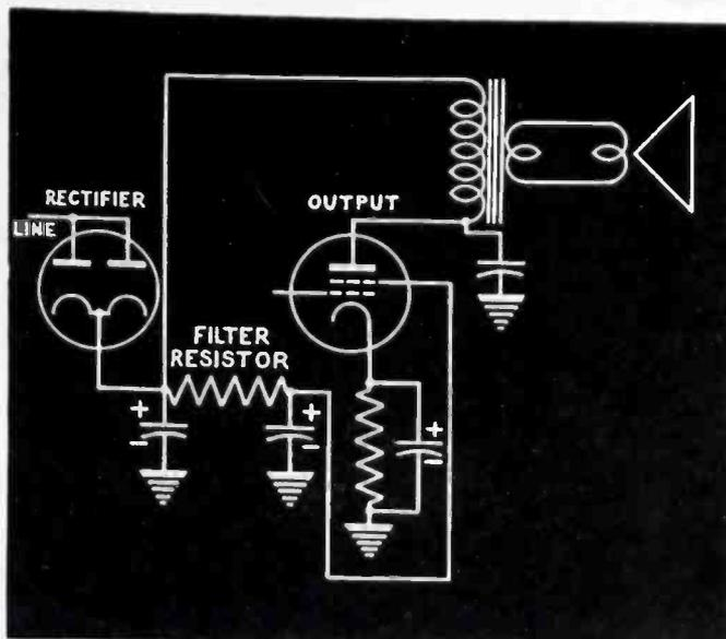
Fig. 7. A p-m speaker in a resistance-filter.
