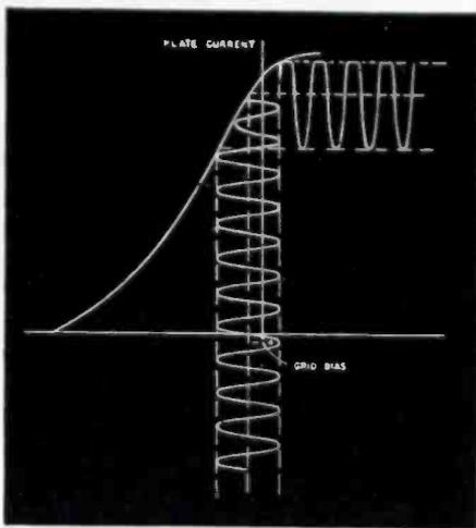
Fig. 3 shows what happens when the signal input exceeds the bias voltage. On the positive peaks of input the grid draws current and creates distortion. Note the distorted flat top on the output signal. This, in effect, is a form of signal rectification.
