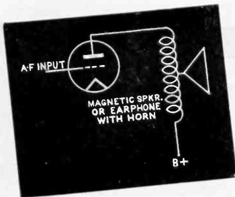
Figs. 1 (left) and 2 (right). In Fig. 1 we have a directly connected speaker in series with the plate supply. Fig. 2 shows an old type cone magnetic speaker in an impedance coupling circuit. The impedance coupling unit connected to the power tube eliminates d-c in the speaker.
