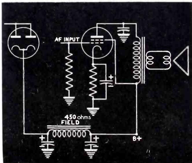
Fig. 6, a 450-ohm series-field filter in an a-c/d-c receiver.
