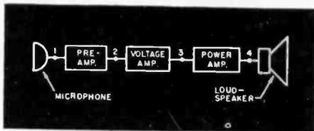
Fig. 1. Block diagram of a simple public-address amplifier.
