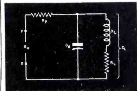
Fig. 7 (above). Here we have a circuit illustrating the effect of  $X_{Lc}$ . As this becomes larger, feedback may result due to resonance or to the fact that the plate load is higher in value than the grid-plate impedance of the tube. Fig. 8 (below). An oscilloscope setup to check output.
