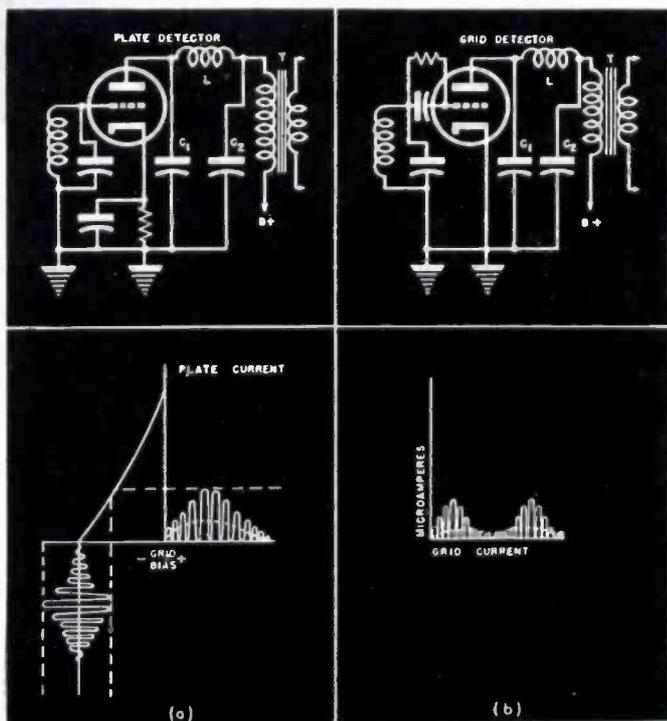
Fig. 4. How grid bias influences detection is illustrated here. In (a), since the tube is biased to cutoff, plate current will flow only on positive peaks of input signal. In (b) we have a grid detector. Here grid current serves to bias the tube. This occurs on positive peaks of the input signal and the plate current is reduced proportionately.
