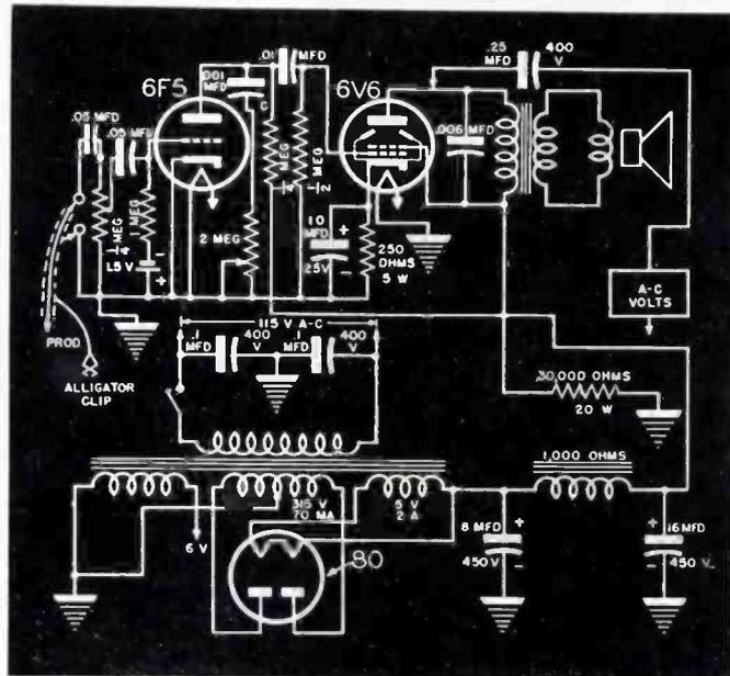
Fig. 2. An audio-frequency test amplifier. This unit can be used as an audio signal tracer. A shielded lead may be connected to the input. Audio voltages can be checked for intensity and distortion, and hum content or relative hum level.
