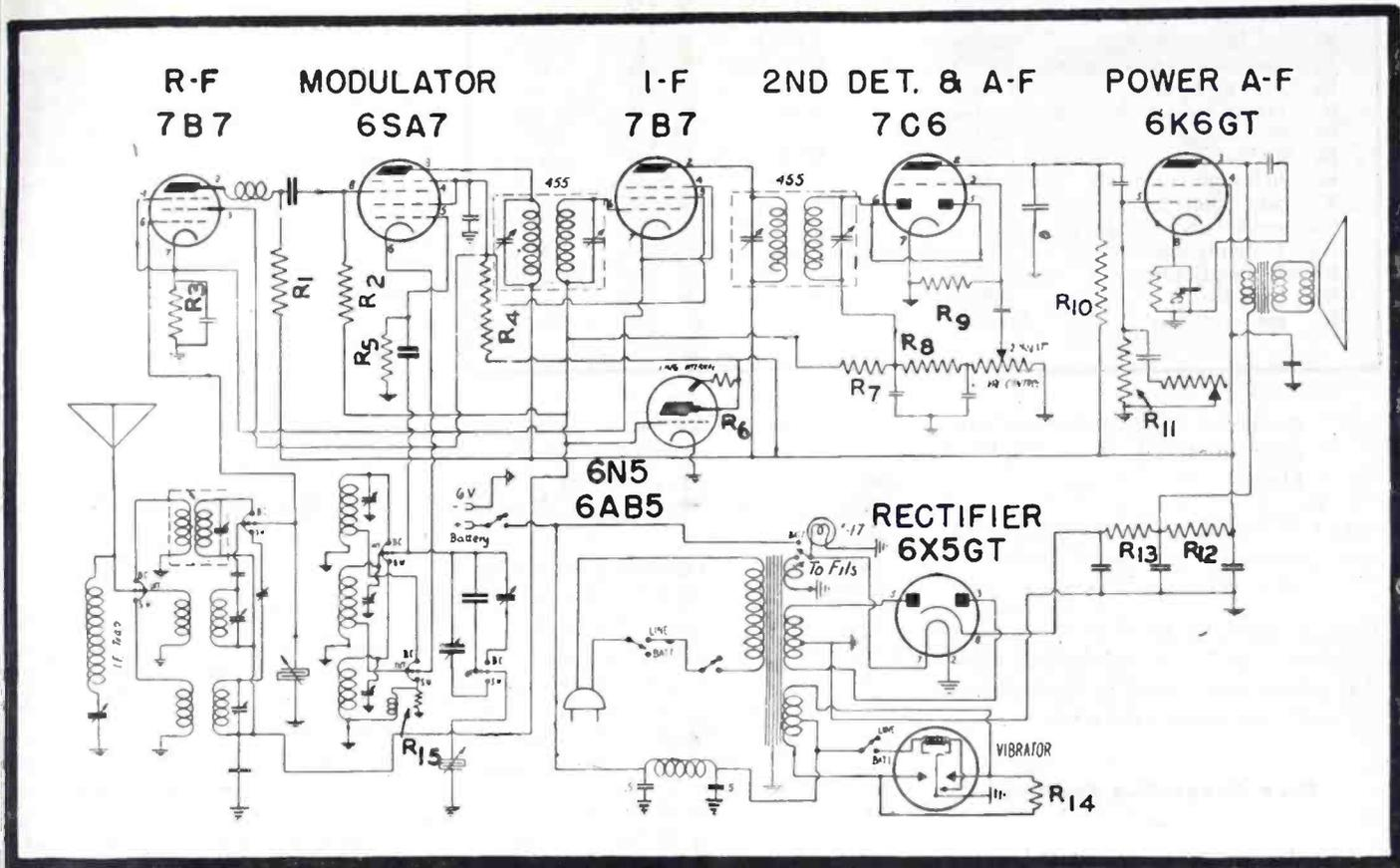
Fig. 1. A battery/a-c 7-tube super that employs fifteen fixed resistors for performing the various important functions described in this article.
