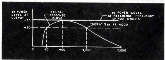
Figs. 4 (left) and 5 (above). Fig. 4, a setup used to test audio response. The vacuum-tube voltmeter connected to the input checks the input signal level, which should be kept constant as we vary the frequency. Output meter may be of the power level indicator type, which shows the output in db in reference to the standard level of .006 watts.  $Z_L$  = dummy load resistance = 1.5 x voice coil resistance. Fig. 5, variation in audio power output as a function of frequency.
