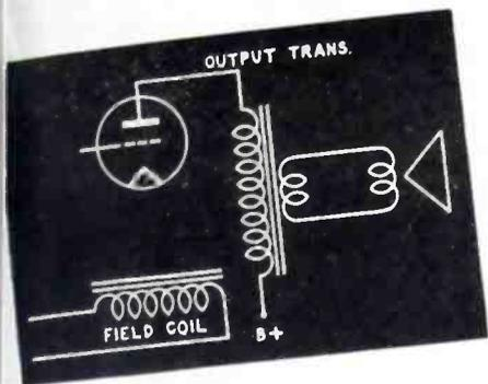
Figs. 3 (left) and 4 (right). Fig. 3, an output transformer used to provide matching between low-impedance voice coil and high impedance tube. Fig. 4 illustrates a simple push-pull circuit that helped to provide a decided improvement in quality.
