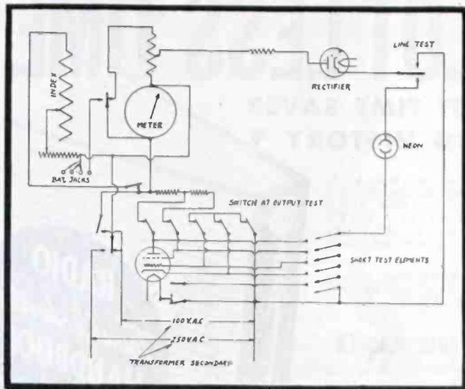
Fig. 2. The G.E. TC3 and 3P tube checker with individually operated lever switches to control voltage ranges from 1 to 117.
