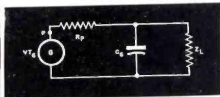
Fig. 6 (above). This circuit illustrates the reflection of the voice coil load, which is largely resistive. As the frequency rises, we have an increased shunt effect for  $C_c$  and more of the available current flows in  $C_c$  than in  $X_{Lc}$ . Thus if  $C_c$  is made lower, the h-f output will rise.
