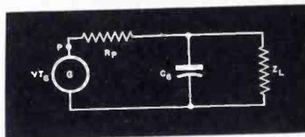
Fig. 4 (above). This circuit illustrates the reflection of the voice coil load, which is largely resistive. As the frequency rises, we have an increased shunt effect for  $C_6$  and more of the available current flows in  $C_6$  than in  $Z_L$ . Thus if  $C_6$  is decreased the h-f output will rise.
