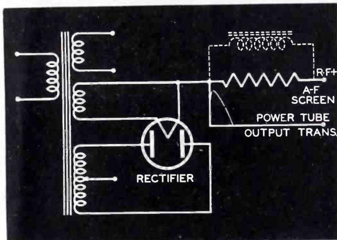
Figs. 3a (top) and 3b (right). How to increase *B* voltage by changing an electromagnetic speaker to a p-m speaker. In *a*, we have the e-m installation, while in *b*, we have the p-m substitution.
