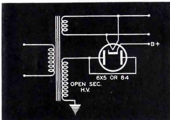
Figs. 4a (right) and 4b (below). Here we have a method of using a transformer with an open transformer or a filament transformer as a power transformer with the *B* voltage coming directly from the line.
