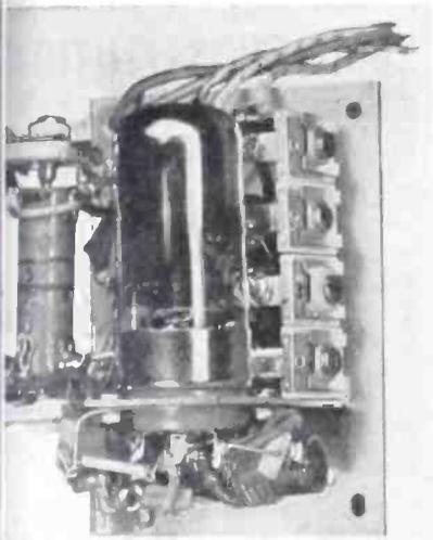
Side view of one-tube converter showing the tube, bandpass inductances, and adjustable capacitors.
