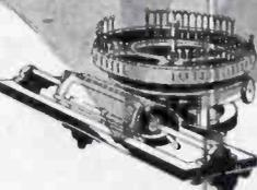
One of the first type-writers developed was that of Thurber in 1843. Then clumsy and slow, it has been brought to its present high level of efficiency and speed by careful application of design.
