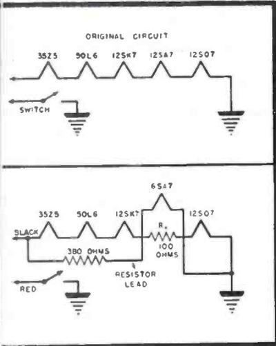
Figs. 1 and 2. Original and rewired circuits.
