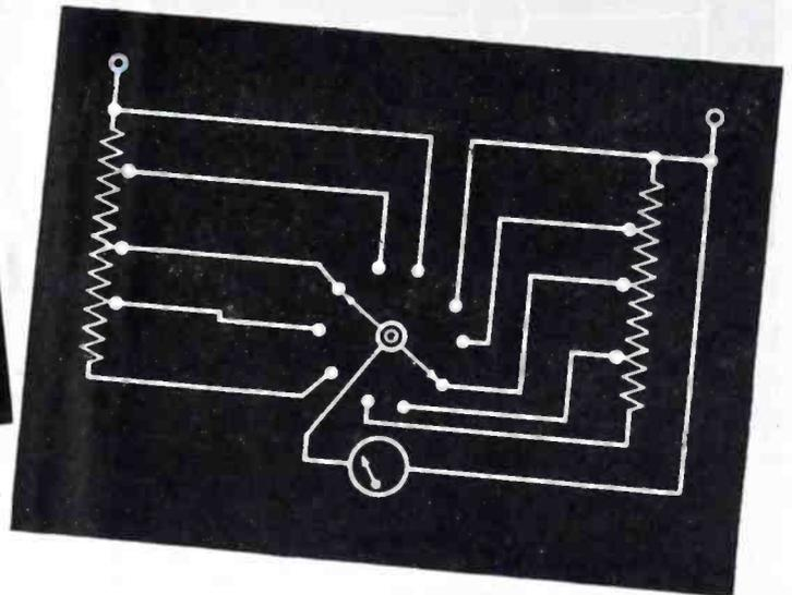
Figs. 1 (above) and 2 (right, above). Fig. 1. Inserting a shunt so that combined resistance of meter and shunt are equal to that of meter when used alone. Fig. 2 shows a method used to change series and shunt resistor ranges with a double-ended rotary switch.
