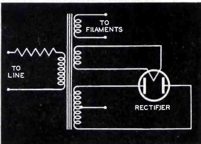
Figs. 1a (above) and 1b (left). In a we have a standard 6.3-volt transformer installation. How to use a 2.5 and 5-volt transformer to secure 6.3 volts is shown in b. The two windings are connected in series aiding to provide the required voltage.
