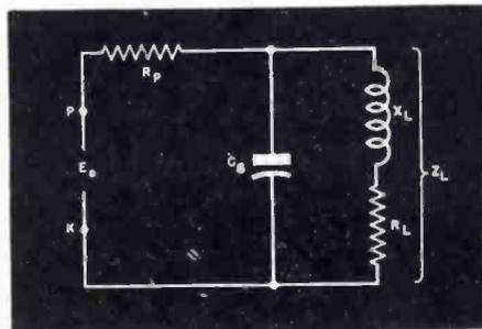
Fig. 5 (above). Here we have a circuit illustrating the effect of  $X_L$ . As this becomes larger, feedback may result due to resonance or to the fact that the plate load is higher in value than the grid-plate impedance of the tube. Fig. 6 (below). An oscilloscope setup to check output.
