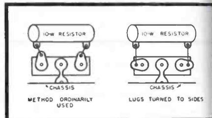
Fig. 5. Old and new methods of mounting resistors.
