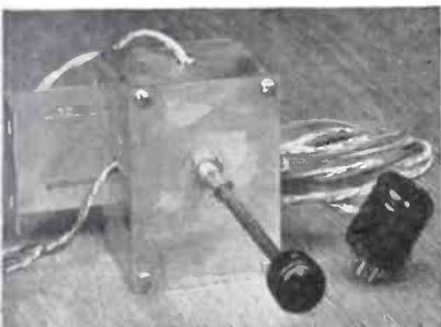
The tube converter, complete with mounting bracket, power take-off plug, etc.
