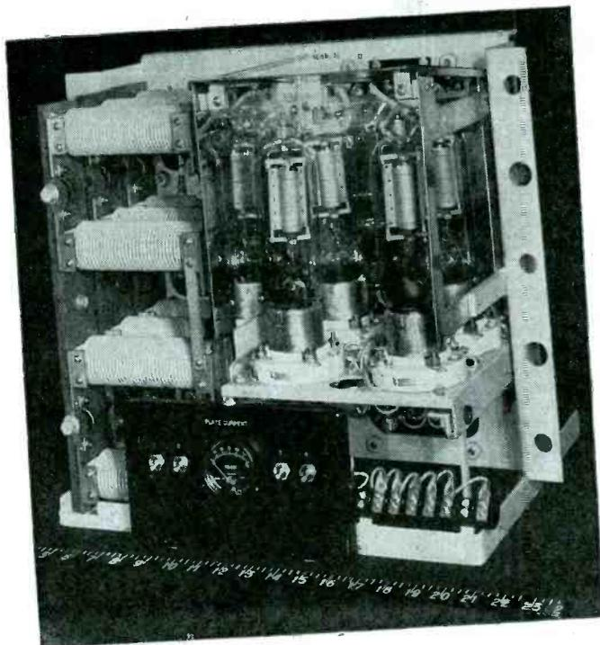
Figs. 1 (left) and 2 (below) Fig. 1 illustrates a 500-watt power amplifier used aboard warships. This amplifier is driven by the 40-watt preliminary amplifier shown in Fig. 2. Note the small size of the power amplifier.
