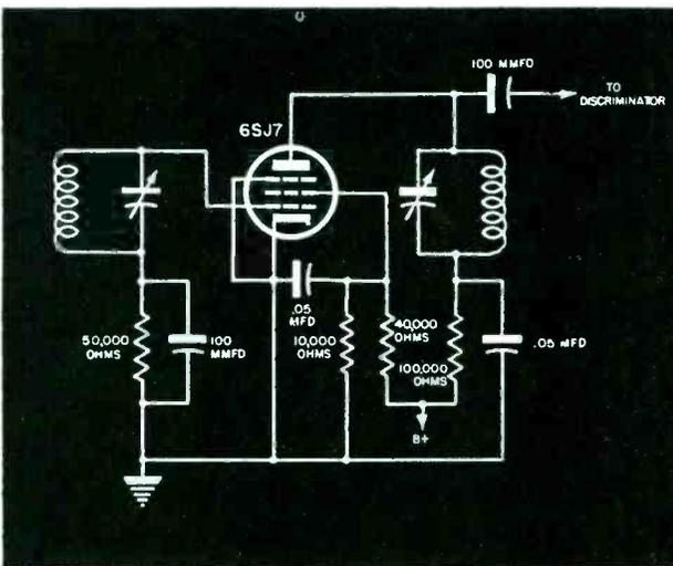
Fig. 5. The Emerson FM 460 limiter. This limiter is used in the a-c/d-c model, which accounts for the low value plate and screen voltage dropping resistors.
