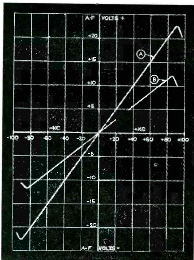
Fig. 1. Typical characteristic curves for an f-m discriminator. The curves represent the differential audio voltage output in terms of the frequency swing; curve A represents the characteristic for a given value of input; B shows the curve for a smaller value input. Note that the output voltage is a direct function of the input voltage.
