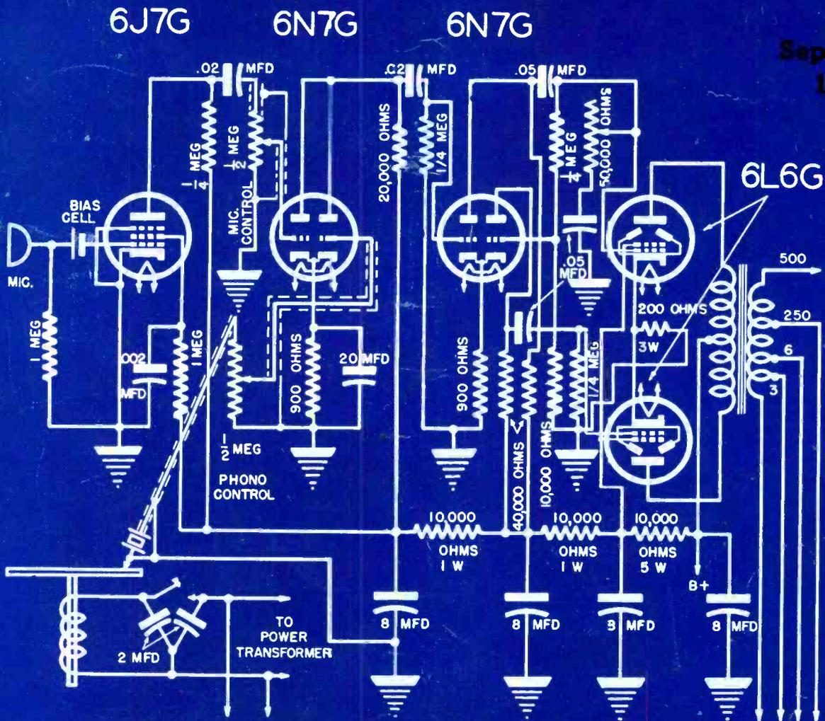
Four-stage, 6-tube, 20-watt mobile p.c. unit that can be used on 6-volt d-c or 115-volt a-c. (See page 51.)
