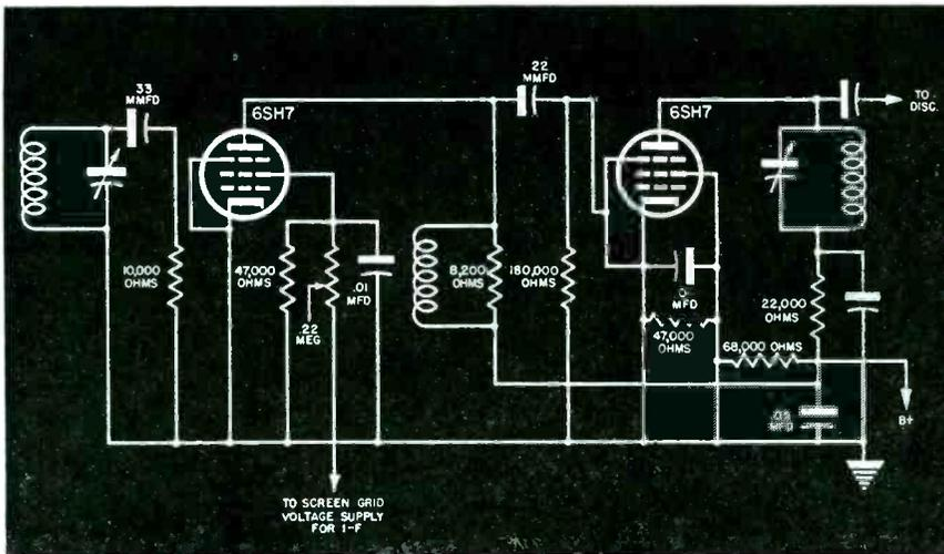
Fig. 6. Cascade limiter used in the G.E. model 40. Resistance coupling is used interstage to reduce the hazard of feedback. Both limiters have almost the same time constant, since limiter 1 has already limited the range of input to limiter 2.
