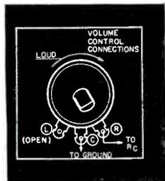
Fig. 3. A bias type of volume-control circuit requiring a resistor having right-hand taper;  $R_c$  is a fixed minimum-bias resistor.
