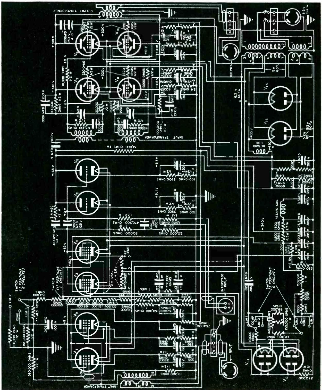
Fig. 3. Preliminary amplifiers schematic.  $V_1$  and  $V_2$  are 6J7s;  $V_3$  and  $V_4$ , 6L7s;  $V_5$  and  $V_6$ , 6C5s;  $V_7$ ,  $V_8$ ,  $V_9$  and  $V_{10}$  are 6L6s;  $V_{11}$  and  $V_{12}$ , 6H6s; and  $V_{13}$  and  $V_{14}$  are 5T4s. This amplifier of 40-watt capacity was used either as a preamplifier to the 500-watt unit, or alone. In turret or anti-aircraft systems, the 40-watt unit was sufficient.
