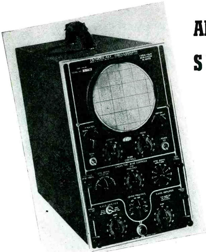
Fig. 1. Oscilloscope with 5" screen
