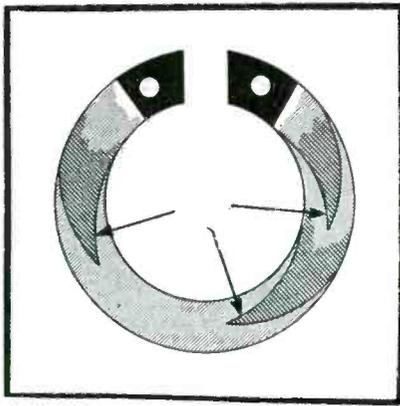
Fig. 5. The resistance element of a composition-element control; one method of obtaining smooth taper.
