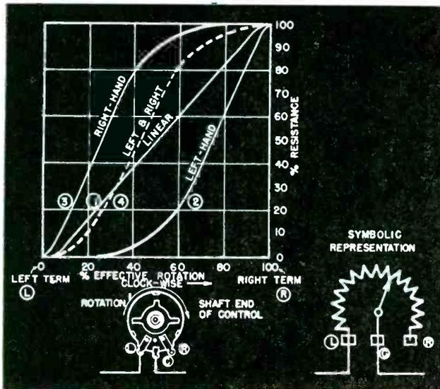
Figs. 1 (left) and 2 (right). In Fig. 1, we have resistance characteristic curves illustrating linear, left-hand, right-hand, and combination left-and-right-hand taper. Fig. 2 shows two variations of an audio shunt type of volume control. Both require a control having left-hand taper, but the control terminals are connected differently in each case.
