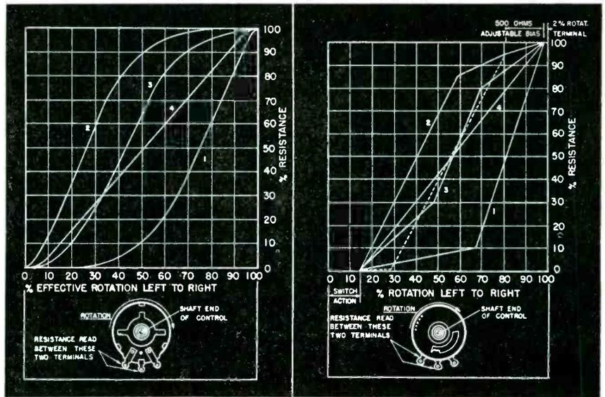
Fig. 6. Typical tapers obtainable in composition-element and wire-wound controls for meeting all replacement requirements. Left-hand illustration covers composition-element controls; right-hand illustration for wire-wound controls.
