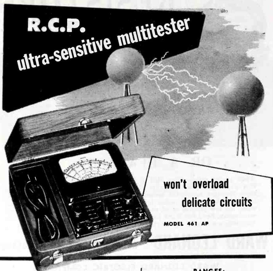
DC sensitivity of 20,000 ohms per volt in the R.C.P. Multitester results in negligible loading of most circuits. A wide range of measurements for field, shop and laboratory testing is provided in one handy and responsive instrument. The 4½" wide scale meter has a movement of 50 microamperes and gives readings as low as 1 microampere on the 100 microampere scale. Meter movement is accurate to 2%. Shunts and matched pair voltage multipliers accurate to 1%.
