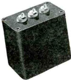
UTC Interstage Filters (10,000 ohms impedance) are available in low pass (LPI), high pass (HPI), and band pass (BPI) types for all frequencies from 200 to 10,000 cycles. Designed to effect 6 DB loss at cutoff frequency . . . 35 DB at .75 and 1.5 times cutoff frequency . . . 40 DB at .5 and twice cutoff frequency. Dual alloy magnetic shielding reduces pickup to 150 Mv. per gauss.
