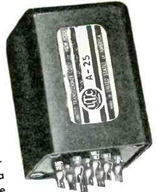
For compact, high fidelity equipment, UTC Ultra Compact units are unequalled. Light in weight, yet providing frequency response  $\pm 2$  DB from 30 to 20,000 cycles. All units except those carrying DC in primary employ true hum balancing coil structure which, combined with high conductivity outer case, insures good inductive shielding. Units available for all audio applications up to + 10 DB in operating level.
