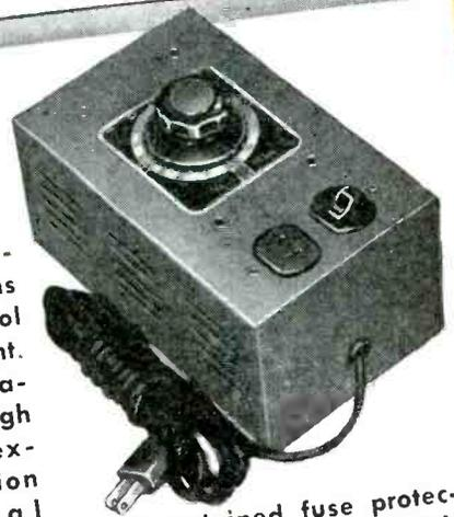
Varitran units provide an ideal means of voltage control for AC equipment. Performance features include high efficiency . . . excellent regulation . . . universal mounting features . . . self-contained fuse protection. Available in 115 volt and 230 volt models with from 1 to 11 Amp. output rating. These units afford stepless adjustment of voltage from 0 to 113% of line voltage.
