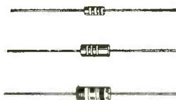
1/2 watt, 1 watt, 2 watts
