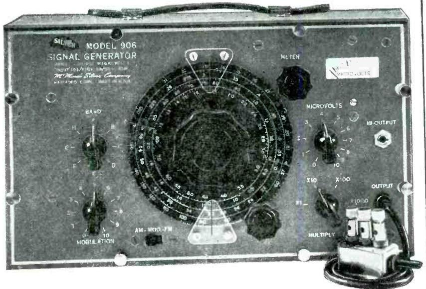
The one word "greatest" best describes new MODEL 906 Signal Generator . . . greatest frequency range of 90 kc. through 170 mc. AM; 90 kc. through 210 mc. FM . . . greatest calibration accuracy of 1% . . . greatest output range — metered and continuously variable from less than 1 microvolt to over 1 volt . . . greatest freedom from strays . . . greatest "buy" in history at only \$89.90 net.
