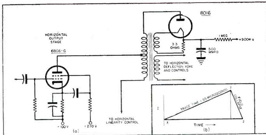
Fig. 5a and b. In a appears circuit of the kick-back power supply used in the RCA 630TS television receiver. In b appears a plot of the applied wave; trace time between x and y causes slowly increasing current through portion of scanning transformer.
