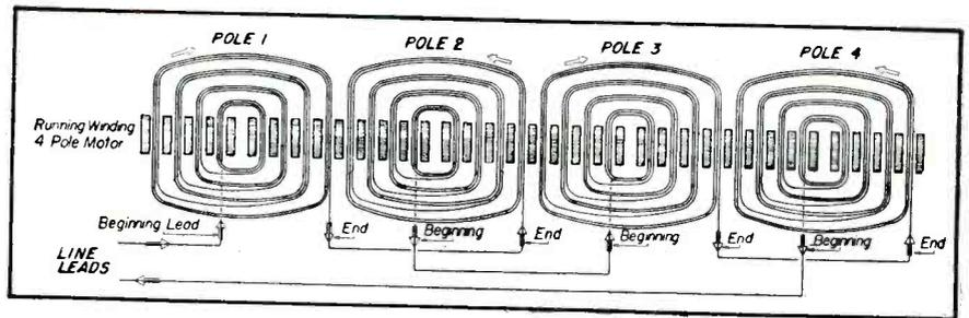
Fig. 17. Four poles of the running winding connected for correct polarity.
