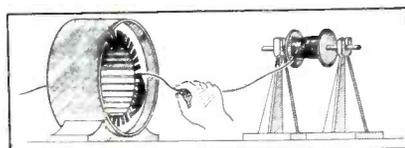
is accomplished by connecting them in such manner that the current will flow through the first pole in a clockwise direction and through the second pole in a counterclockwise direction; Fig. 17. This shows a four-pole running winding of a thirty-six slot motor.
