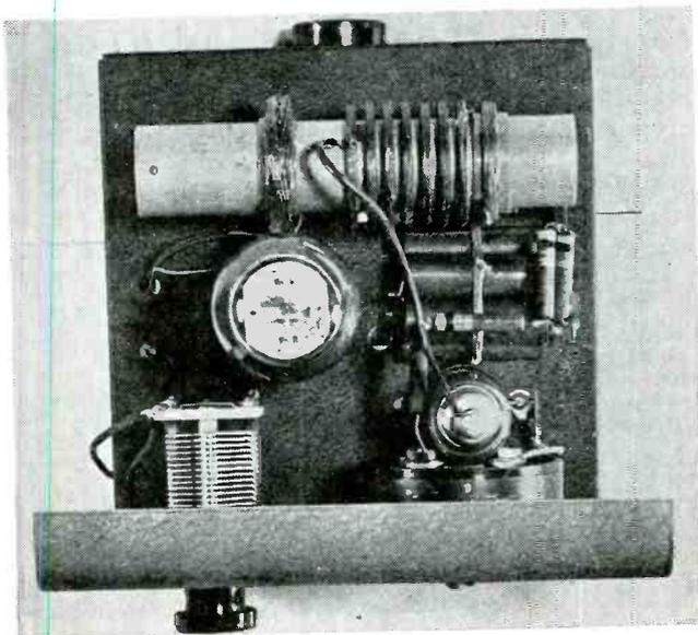
View of the fly-back power supply. The deflection yoke for magnetic deflection, used with the picture tube, appears at upper left. At extreme right is the high voltage rectifier, 8016, while at the lower right appears the horizontal output transformer.
