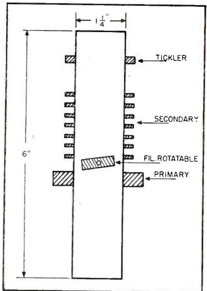
Fig. 2. Cutaway view of r-f coil. Top coil is grid-tickler winding; center, multiple  $\pi$  sections of high voltage secondary.
