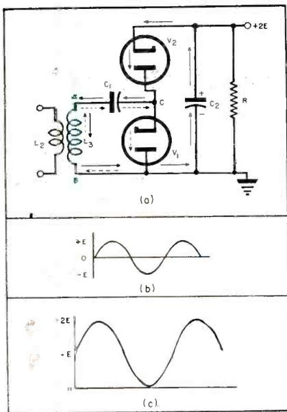
Fig. 3a, b and c. In a appears a circuit of a cascade voltage doubler. Plots of b and c represent the doubler action, shifting of axis of input sine wave; this is similar to d-c restorer operation in tv receivers.
