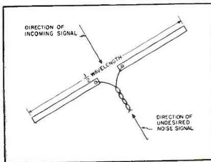
Fig. 5. Signal response of a half-wave dipole.
