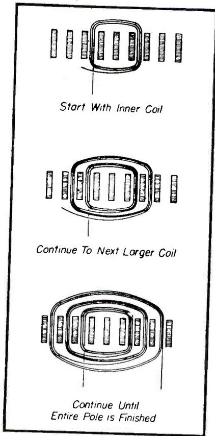
Fig. 15. Procedure for winding a stator pole by hand.
