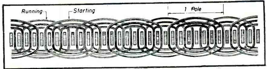
Fig. 10. Diagram of the poles of a thirty-two slot four pole motor. Note how the starting winding overlaps the running winding.
