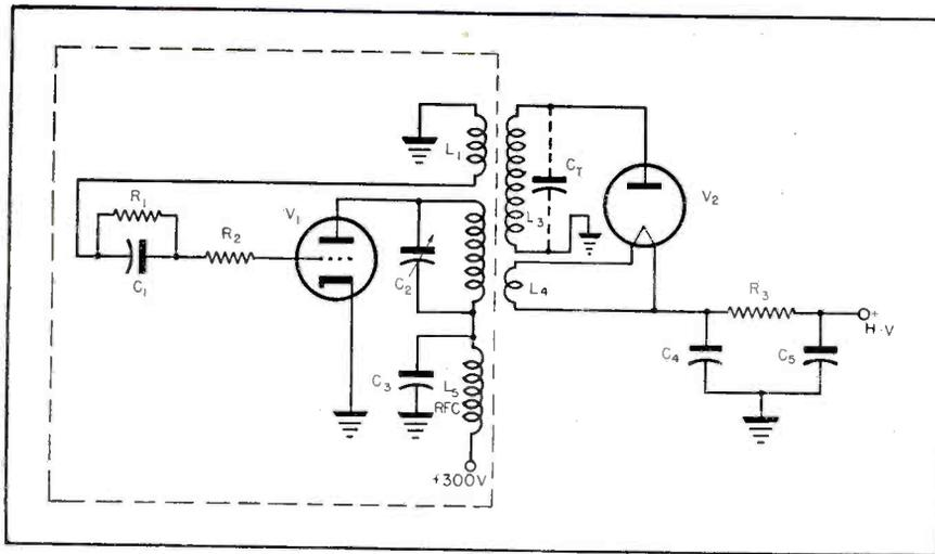
Fig. 1. Circuit of a basic r-f tv power supply.
