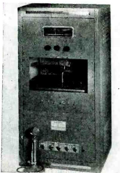
A 35-watt amplifier for indoor use, which features a 2-band tuner and record changer player. System is supplied with fourteen 12" p-m speakers. (Courtesy Radio Wire Television Inc.)
