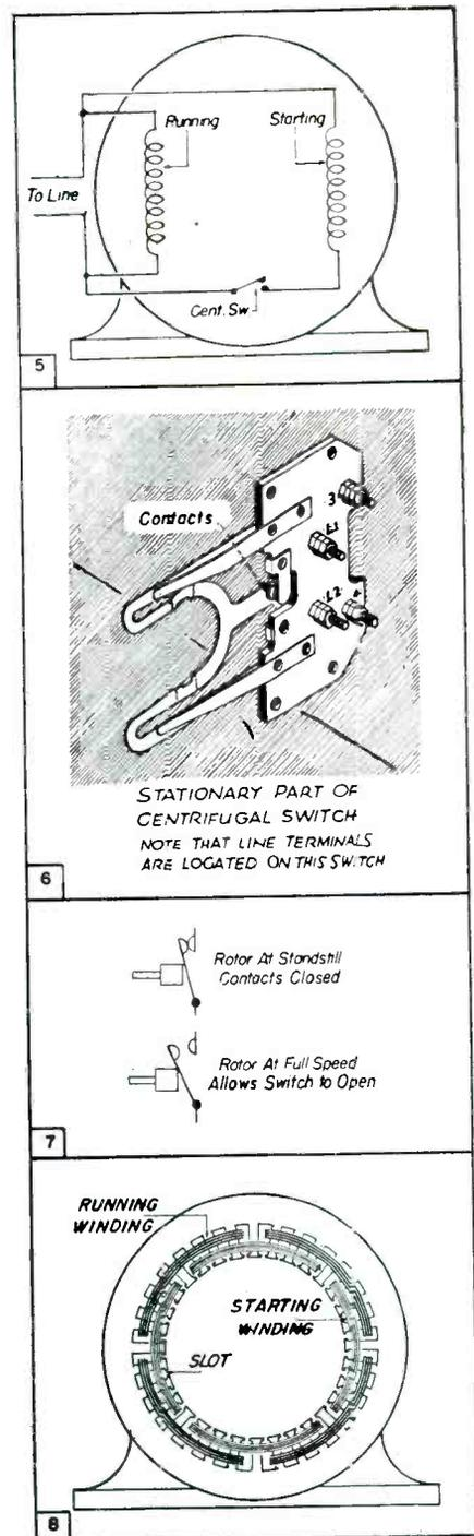
Figs. 5, 6, 7 and 8. Fig. 5 shows a wiring diagram of a split-phase motor. Note windings and the centrifugal switch. In Fig. 6 we have the stationary part of a centrifugal switch. Fig. 7 shows the steps involved in the operation of a centrifugal switch. The two windings of a split-phase motor appear in Fig. 8. Note the four sections or poles in each winding.
