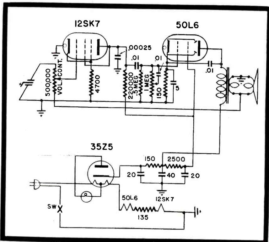
Fig. 2. Electromatic APH 301A amplifier using one 12SK7 as a triode with plate and screen tied together.
