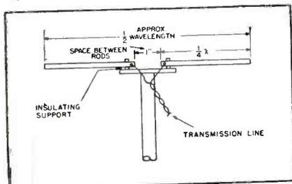
antenna provides a radiation resistance or about 72 ohms at resonance. A dipole resonates when its length is approximately equal to one-half wavelength of the frequency that it is to be used on.
