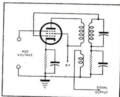
Fig. 5, left. Representative circuit of a suppressor-grid modulated oscillator. Any voltage impressed between the suppressor grid and ground will vary the oscillator signal by establishing a virtual cathode between suppressor and screen grid. The amplitude of the oscillation will then become a function of the amplitude and polarity of the suppressor voltage.
