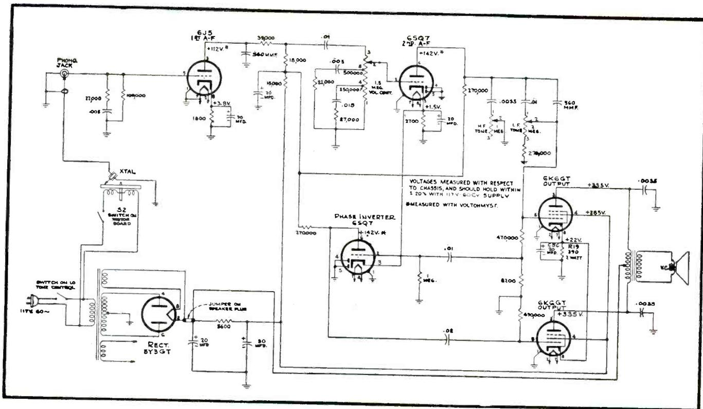
Fig. 4, above. RCA Victor 66E amplifier designed for a low-voltage pickup.
