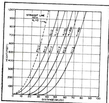
According to the formula: Maximum distance for straight-line path =  $1.23(\sqrt{H_t} + \sqrt{H_r})$ , where the antenna heights are in feet and the distance is in miles.
