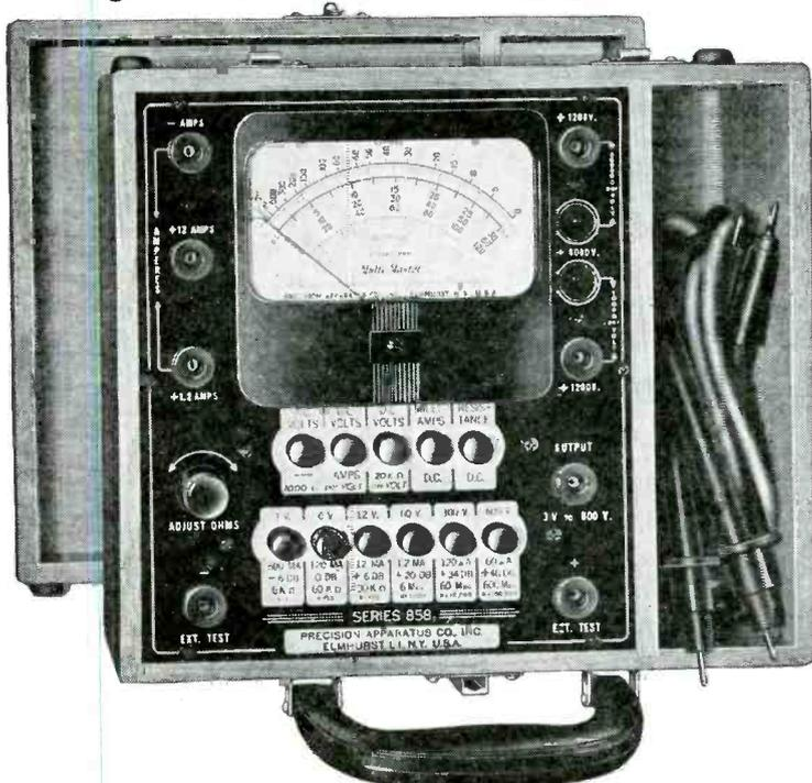
Series 858 MULTI-MASTER features "Precision" Automatic Push Button range and function selection, affording the ultimate in operational efficiency and simplicity.
