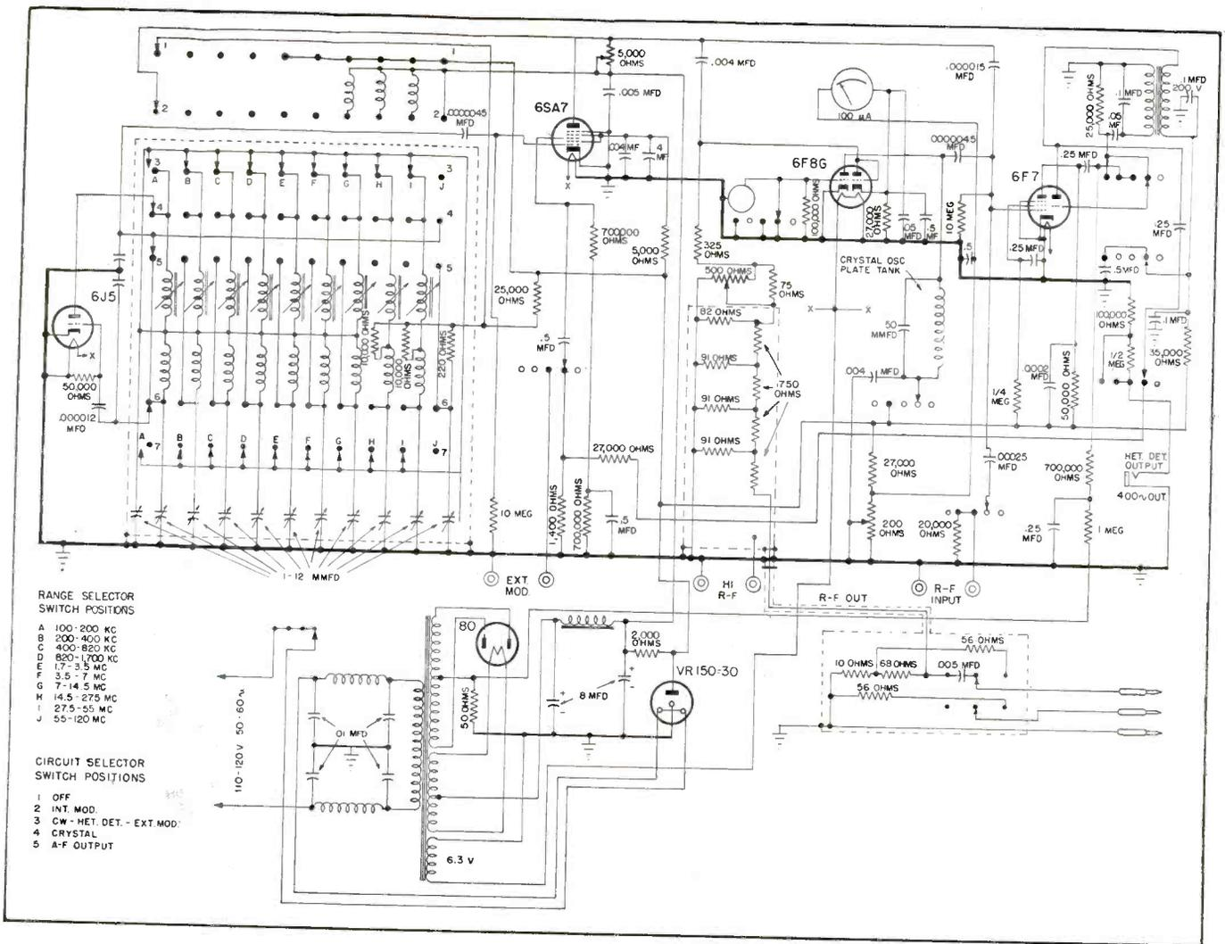
Fig. 1. Circuit of the Triplet 1632 signal generator.
