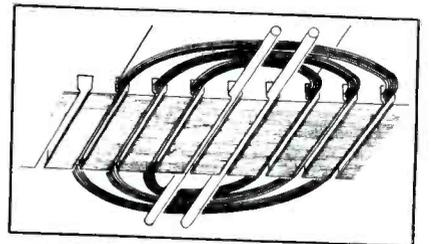
Fig. 16. How wooden dowels may be placed in empty slots to hold coils in position while winding.
