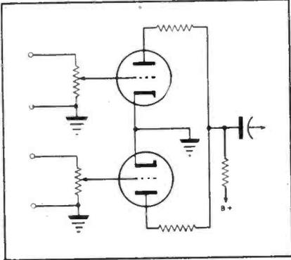
Fig. 3. An input system with pentode high-impedance circuits where isolating resistors are unnecessary.
