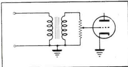
Fig. 5. Connection of two phono inputs to one tube.
