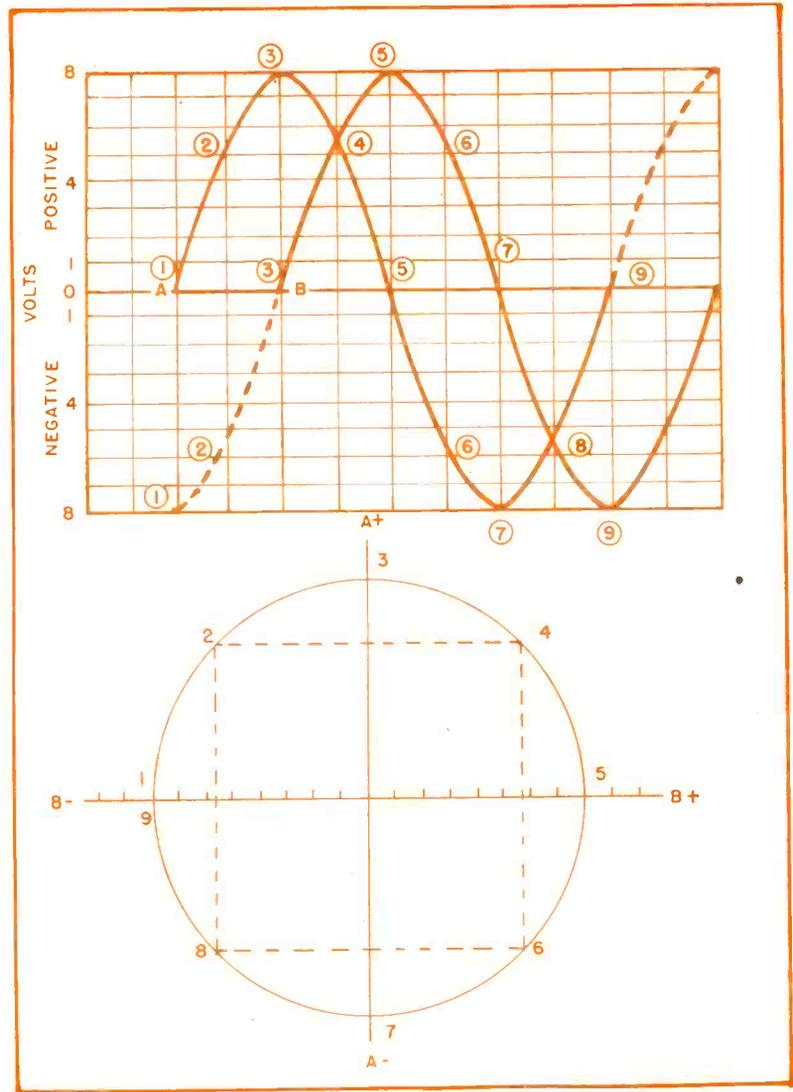
Figs. 4 (above) and 5 (below). The tracing of a Lissajou figure is here shown in detail. Two similar voltages have been applied to both the horizontal and vertical plates. However, one voltage is starting  $90^\circ$ , or  $\frac{1}{4}$  of a cycle later than the other. In Fig. 5, A — and + represent the vertical voltages, and B — and + the horizontal voltages. The position of the dot will then be a function of these two voltages. The resultant picture in this case is a perfect circle.
