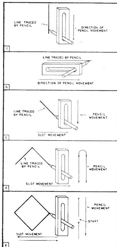
are so balanced as to move in pairs. One pair moves vertically, the other pair horizontally, as shown in Fig. 1c, the movement being a function of the voltages applied to these plates.
