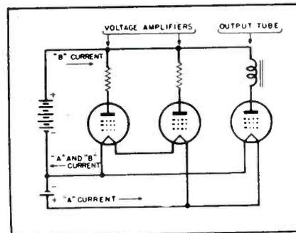
Fig. 1. A typical 3-tube hearing-aid circuit using two voltage amplifiers and an output tube. The a supply of 1½ volts feeds two tubes with their .625-volt filaments in series. The filament of the output tube is rated at 1.25 volts. (Courtesy National Carbon Co.)
