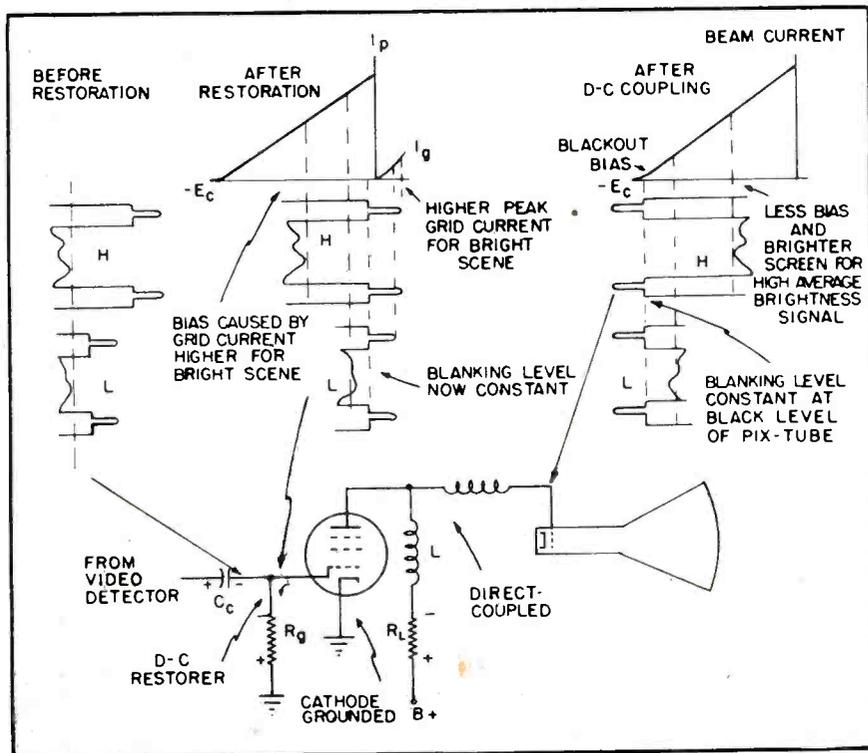
almost the entire line is at a high negative voltage level (near the blanking level) which maintains a high negative voltage on the grid, producing a correspondingly dark scene. Although the average brightness is low, there can be instantaneous bright spots along the line such as point *C*, which represents a very brilliant spot.
