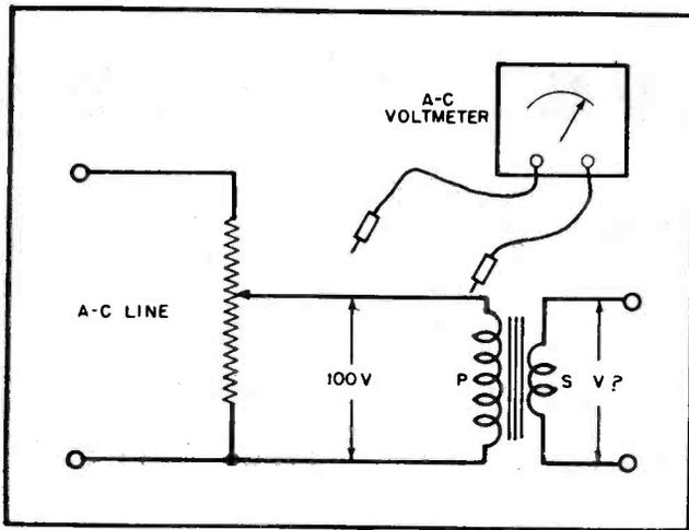
Fig. 1. Dropping voltage to 100 with a potentiometer and measuring circuit to determine winding ratios with an a-c voltmeter.
