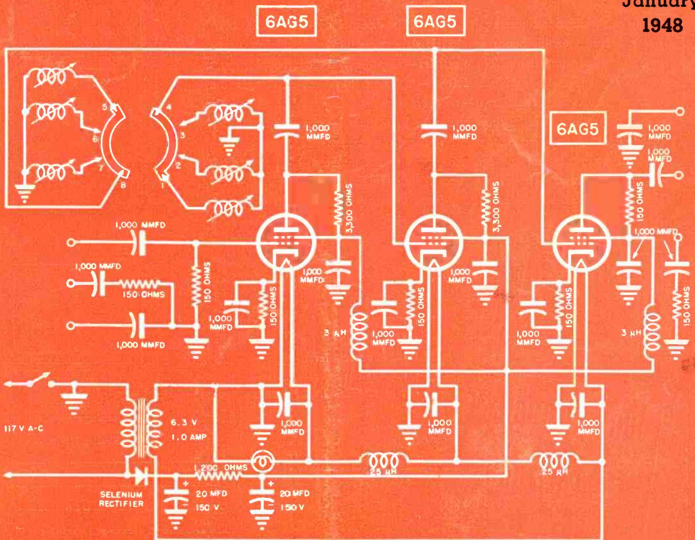
Three-tube high-gain television-signal booster, with provision for 75-ohm or 300-ohm inputs and outputs.
