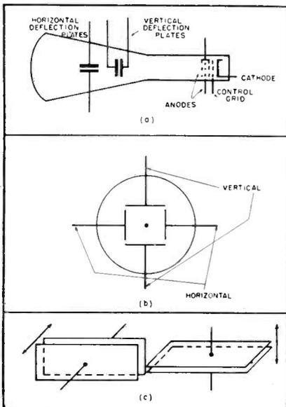
operated at very high potentials and differ from ordinary tube plates in that, instead of attracting the electrons emitted by the cathode, they serve to accelerate the electron flow. In other words, they *push 'em along*. The electron stream then passes between the two sets of deflection plates, which
