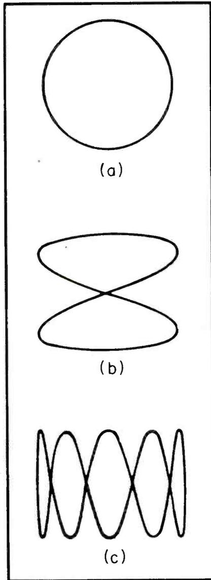
Fig. 7. Three types of Lissajou figures. In *a* we have a frequency relationship between the horizontal and vertical deflection voltages of one to one. At *b*, the ratio is two to one, and at *c*, one to five.
