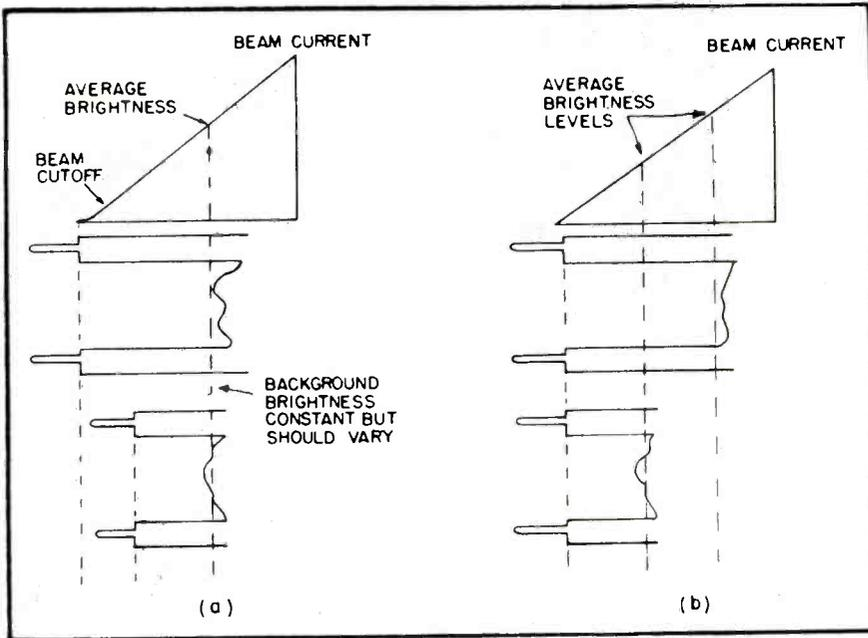
Fig. 3. Signal distribution on grid of picture tube with and without proper restoration. Plot at left shows how the blanking level varies with the signal content. Blanking does not always coincide with the blackout level at all times. The plot at right shows the proper restoration. Here the blanking level is constant and the average bias varies with average brightness of the scene.
