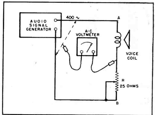
Fig. 2. Circuit used to measure v-c impedance with an a-f generator set at 400 cps and an a-c voltmeter.
