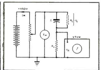
Fig. 2. Setup using a vacuum-tube voltmeter for the checking of leakage resistance of capacitors. C is a capacitor under test;  $R_c$ , leakage resistance of the capacitor in megohms;  $R_v$ , total resistance between the vtvm terminals in megohms before the capacitor is placed into the circuit;  $V_c$ , voltage drop across  $R_c$ ;  $V_R$ , voltage drop across the vtvm and  $E_w$ , working voltage for the capacitor being tested.
