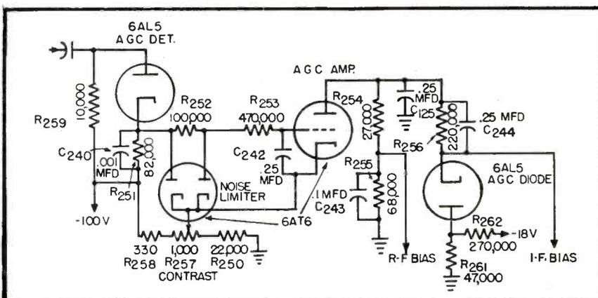
Fig. 1. The agc system used in the RCA 641 tv receiver.
