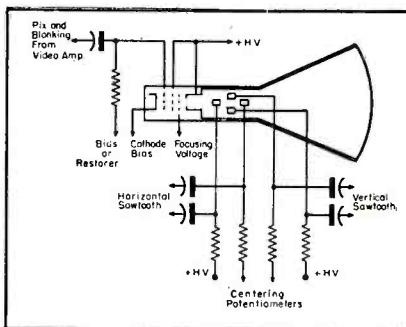
Fig. 4. A picture tube circuit for electrostatic deflection and focusing.
