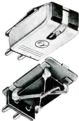
compliance at the expense of lowering the electrical output in proportion to the additional compliance it offers. Needles, too, have been designed with extra flexibility with improved performance, particularly on low frequencies.
