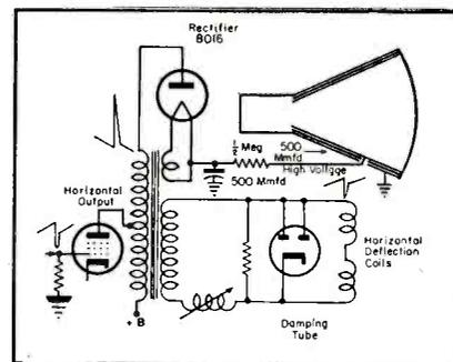
Fig. 5. A flyback high-voltage supply.
