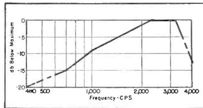
Fig. 1. Overall acoustic response, from microphone input to horn output, of typical electric megaphones.
