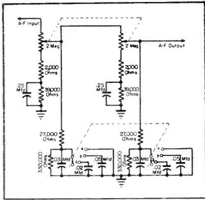
Fig. 3. A dual volume-control circuit used to obtain the desired bass-boost characteristics over a wide range of output levels. Circuit is similar to that used in the G.E. model 41.
