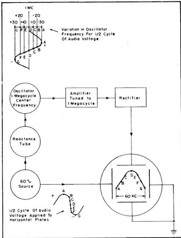
Fig. 3. Simplified visual alignment circuit.
