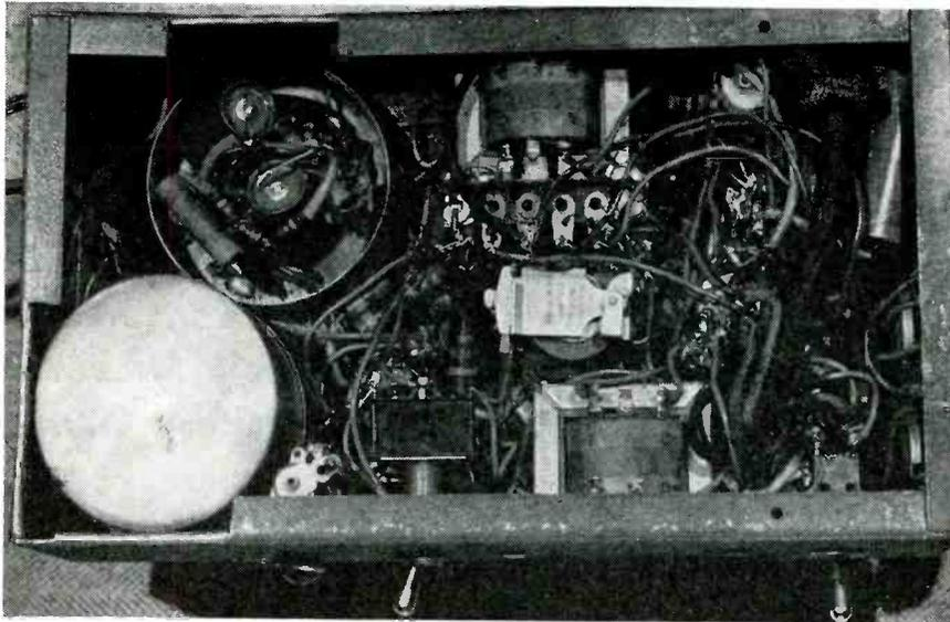
Bottom view of chassis with cover of high gain stage of one channel removed. Switch at lower left is the listening switch. Relay in center is *E* relay.
