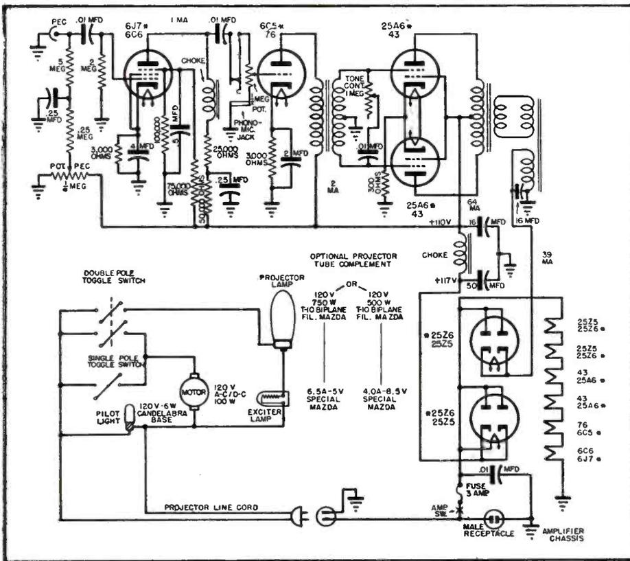
Fig. 1. Circuit of the projection and amplifier system of the Victor model 25 universal. Early models used the 6C6, 76, 43 and 25Z5; later models, 6J7, 6C5, 25A6 and 25Z6 tubes. Readings in ma were made at 115 v. a-c.
