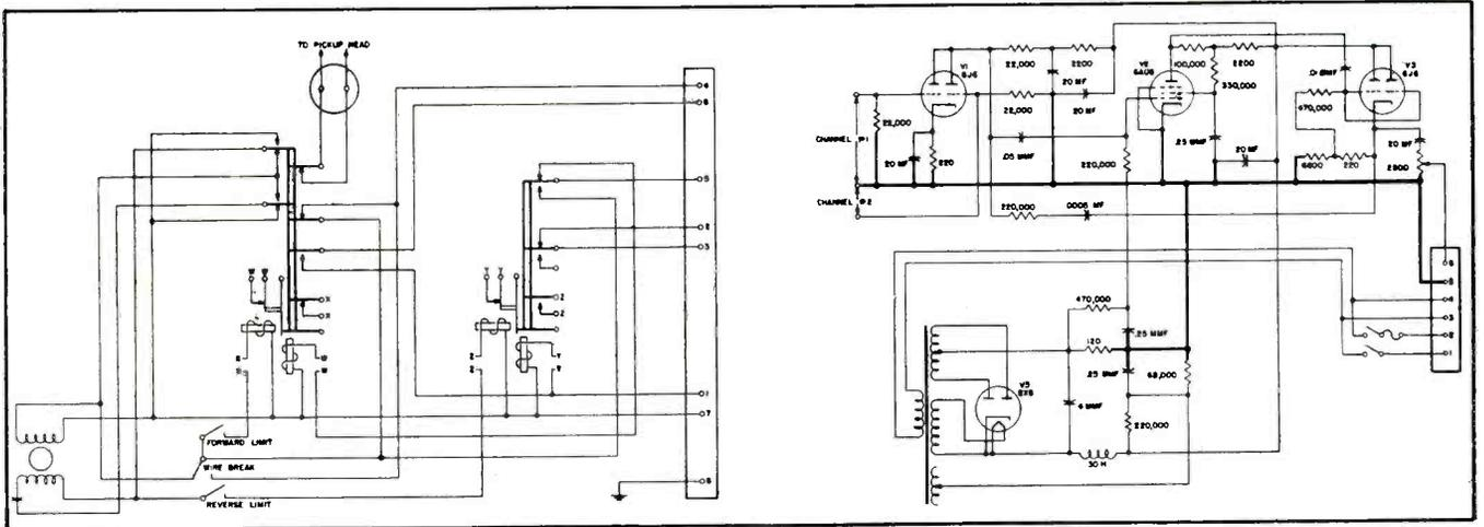
Fig. 2. Wire reproducer and preamp schematics.
