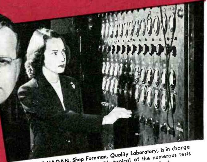
ROBERT HAGAN, Shop Foreman, Quality Laboratory, is in charge of the strict Life Test, above. It's typical of the numerous tests that Ken-Rad tubes must pass before leaving the plant.
