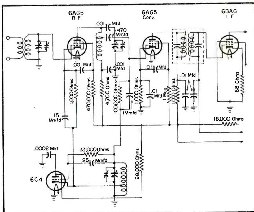
Fig. 5. Meissner 8C FM tuner circuit, which features capacity tuning.
