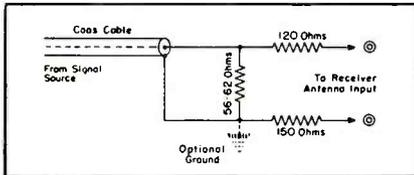
Fig. 4. Resistance matching pad, coax-to-balanced.
