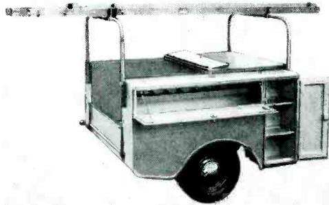
The All Purpose Workshop Trailer of All Steel Construction Can Be Readily Towed by a Car or Truck
