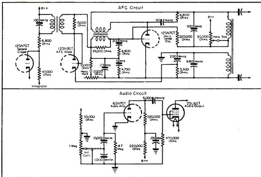
Fig. 2. Circuits developed to provide *afc* for the Motorola VT71 TV receiver. The audio circuit changes required are also shown in this figure.
