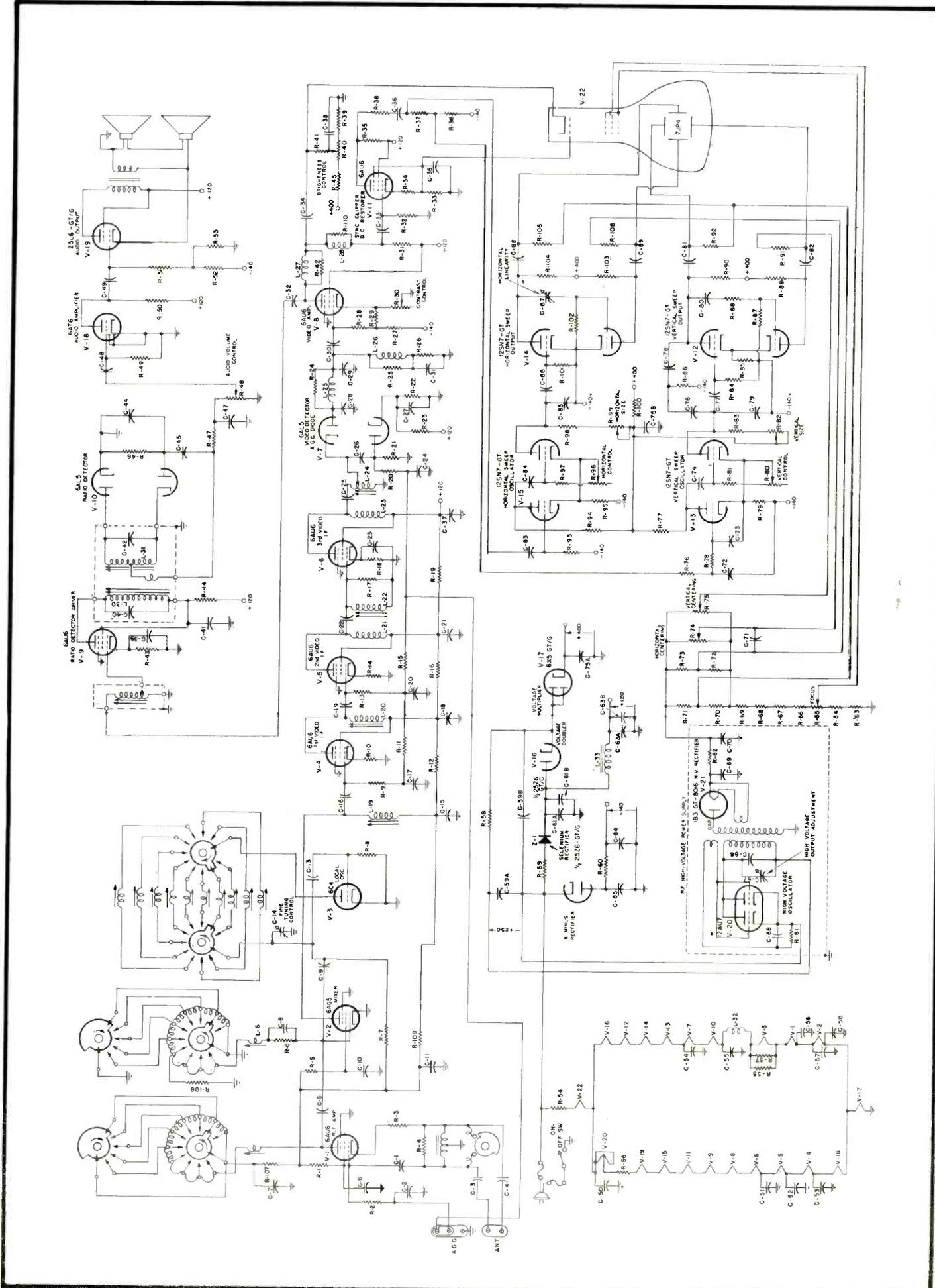
Fig. 1. Complete circuit diagram of the NC-TV-7/NC-TV-7M. (See parts lists on page 18.)
