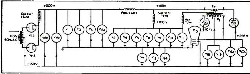
Fig. 3. Power supply distribution and division of potentials in the Bendix receiver; arrows indicate direction of electron flow rather than the conventional positive current flow.
