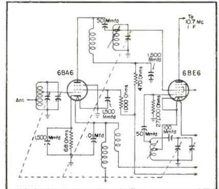
Fig. 2. Circuit of the capacity-tuned unit shown in Fig. 1.
