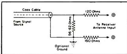
Fig. 4. Resistance matching pad, coax-to-balanced.
