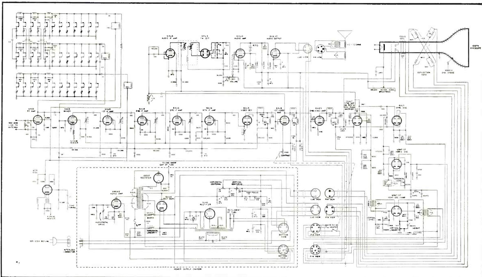
Fig. 2. Circuit of the Hallicrafters T-61 and T-67 TV chassis.
