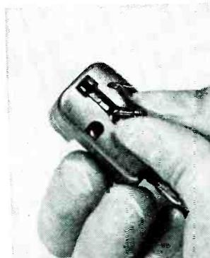
3 Insert new stylus into cartridge with fingers.
