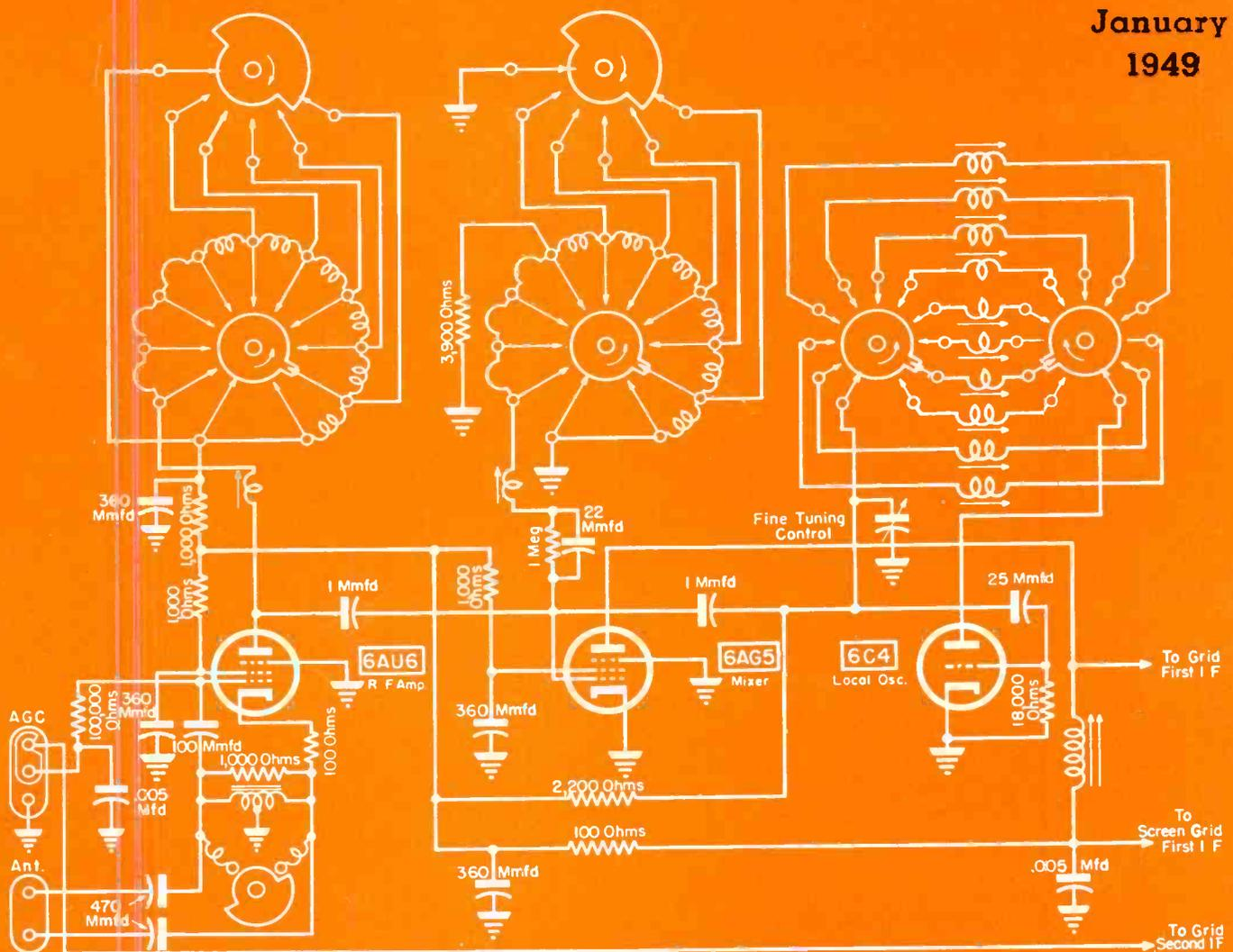
Front end of a 7" direct-view twin-speaker TV receiver featuring the intercarrier-sound system.
