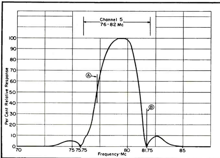
Fig. 5. Overall response at video detector. At (A) appears the picture rf carrier point, 77.25 mc, and at (B) appears the sound rf carrier point, 81.75 mc.
