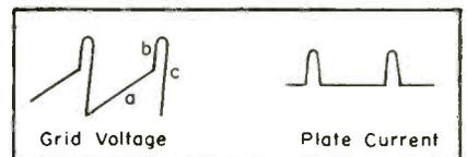
Fig. 7. Sawtooth of potential at grid superimposed upon which is a positive pulse: a, high negative grid potential is leaking off grid resistor; b, tube begins to conduct and grid is driven positive; c, grid is driven sharply, highly negative.
