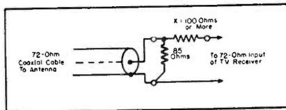
Fig. 2. Simple pad for adjustment of signal level between 72-ohm coaxial line and a receiver with a 72-ohm unbalanced input.
