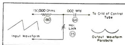
Fig. 2. The parabola circuit.
