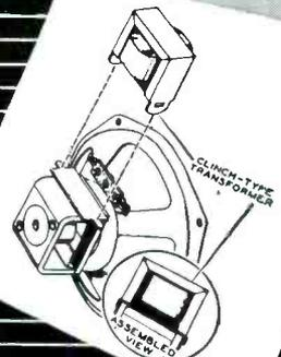
Another RCA first, to speed your service work . . . the universal transformer mounting bracket. Saves time in mounting either clinch-type or strap-type output transformers. Included with all 4", 4" x 6", and 5" RCA PM speakers. Larger speakers include mounting holes on frame according to RMA standards.
