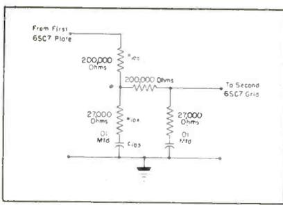
Fig. 1. Alternate If compensation circuit.
