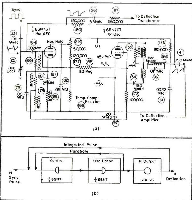
Fig. 1. Basic circuit of the Magnavox horizontal afc system.
