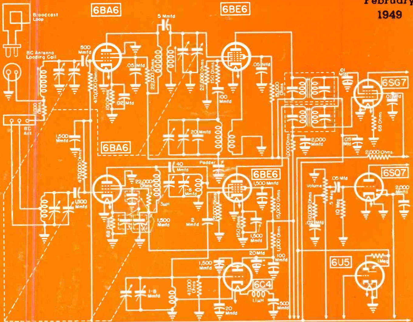
The *r<sub>f</sub>* converter, mixer, oscillator, *1<sub>f</sub>*, first of and tuning indicator stages of a 10-tube AM-FM tuner.
