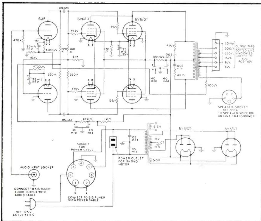
Fig. 1. Circuit of the audio amplifier designed for the tuner.
