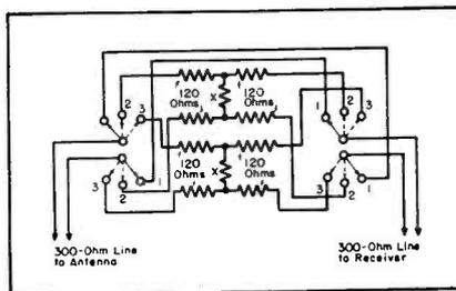
Fig. 3. A two-gang double-pole three-position selector-switch arrangement which permits insertion of pads in 300-ohm lines in those channels where the TV signals are too strong.
