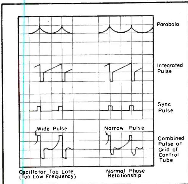
Fig. 4. Composite wave form which results when the three components (parabola, partially integrated pulse, and sync pulse) are applied to the grid across the variable horizontal lock capacitor.
