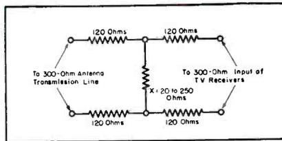
Fig. 1. Flexible pad for adjusting signal level between 300-ohm transmission line and 300-ohm receiver input.
