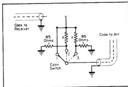
Fig. 4. Coaxial switch circuits which adds circuit attenuation on those TV channels where the TV signals are too strong.
