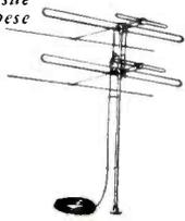
channels for which it is not adjusted. The high-frequency channel signals picked up by the low-frequency elements may have out-of-phase reflections with respect to the TV signals on the high-frequency elements, and unless the networks filter out the high-frequency signals on the low frequency rods, the high-frequency channel pictures may be marred unnecessarily by reflections.<sup>4</sup>
