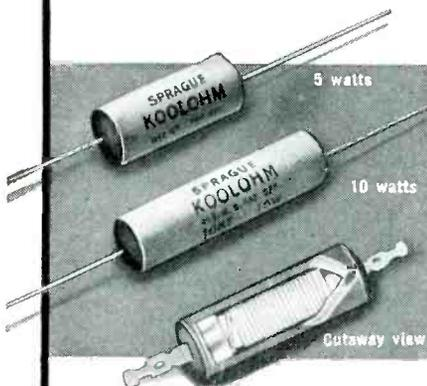
Wound with ceramic-insulated wire. More resistance in less space. Doubly protected, insulated and sealed by outer ceramic jacket. Highly resistant to moisture and heat.
