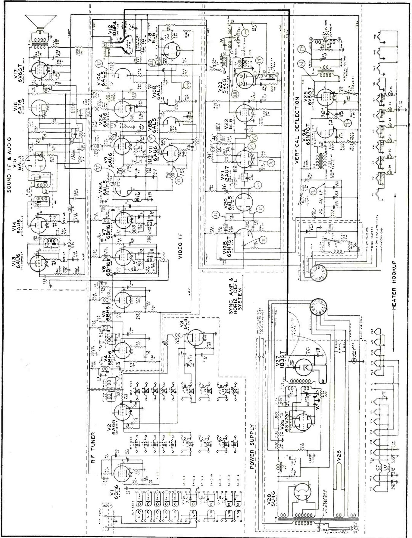
Fig. 1. Schematic of the Sparton TV chassis.
