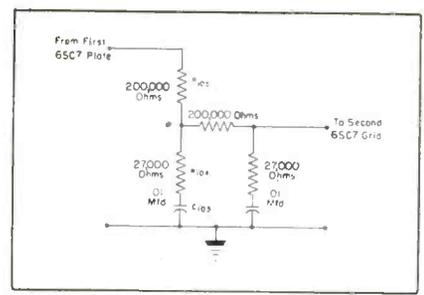
Fig. 1. Alternate If compensation circuit.
