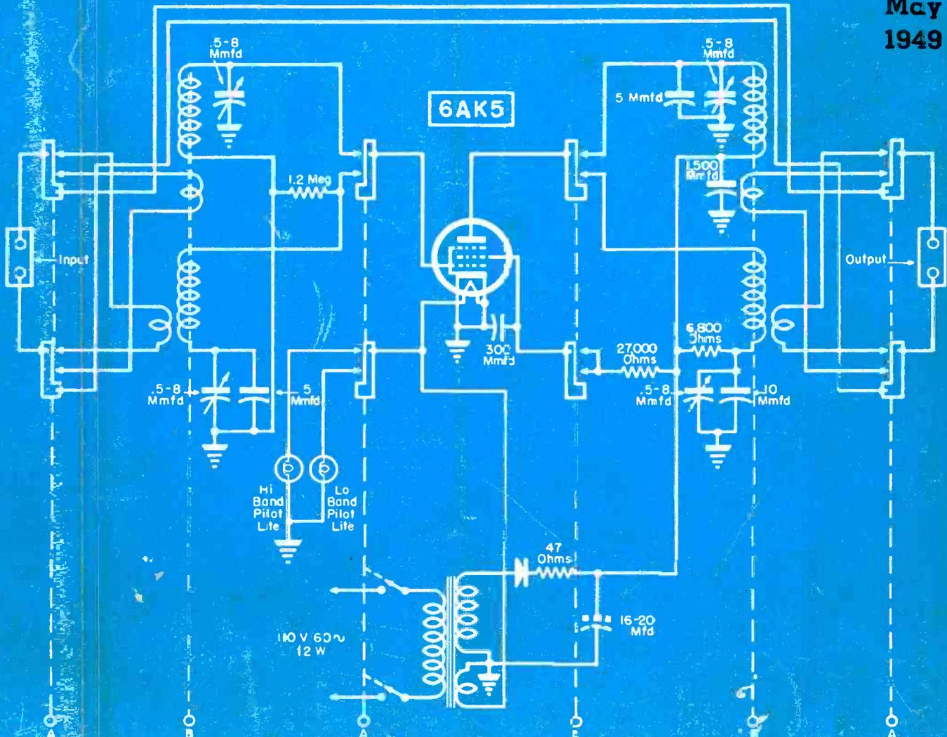
A one-tube iron-core tuned TV booster,
