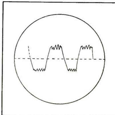
Fig. 3. Open or buffer which is too small will cause excessive peaking or pips on leading edges as indicated in this pattern.
