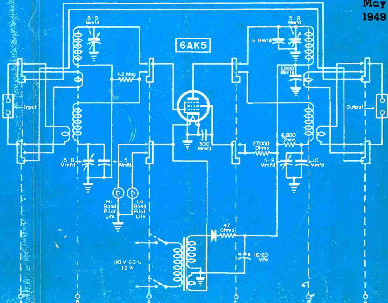
A one-tube iron-core tuned TV booster,
