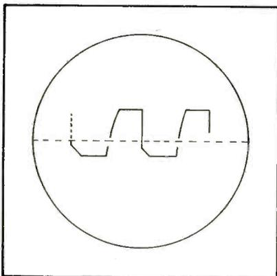
Fig. 2. Severe point bouncing will appear as a ragged top and bottom in the pattern as indicated below.
