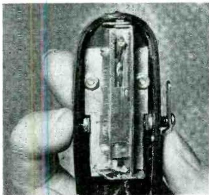
Titone type-dual needle pickup using piezo-electric ceramic element which can be employed for the standard and fine-line records. (Courtesy Sonotone)
