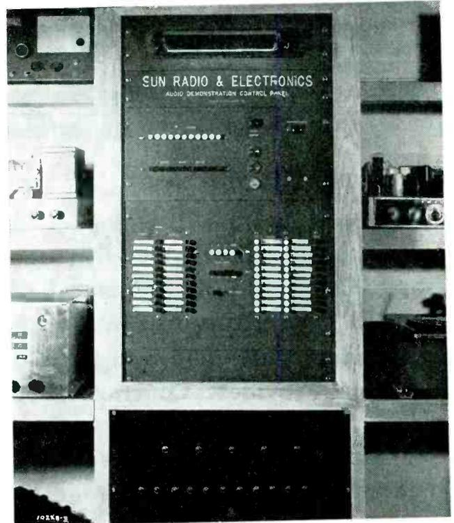
Fig. 2. Closeup of the control panel. The ac switch panel below the rack provides almost complete remote control of components. Note the impedance matching switches in the center of the push-button panel.
