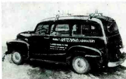
Mobile TV antenna laboratory designed to field test antennas under all types of transmitting conditions and all urban and rural topographical situations. Equipped with *hf* signal generators, transmitters, cable, etc.
