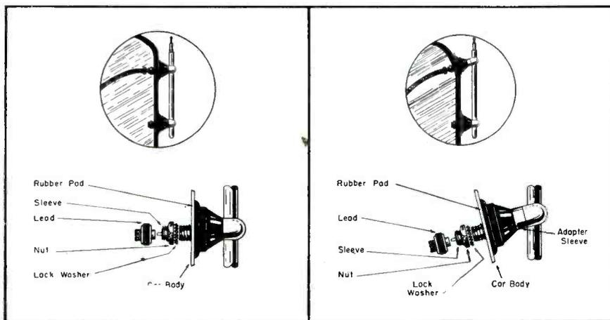
Fig. 1. How a four section side cowl antenna is installed.
