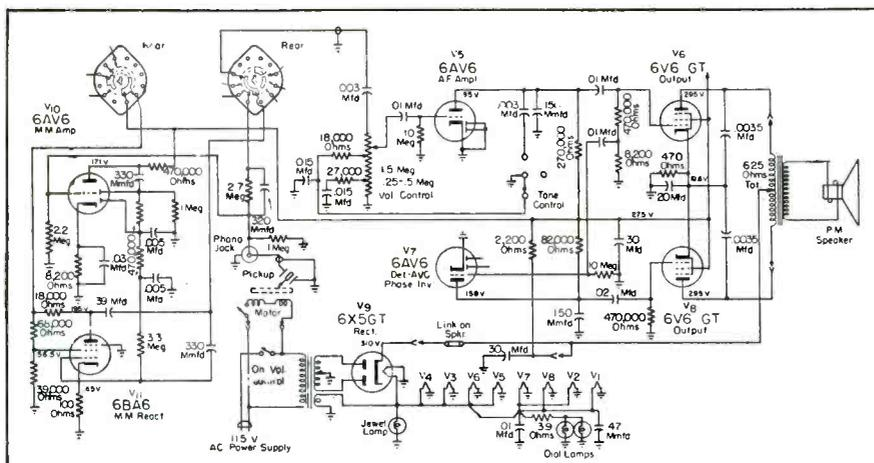
Fig. 2. The Hush-O-Matic circuit used in Bendix models 1524 and 1525.
