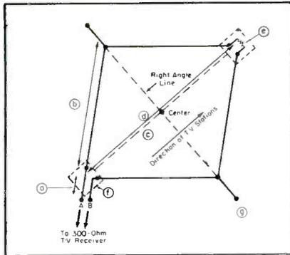
Fig. 1. Typical rhombic antenna layout for unidirectional reception; *a*, 500-ohm quarter-wavelength matching section; *b*, five wavelengths at lowest frequency TV channel; *c*, five wavelengths less approximately half wavelength to center; *d*, nine wavelengths; *e*, 800-ohm load at TV channels, in water-tight box; *f*, water-tight box for transmission-line termination; *g*, insulated supports, minimum of 10' from ground.
