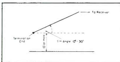
Fig. 3. A bidirectional rhombic antenna layout where the 800-ohm termination is omitted.
