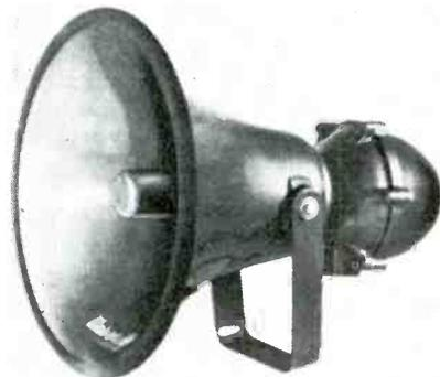
Explosion-proof speaker recently developed by University Loudspeakers, employing a reflex trumpet speaker and integral 30-watt driver, with a built-in multi-tap matching transformer. Unit is UL approved and available in model 7101 (class 1, groups C and D) and model 7102 (class 2, groups E, F and G.)
