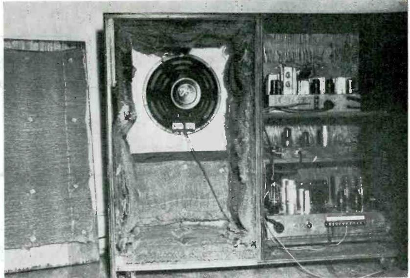
Rear view of the receiver-amplifier console. At right are the tuner, preamp equalizer and 14-watt amplifier, while at the left is the speaker compartment with treated walls.
