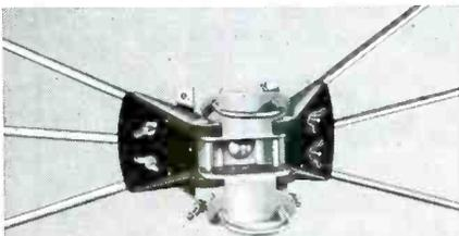
The Brach Bow Tie V insulator is a specially designed 6 element clamp, made of sturdy high impact Bakelite and heavy gauge tempered aluminum. It has real VHF insulation to minimize signal loss. Its tight grip provides a hold on the elements that wind, sleet, snow won't budge.
