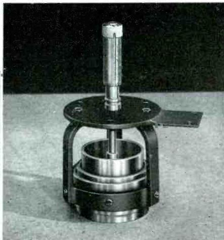
Fig. 4. Exploded view of the micrometer head, tapered rotor and tubular stator.
