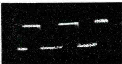
Fig. 3. Rounded wave pattern illustrating poor treble response.
