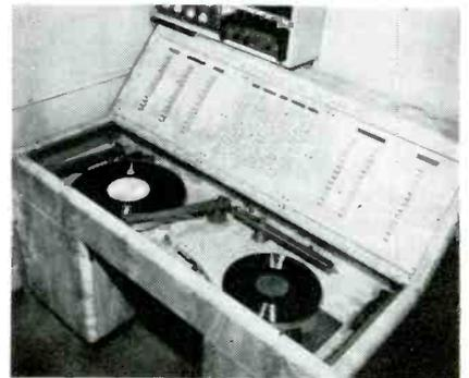
Push-button console switching system which provides instantaneous selection and playing of any one of over 371,000 different custom music component combinations. Console is connected to approximately 60 units: pickups, turntables, record changers, noise suppressors, equalizers, preamplifiers, tuners, tape recorders, power amplifiers, and speakers.
