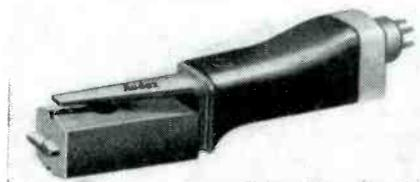
Magnetic pickup unit for 33 1/3, 45, or 78 rpm. Special connector permits the unit to be plugged into a Garrard changer arm. The point pressure is said to be 8 grams for all discs. Output is approximately 20 mv. (Polyphase reproducer L-6-G; Audak Co., 500 Fifth Ave., New York 18, N. Y.)
