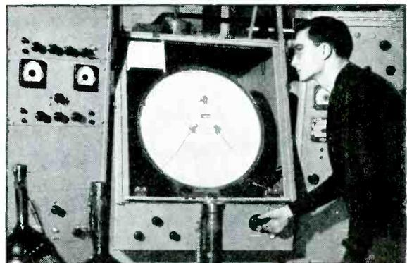
Every G-E picture tube is carefully tested for electrical and screen characteristics. Here brightness is being measured, and the screen area inspected for any blemishes. Many other tests follow. G-E tubes are pre-checked for superior performance!
