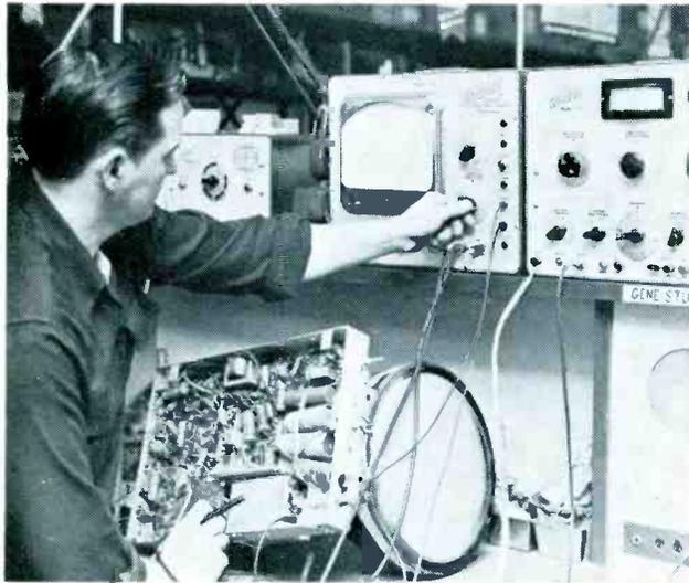
Left: A *vtvm* setup on a TV servicing bench. (Photo courtesy Mirus TV Service, Cincinnati, Ohio).
