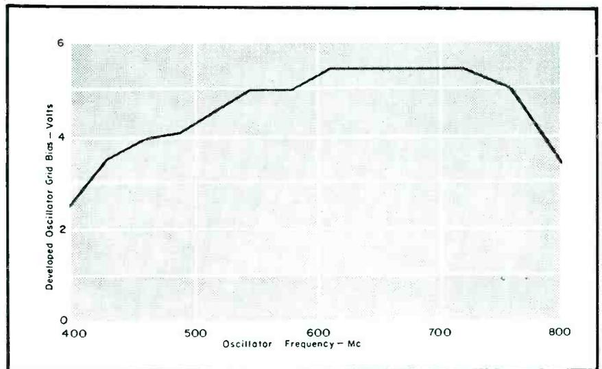
Fig. 1. Oscillator developed grid bias characteristic in *uhf* converter.
