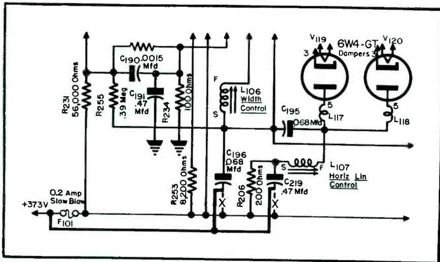
Partial schematic of RCA 21-inch TV chassis, illustrating circuit changes required for slow-blow fuse installation.
