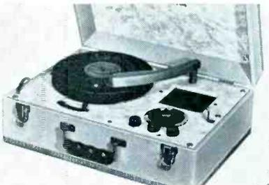
Radio and 3-speed-phono combination, which features a 5-tube ac/dc superhet, separate tone and volume controls, and instant change-over phono-radio switch. The phono consists of constant 3-speed motor, dual needle arm, and 3-tube audio amplifier. (Model 550B; Clinton Radio and Phono Corp.)
