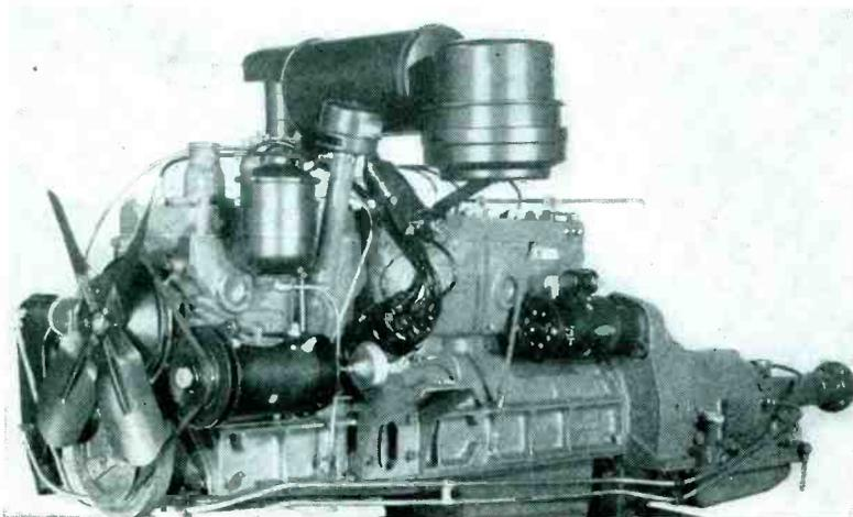
Left: View of generator, fan belt and engine in a modern car.
