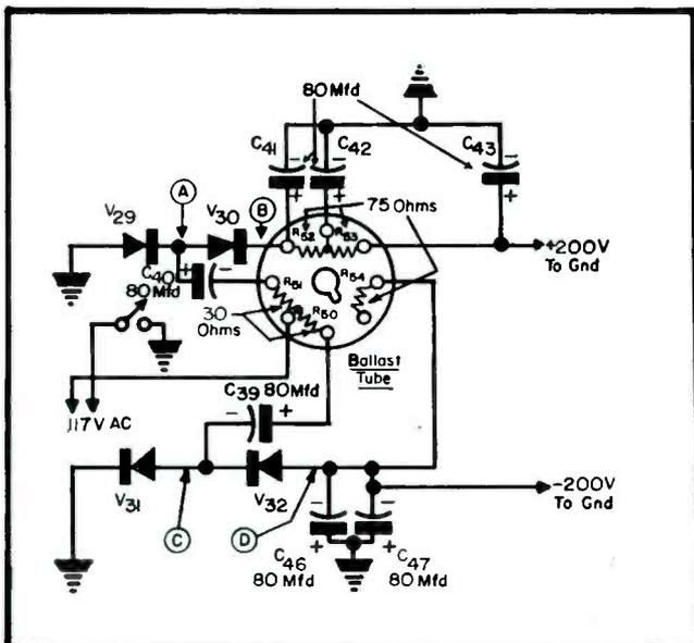
Fig. 4. A low-voltage power supply; Emerson chassis 120087B. *A*, *B*, *C* and *D* represent voltage test points.
