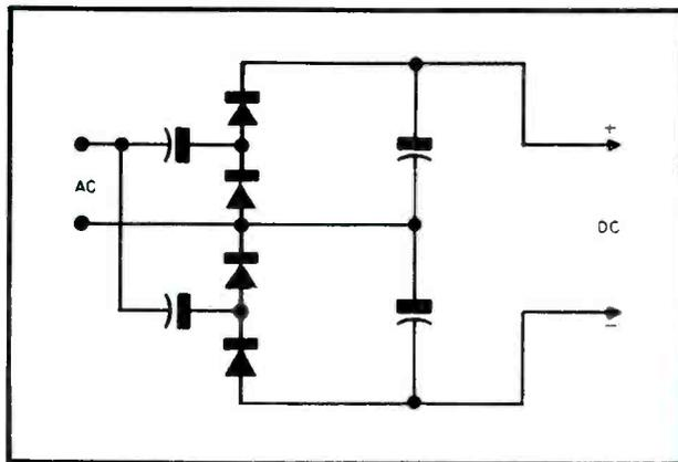
Above: A voltage-quadrupler circuit, with two half-wave voltage doublers and their ac inputs connected in parallel, and the dc outputs connected in series. The no-load dc output voltage delivered equals 5.65 times the ac rms input voltage. Thus, with an ac input voltage of 117, the dc output at no-load will be 661 volts. Voltage regulation when using 40-mfd capacitors is about 88% and about 36% when using 200-mfd capacitors. (Courtesy International Rectifier Corp.)
