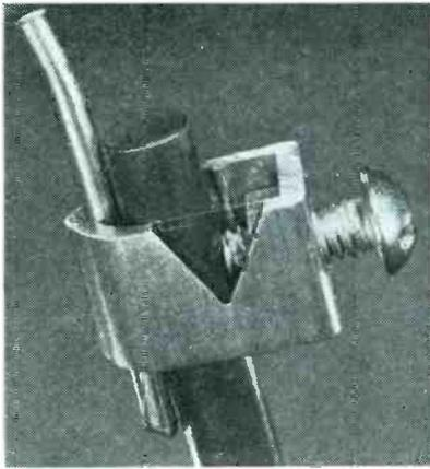
Cutaway view of ground rod with an extruded aluminum wire clamp, which will accommodate all ground lead wire from No. 3 to No. 20. Screw and nut fastening provision is said to permit wire to nest in grooved slot in the clamp. (South River Metal Products Co., Inc., 377-37<sup>th</sup> Turnpike, South River, N. J.)
