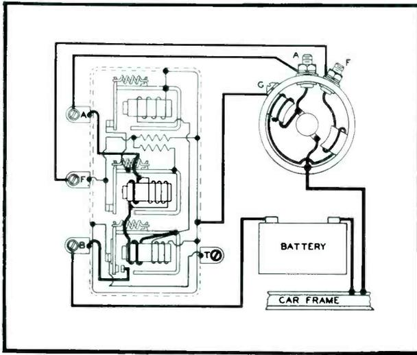
Left: Voltage regulator used in auto radio system.
