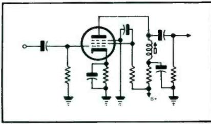
Fig. 1. A typical if-amplifier stage using a pentode.
