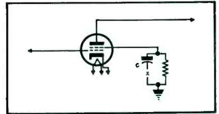
Fig. 3. Screen circuit of a beam-power tube, in which the bypass capacitor is open at X; a fault which can only be disclosed by a 'scope.
