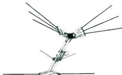
Conical-V-Beam antenna which features all-aluminum outrigger pivot plate and mating pressure plate which is said to reduce set-up time. Tightening of a wing nut grips solid dural element rods in the jaws of a 3" all-aluminum element clamp. Insulation is of laminated micarta. Has a Hi-Y reflector, integrally embodied. (Meteor E-Z-Rig available in the basic single unit ME-2X-TV, two bay array ME-4X-TV, and a four bay unit ME-8X-TV; Telrex, Inc., Asbury Park, N. J.)
