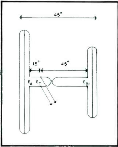
How spacing of the dipoles is accomplished in the Channel Master broad-band yagi. Dipoles are 45° apart in free space. Feed points are 15° in front of the lower frequency dipole. Higher frequency fold is fed through a length of twin lead 45° long which is transposed so that its effective length is 135°.
