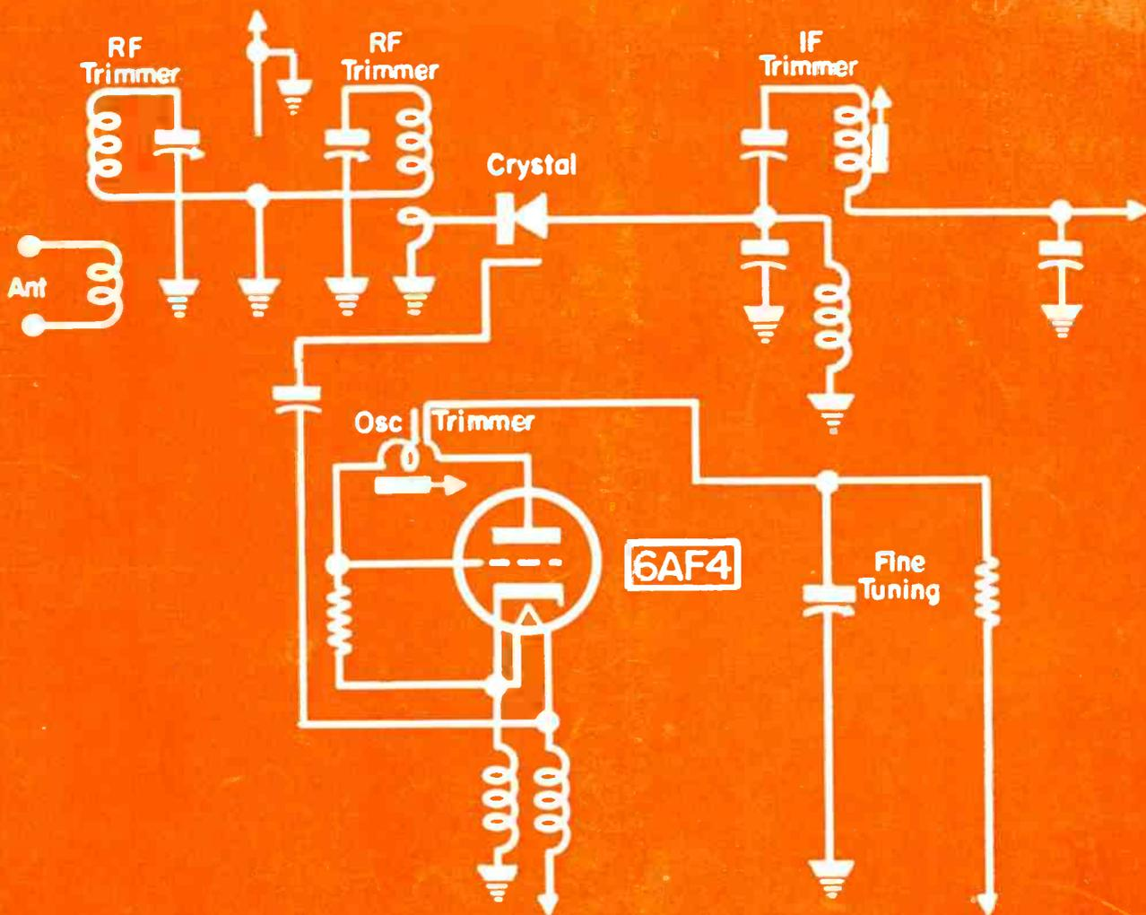
UHF receiver designed to cover the 470-710 and 670-890-mc bands.
