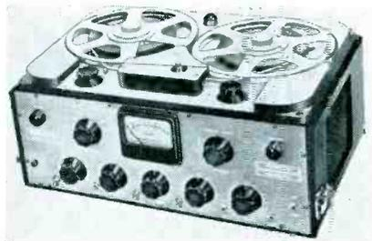
Three-speed tape recorder which plays 10½-inch NARTB reels and 5 and 7-inch reels. Has a push-pull 9-tube 12-watt amplifier. Mixing channels for mike, radio and phono input. (Tapesonic model 70; Premier Electronic Labs., 382 Lafayette St., N. Y. 3.)
