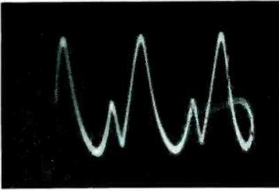
Fig. 1. Waveform with two components. A *vtvm* can indicate the voltage of the larger component, but does not reveal the presence of the smaller component.
