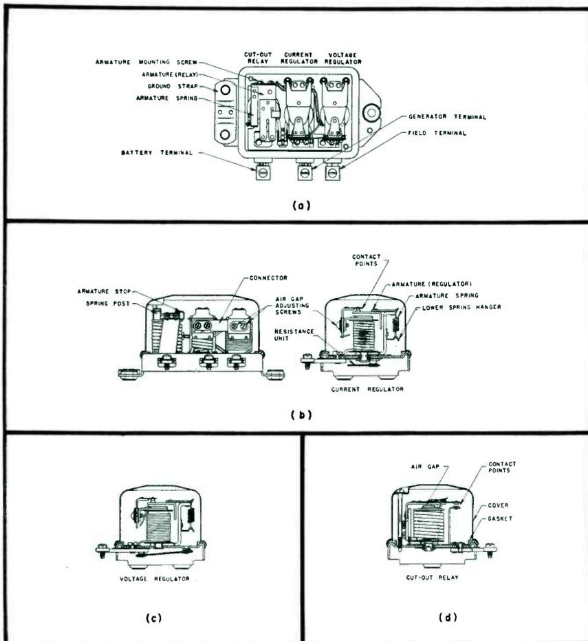
Views of current and voltage regulators (a), current regulator (b), voltage regulator (c) and cut-out relay (d).
