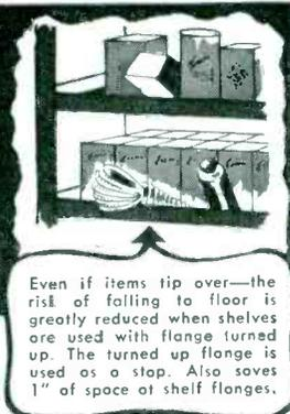
Even if items tip over—the risk of falling to floor is greatly reduced when shelves are used with flange turned up. The turned up flange is used as a stop. Also saves 1" of space at shelf flanges.
