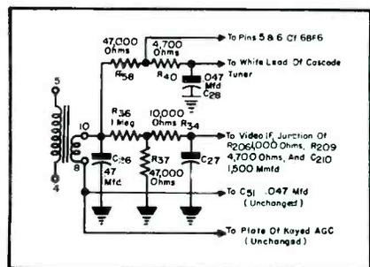
$R_{41}$  (33,000 ohms) may be removed also. These two resistors should be altered as suggested to suit experimentally the general performance of the chassis in question because of varying inherent sync levels.
