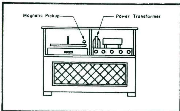
Fig. 1. Layout of components which involves danger of hum pickup: Power transformer and magnetic cartridge are too close to each other.
