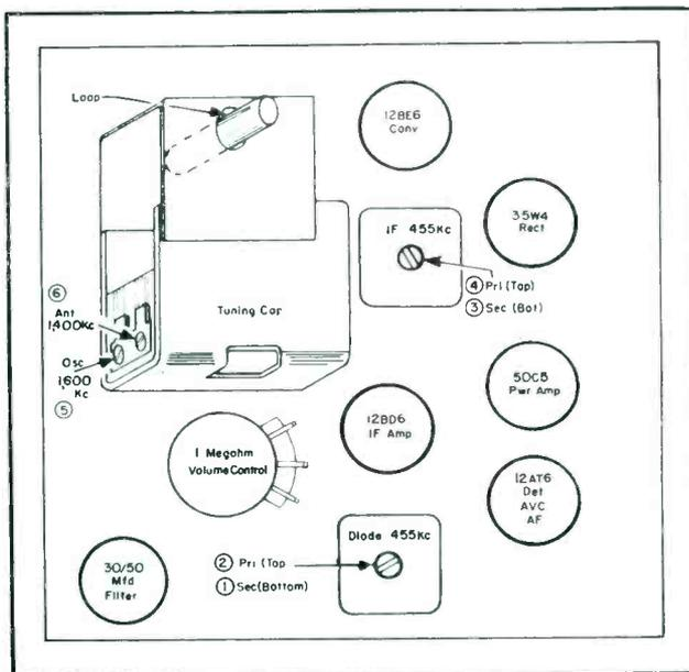
Fig. 3. Motorola pc chassis tube and trimmer locations.
