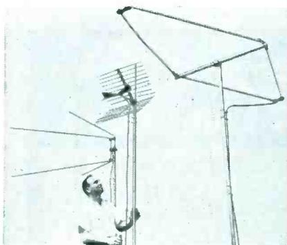
Above, line of *uhf* antennas: single and stacked Vs, corner reflectors, and rhombic. Stacked V antenna is a broad-band *uhf* type. Diameter of the rods is 4", while the dipole's lengths is 55". Stacking is approximately 1/2 wavelength apart at lowest operating frequency. Corner-reflector is claimed to offer up to 12 db gain. The reflector grids are of solid aluminum.
