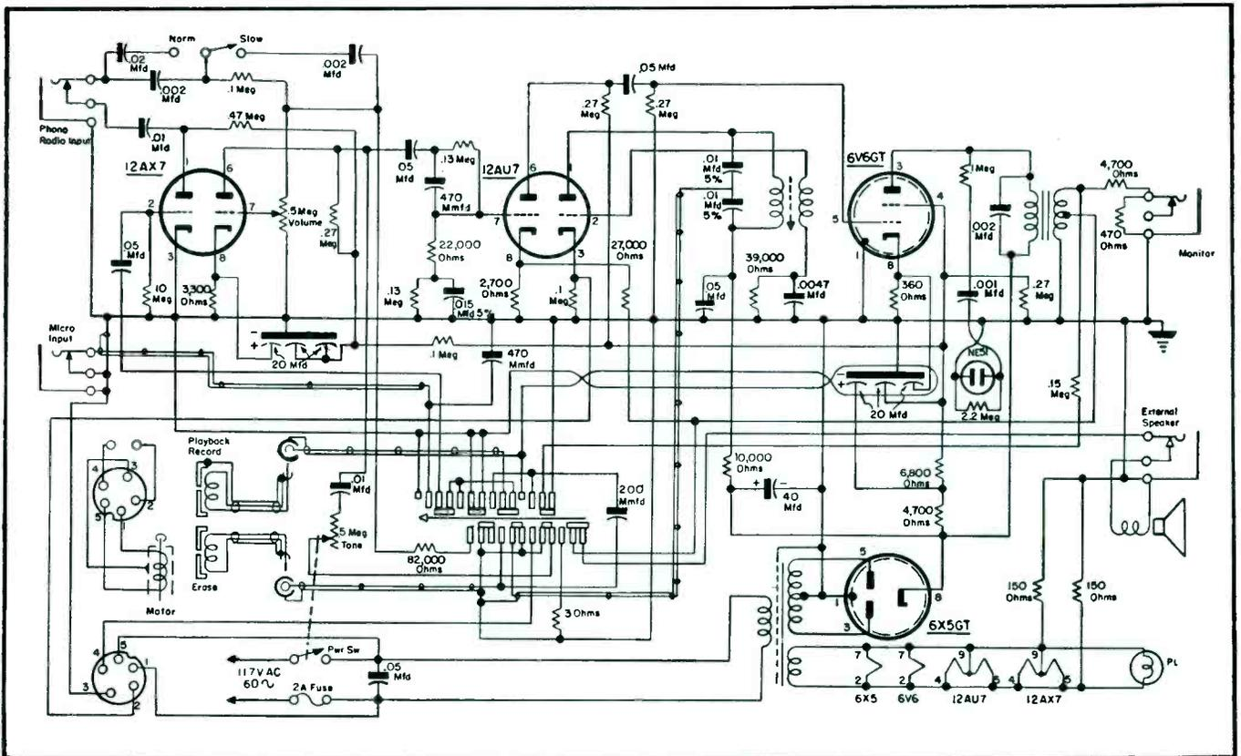
Fig. 1. Circuit of three-speed dual-track tape recorder; Bell Sound System model RT65B.
