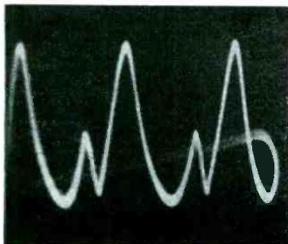
Fig. 2. Energy content of a very narrow pulse is small. The small energy requirement of a 'scope permits it to reproduce pulse correctly, but a peak-to-peak *vvm* will read a subnormal voltage.
