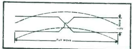
Fig. 2. When dipoles cut for a full wavelength are placed one above the other a half wave apart the incoming wave striking the dipoles will occur at the same instant; therefore the electrical charge on each element will be in the same phase, voltage and current.
