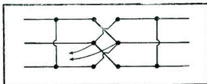
Fig. 4. Tying of elements together found to provide a better impedance match to transmission line.
