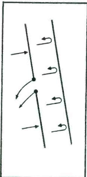
Fig. 1. Representation of concept that reflector is an element placed in a horizontal plane behind a dipole at the proper spacing and length to permit forward gain, a gain that is said to occur by waves inducing a current in the reflector element and radiating back to dipole in phase with incoming signal.
