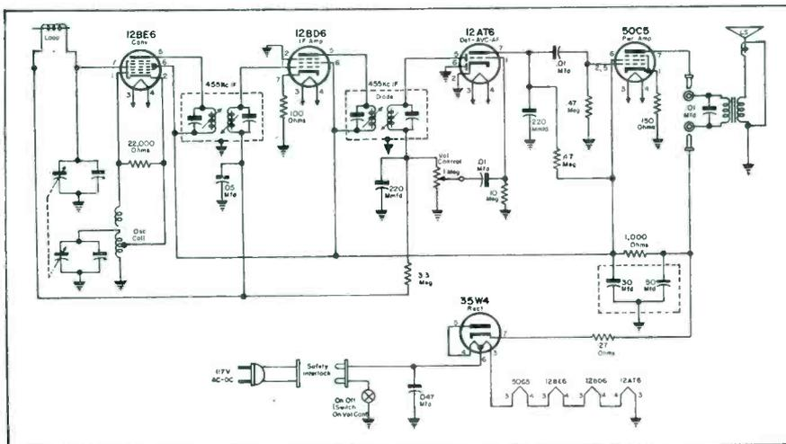
Fig. 2. Schematic of the Motorola HS-289 plated-circuit chassis.
