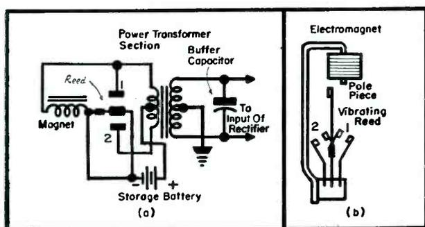
Fig. 1. At left, schematic of simple vibrator circuit. The vibrator is a shunt-fed one. At right appears a pictorial sketch of the vibrator shown at left.
