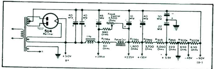
Fig. 1. Low-voltage power supply used in Capehart CX-33, showing resistive voltage divider employed to obtain different voltage outputs.
