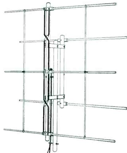
Fig. 6. Forward gain regenerative TV antenna. (Model 45-4F; Barb City Industries, Inc., 1150 S. Fourth St., DeKalb, Ill.)
