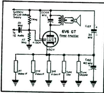
Fig. 2. An example of tube voltage-divider circuitry; a  $\mu a$  stage in series with a parallel group of three video *if* stages and two sync stages.
