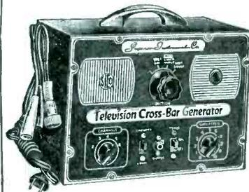
Power Supply: 105-125 Volt 60 Cycles. Power Consumption: 20 Watts. Channels: 2-5 on panel, 7-13 by harmonics. Horizontal lines: 4 to 12 (Variable). Vertical lines: 17 (Fixed). Vertical sweep output: 60 Cycles. Horizontal sweep output: 15,750 Cycles.
