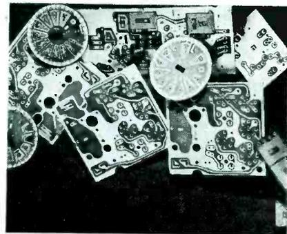
Above: Variety of circuit designs and layouts produced by Motorola pc process, in which a thin copper pattern is applied to a die-stamped plastic base.
