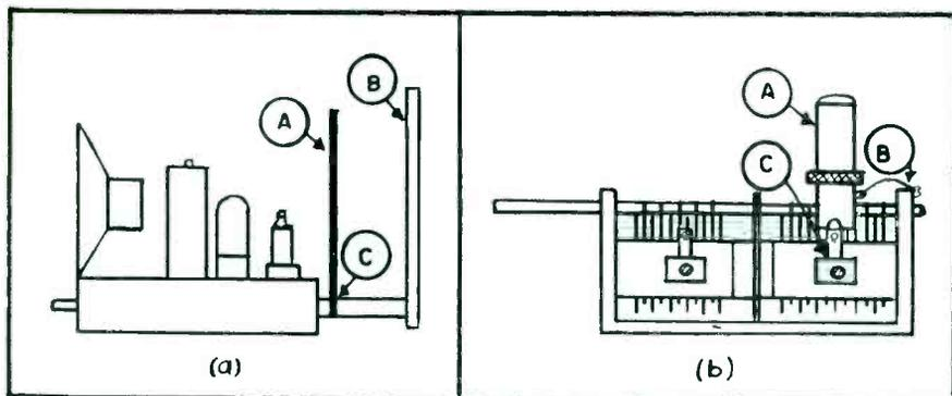
Fig. 1. At left is illustrated position of metal shielding added to *ac/dc* chassis to prevent oscillation at low-frequency end of the dial: *A* represents the added metal shield; *B* is the loopstick and *C* is the ground to chassis at two or more points. At right, the ferris-loopstick mounting is illustrated; *A* is the loopstick; *B*, connection from stick to frame of capacitor or *avc*; and *C* is the hot wire to lug on the antenna trimmer
