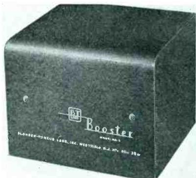
Automatic booster; 3-stage amplifier which it is said will deliver in excess of 18 db over all channels. Uses a cascaded circuit and three dual triodes. Additional features include automatic on-off operation with TV set, a switch for attenuating strong signals and *uhf* adaptability. (Model HA-3; Blonder-Tongue Laboratories, Inc., Westfield, N. J.)
