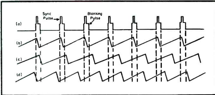
Fig. 1. Relationship of sync pulse to deflection waveform.
