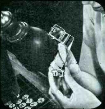
Completed mounts are inspected for visual defects.
