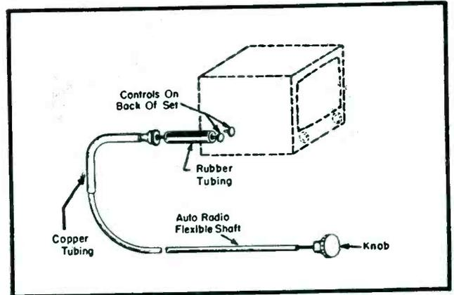
Fig. 1. Flexible shaft extension designed to permit adjustment of rear controls on TV receivers. Copper tubing is helpful in controlling degree of bend to prevent binding. Short length of rubber tubing can be cut from windshield wiper hose. (Courtesy Motorola.)
