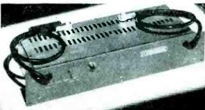
been devised for the community setups. For one, two, or three channel service, for instance, there is available a tower amplifier system.<sup>1</sup> The equipment is used specifically for boosting the incoming TV signals to a level sufficient for carrying them to the next amplifying station. Associated converter equipment is used with the tower amplifier system for conversion of the incoming frequencies to those used in the outgoing channels of the tower amplifier.
