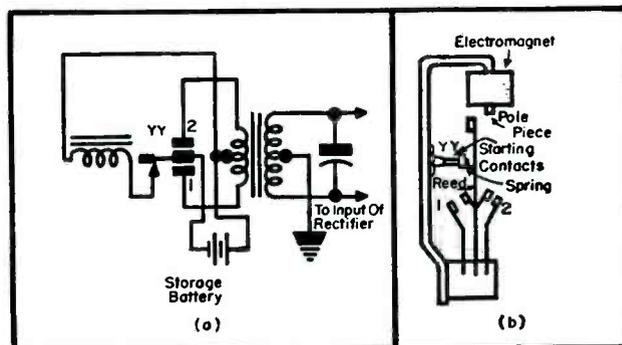
Fig. 2. At left, series-fed vibrator schematic. At right, a pictorial sketch of the vibrator.
