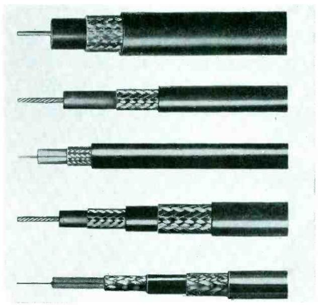
TV coax designed for community installations. From top to bottom: primary leadin; secondary leadin; tapoff leadin; and secondary and tapoff leadin used where radiation exists. (K-14, RG11/U, RG59/U, SP-75 and SP-76; FTR).
