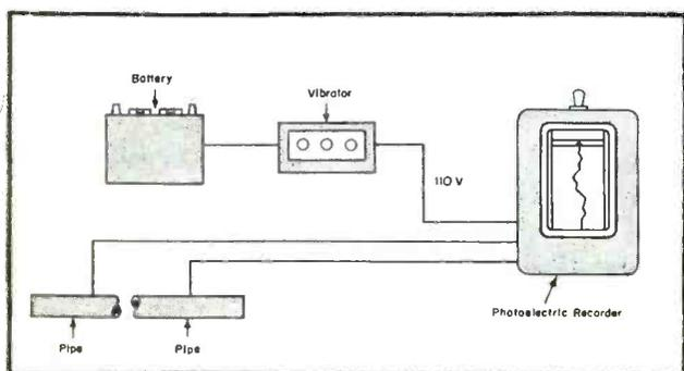
Fig. 2. Complete Pacific Evenness Tester, which uses a photoelectric unit to provide a record of the evenness of the textile material under test.
