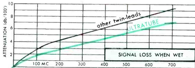
ULTRATUBE and other twin-lead constructions were tested under both wet and dry conditions. The data clearly show that for clear, strong signals under adverse weather conditions, no transmission line gives better reception than Synkote ULTRATUBE.
