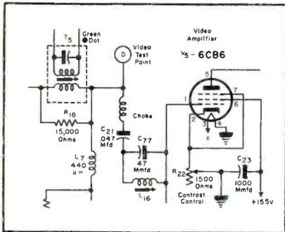
Figs. 3 (top) and 4 (bottom). Black horizontal streaks over the picture, when tuned to channel 6 in 120169 (triangle A to D) Emerson chassis, may be eliminated by connecting a 10- $\mu$ h *rf* choke in series with .047-mfd capacitor; Fig. 3. Same remedy may be applied in 120169 (triangle E or higher) chassis; Fig. 4.
