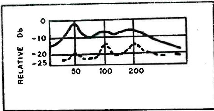
Fig. 3. Comparative rumble level of inexpensive (solid line) and high-quality (dashed line) turntable motor. (Based on Briggs data.)
