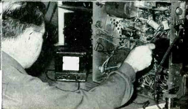
2. **LOCATING THE SHORT**—With Loadchek you can quickly check the shorted side, part by part, without laying down tools or picking up test leads. Here, the trouble was a short in the transformer, spotted without having to warm up set. Overloads are found the same way.
