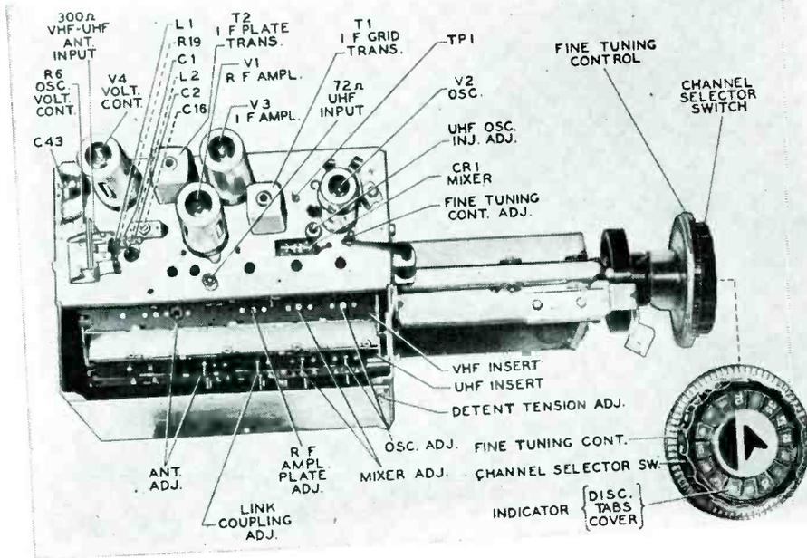
is made possible by tuned inserts which are placed within a drum assembly in the *rf* tuner. A 2:1 step-down ratio is used in the turret drive assembly to rotate the drum.
