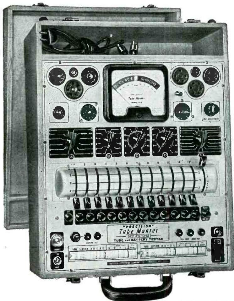
To test modern tubes for only one characteristic will not necessarily reveal **OVERALL PERFORMANCE CAPABILITIES**. Modern tube circuits look for more than just mutual conductance or other single factor.
