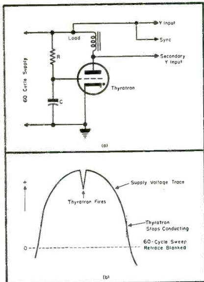
Fig. 6. Circuit used to determine firing point of thyatron appears in *a*. At *b* is a trace showing thyatron operation.
