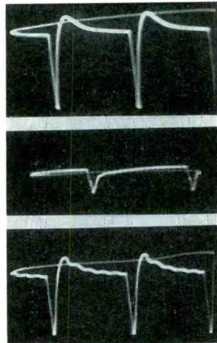
Fig. 4. Additional examples of normal and abnormal waveforms in horizontal sweep system: A (top) = secondary voltage during normal operation; B (center) = secondary voltage when there is a short in secondary winding; C (bottom) = secondary voltage, when circuit is ringing.
