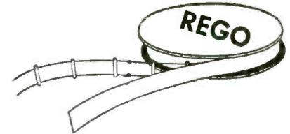
A 300-ohm transmission line with No. 18 copper or copperweld, and polystyrene spacers 4½" apart. (Rego Insulated Wire Co.)
