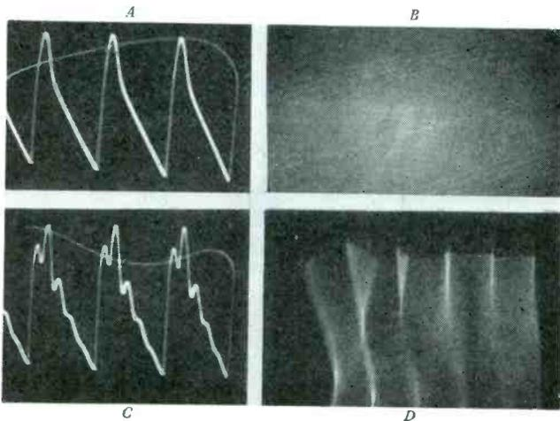
Fig. 3. Other examples of normal and abnormal waveforms in horizontal sweep system: A = normal damper current; B = damper current, when circuit is ringing; C = damper input voltage under normal operation; D = damper input voltage, when circuit is ringing.
