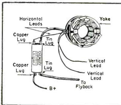
Fig. 5. Circuit illustrating installation of horizontal reframer. Fig. 5a. Three types of horizontal reframers available to compensate for low line voltage which can lead to horizontal shrinkage. (Courtesy Gemco)
