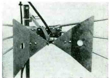
A *uhf* antenna adaptor; an all-channel, *uhf* triangular dipole. A preassembled unit, it can be fastened to the front end of *super fan*. The distance is said to be pre-fixed, and the *uhf* dipole is veed forward so that it is always parallel to the *vhf* fan elements which function as a sheet reflector. Designed for use with separate *vhf* and *uhf* leads to TV set or converter. (Model 415, Econo-Dapter; Channel Master.)
