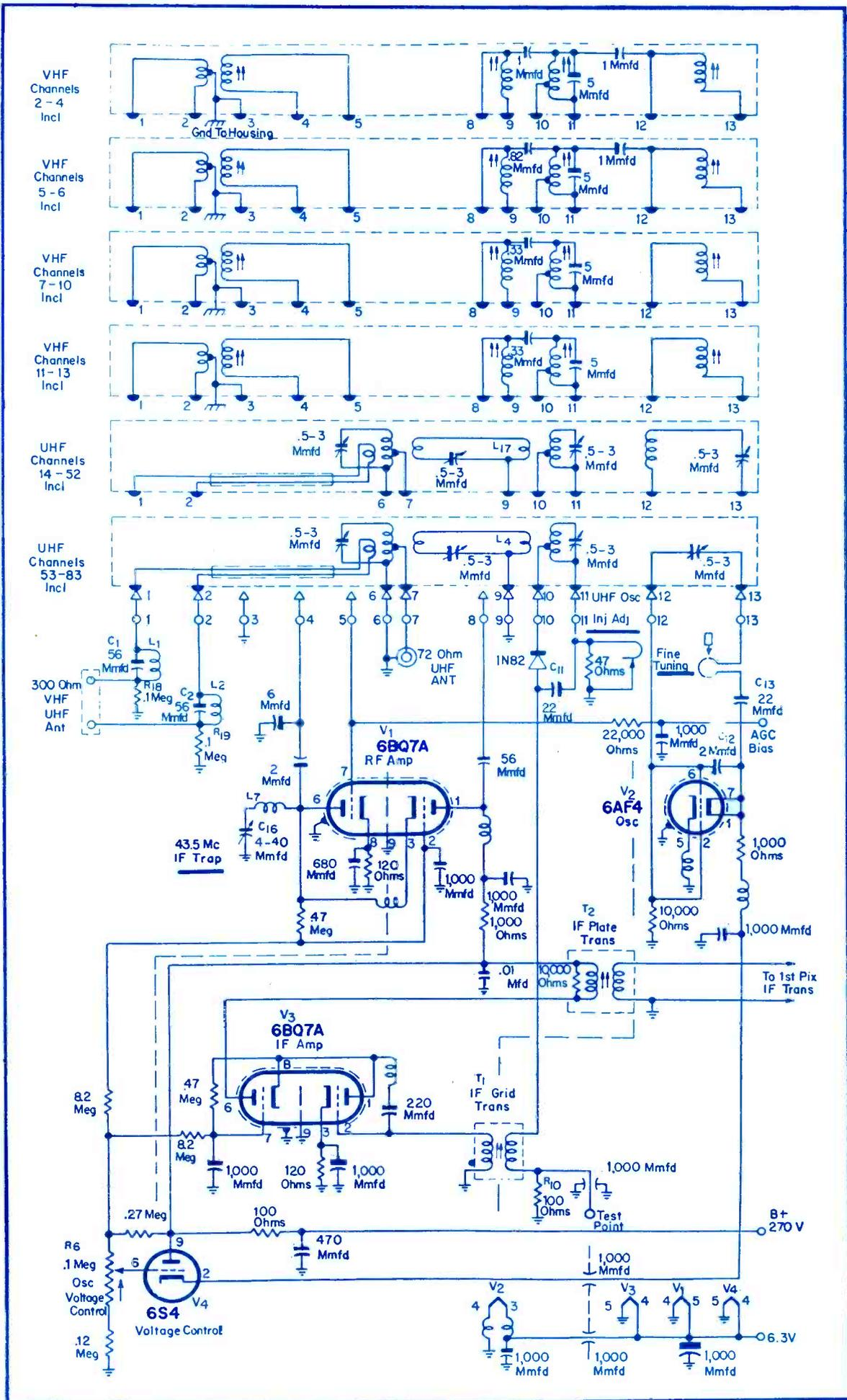
Fig. 3. Schematic of 44/44/44 tuner<sup>2</sup> with which it is possible to provide coverage of any combination of 16 vhf and 44 hf stations, through the use of tuned units which are inserted in a drum assembly in the rf tuner.
