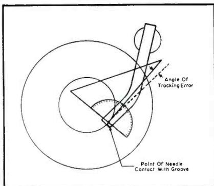
Fig. 6. How a change of cartridge or needle from the original design can change the correct overhang and introduce increased tracking error.
