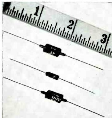
Point-contact germanium diodes developed for video detectors, *uhf* mixers to 900 mc, as well as for general-purpose operation up to 200 volts. Stiff terminal pins are said to permit clipping of the unit into spring terminals either for test or for circuit application; flexible leads permit soldering or other suitable connection means. Types available include NU38, NU39, NU58, IN48, IN51, IN64, IN65, IN69, IN72, and IN81. (Transistor Division, National Union Radio Corp.)
