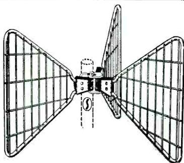
Bow-screen uhf antenna for channels 14 to 83 and vhf channels 7 to 13. Has two fan type galvanized elements. Other features are a thermostetting plastic mount, and U-clamp mast mounting. (UHF-2; Snyder.)
