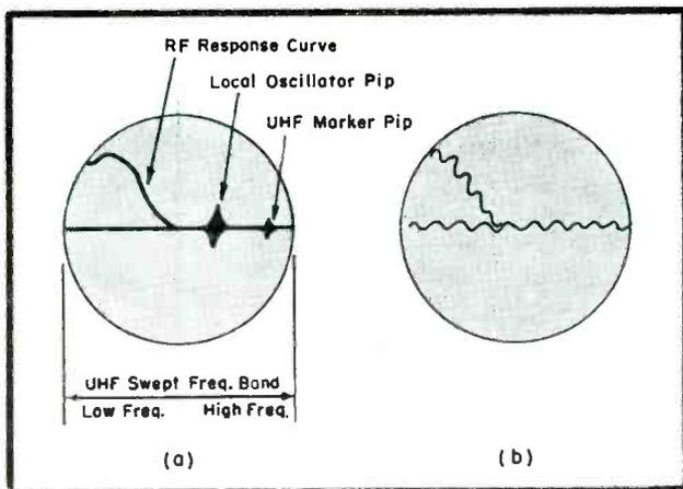
Fig. 2. Patterns obtained when aligning *uhf* local oscillator by the beat-frequency method. Wavelform in a shows result when the local oscillator frequency is lower than the *uhf* marker frequency. A 'scope presentation showing the local oscillator frequency and *uhf* marker producing a low frequency beat frequency, and correctly aligned local oscillator, appears in b.
