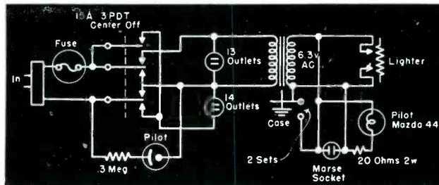
Fig. 6 (above). Circuit of bench outlet.
