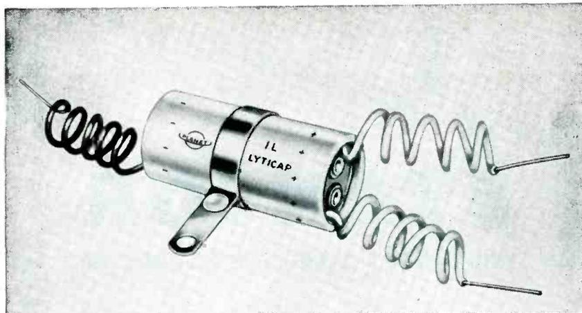
NEW DUAL SECTION ELECTROLYTIC CAPACITORS HERMETICALLY SEALED IN ALUMINUM TUBES WITH COMPLETELY FLEXIBLE INSULATED LEADS. By riveting the leads directly to the condenser end disc, Planet has eliminated the use of rigid terminal risers ordinarily used on this type construction. This allows Planet Type IL capacitors to fit into a smaller space and eliminates the possibility of lead breakage.
