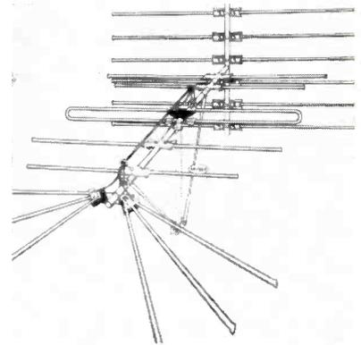
Combination conical-yagi TV antenna with radar-flector. Factory preassembled. Available in single array and 2-array models. Employs seventeen hi-tensil 3/8" aluminum elements, three perma-plastic insulators, a six-element radar-flector, plus a universal U clamp, crossarm support and 60" twin lead phasing stub. (Texas Ranger models AX673 and 674; Snyder Manufacturing Co., Phila., Pa.)
