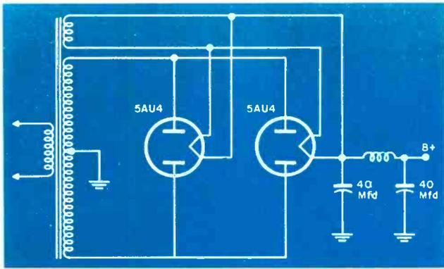
Fig. 2. Conventional full-wave power supply using pair of 5AU4s in parallel with capacitor-input filter.
