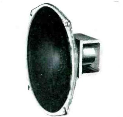
Eight-inch extended range speaker with 6.8-ounce Alnico V magnet, a power rating of 15 watts and a response up to 12,000 cps. It is equipped with an aluminum voice coil. (Model 850; G.E.)
