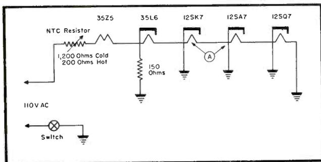
Fig. 4. Locating open filament in series string with voltmeter or neon test lamp. Full-scale meter reading must equal full line voltage; 150 vac scale preferable.
