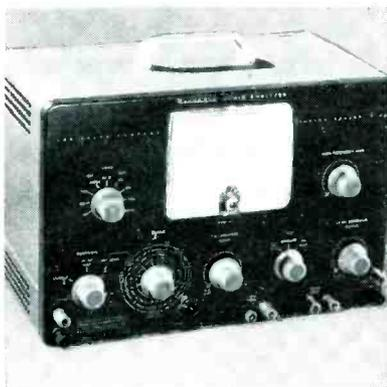
Audio analyzer said to function as three instruments in one; ac vtvm, wattmeter, and intermodulation distortion analyzer. Features built-in low and high-frequency oscillators. (Model AA-1 (kit); Heath Company, Benton Harbor, Mich.)
