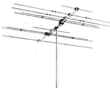
Antenna with a patent-applied-for phasing method (Miracle Phase), said to isolate undesirable interaction and loading of phased elements. Phase inverting element is claimed to permit low-band dipole to function with proper gain and pattern response in high band. (Sabre Senior; Welco Manufacturing Co., 225 S. Third St., Burlington, Iowa.)
