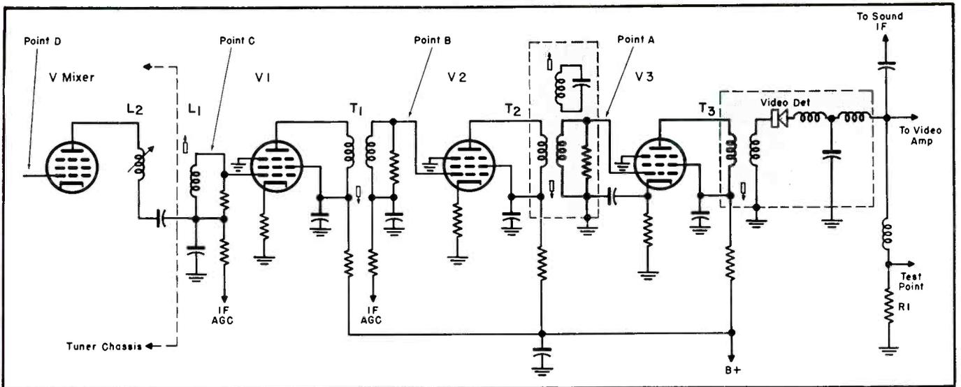
Fig. 1. A typical stagger-tuned if system, including the mixer stage of a tuner, shown because in most receivers the mixer is involved in if alignment; a, b, c and d represent alignment test points using an unmodulated signal generator and a vtvm.
