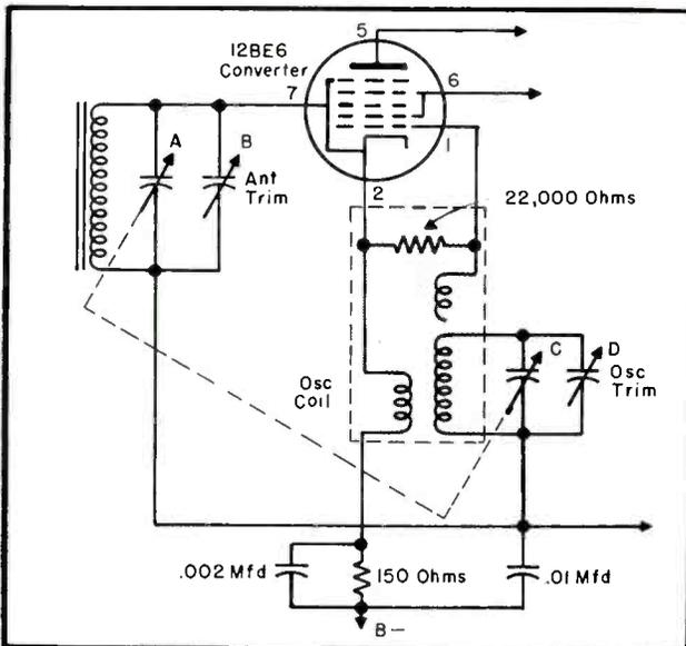
Fig. 1. Modified 12BE6 converter circuit in Westinghouse V-2236-1 chassis.
