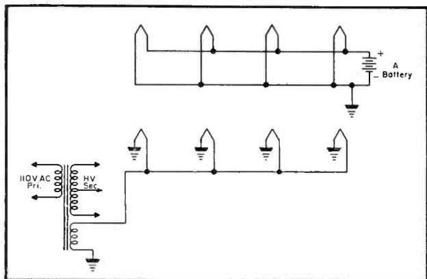
Fig. 1. A typical parallel-heater string, as found in old battery and straight, transformer-powered *ac* sets, and auto radios. It will be noted that one side of this type string may be grounded and one hot wire run to each tube.
