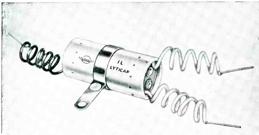
NEW DUAL SECTION ELECTROLYTIC CAPACITORS HERMETICALLY SEALED IN ALUMINUM TUBES WITH COMPLETELY FLEXIBLE INSULATED LEADS. By riveting the leads directly to the condenser end disc, Planet has eliminated the use of rigid terminal risers ordinarily used on this type construction. This allows Planet Type 1L capacitors to fit into a smaller space and eliminates the possibility of lead breakage.
