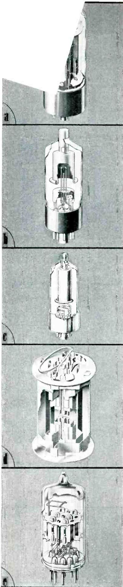
THE FUNCTION OF THE color TV receiver is to reconstruct the red, green, and blue video signals and thus reproduce the original scene both in brightness and color. To provide this performance, the color set requires many more stages and is considerably more complicated than the monochrome models.
