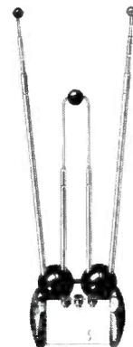
Indoor push-button antenna for uht, vhf and FM. Stands 17" high when collapsed, and sits on  $4\frac{1}{2}$ " base. Comprised of two 3-section stiffs jutting out of both sides of the base and one dual phasing bar in center which can be raised or lowered. Stiffs can be extended to 41". (Model 5D Directronic 8-Position Push Button; Synder Manufacturing Co., Philadelphia, Pa.)
