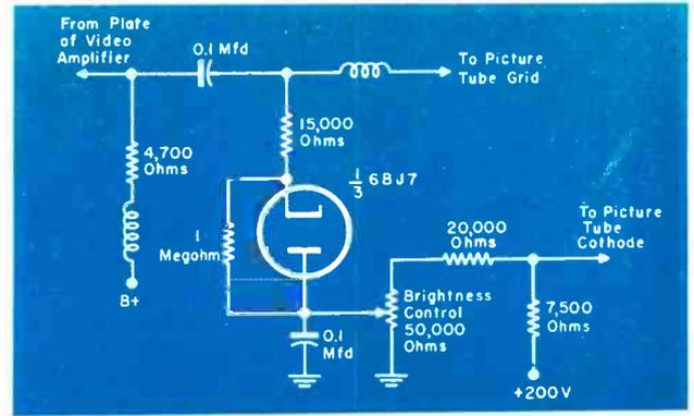
Fig. 3. Schematic of a dc restorer in which one section of the 6BJ7 is used as a dc restorer for one of the signal channels. Circuit shown is for a negative-going signal.
