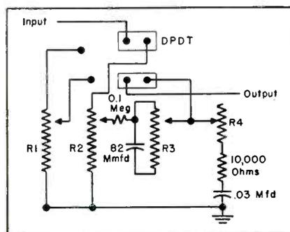
Fig. 1 (left). Readily-assembled unit for demonstrating loudness control. Input lead goes to circuit point to which hot side of receiver's volume control originally connected; the output lead goes to the point where the center tap originally went. (Courtesy IRC)
