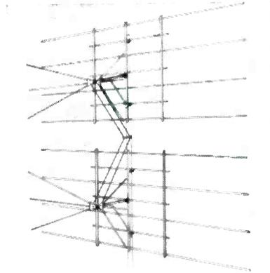
Conical-V-Beam screen array, designed around a single-bay unit, elaborated into a two-bay structure, by addition of specially designed stacking transformers. Model is produced under patent 23,346. The screen reflectors are dimensioned to provide in-line, single lobed directional pattern in both horizontal and vertical planes, at all frequencies. Features all-aluminum construction. (King Pin model 201 (single bay) and 202 (two-bay stacked); Telvex, Inc., Asbury Park, N. J.)
