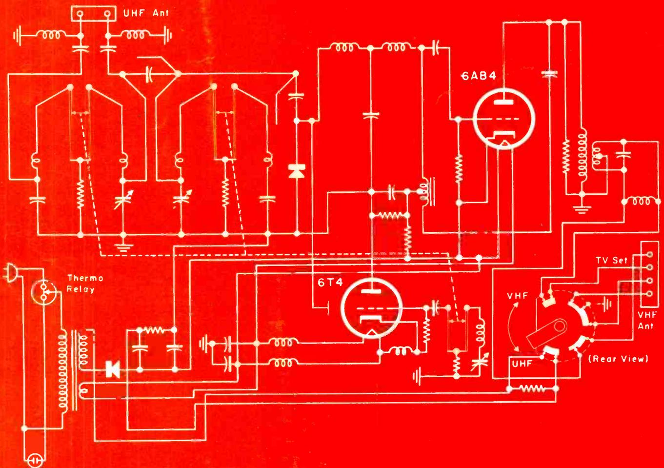
UHF converter with neutralized grounded-cathode if amplifier.
