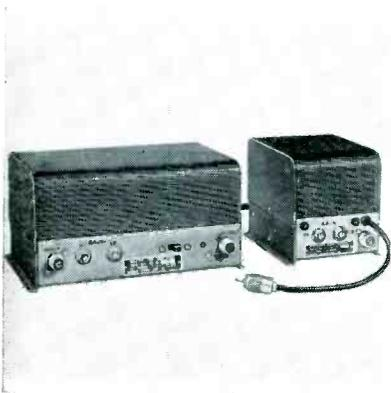
Broadband TV amplifier with auxiliary a.c. Includes cascade circuits said to deliver more than 37 db gain on vhf channels. Four tubes operate on the high band and three on low band. Maximum output is 1.25 v rms on each band. Has 75-ohm input and output coax fittings, and separate high and low-band gain controls. (Model MLA; Blonder-Tongue Labs, Inc., 520 North Ave., Westfield, N. J.)
