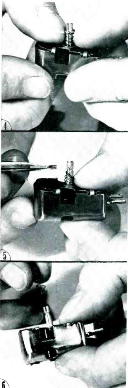
Figs. 4, 5 and 6 (top to bottom): With the v-r cartridge-held stylus side down, tension spring is compressed slightly with thumb nails. Then, holding spring depressed slightly with thumb nail, the C washer is removed with tweezers. Care should be exercised at this point to prevent spring from being lost. After the C washer has been removed, the tension spring can be lifted from shaft.
