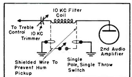
Fig. 2. The 10-kc filter circuit of Magnavox CR 204, 211 and 231 chassis, with a shorting switch that kills filter and extends range to beyond 15 kc, when used for phono.
