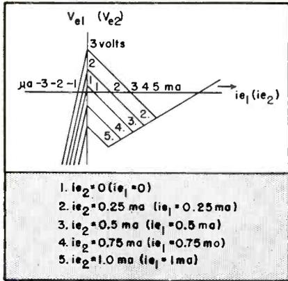
Fig. 3. Emitter negative-resistance characteristics as a function of current of a second emitter.
