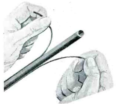
Strip-Ease 300-ohm twin lead; to strip, wire is slit down about 1" on both sides of the wire inside indicated groove and lead is ripped to the desired length. Contains 7-strand 20-gauge copper conductors. Center tubular section, it is said, stays intact as the wall covering is never cut. To keep out moisture, the center section can be sealed by heating end with a match and closing tightly with a pair of pliers. (The Radix Wire Co., 26260 Lakeland Blvd., Cleveland, O.)
