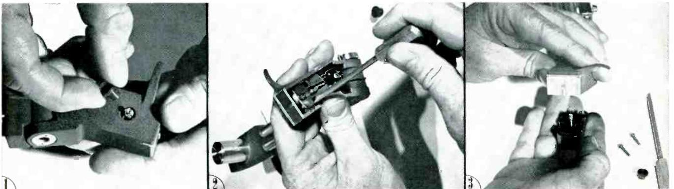
Figs. 1, 2 and 3 (left to right): In removing dual stylus from v-r cartridge selector knob is first pulled off with fingers. Then a screwdriver is used to remove mounting screws. With selector knob and mounting screws removed, cartridge is dropped from tone arm. (See pp. 49 and 50 for additional stylus-removal photos.)
