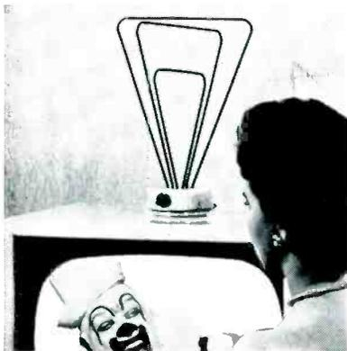
Indoor antenna, designed for metropolitan and suburban area reception, with a built-in, electronic rotating and tuning control. Tuning control changes directivity, by automatically selecting the correct combination of elements. (Star; Waisco Electronics Corp., 3602 Crenshaw Boulevard, Los Angeles 16, Calif.)
