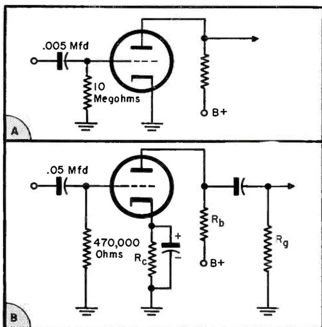
Fig. 1 a and b. In a appears a contact potential bias circuit; conversion of a to cathode-bias circuit is shown in b.
