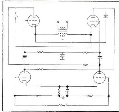
Fig. 4. Feedback-proportioning circuit in Circlotron.
