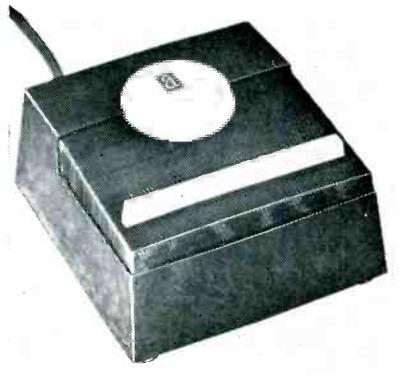
Antenna rotator with control box featuring a fingertip bar which rotates antenna in one direction when pressed on one end and in the opposite when pressed on the other end. Model consists of a rotator unit, enclosed in split die-cast zinc housing. Automatic center disk signal light indicates when limit of travel in either direction is reached. Speed of the new unit is approximately 2 rpm. Has magnetic brake to prevent drifting. (Model K-22 Tenna-Rotor; Alliance Manufacturing Co., Alliance, O.)
