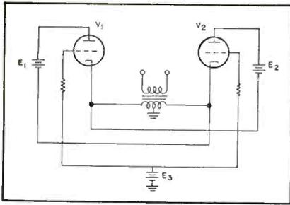
Fig. 2. Transposition of Fig. 1 into more conventional format, showing circuit in simplified form with batteries in place of power supplies.
