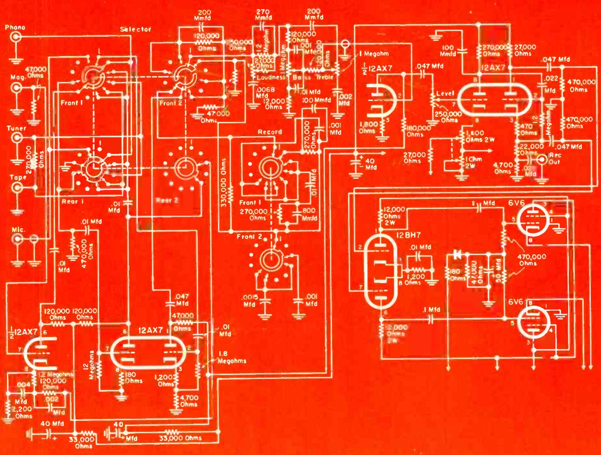
Integral 20-watt unity-coupled amplifier with preamp and tone controls; arrows indicate connections to power supply. [See circuit analysis, this issue]
