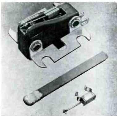
Single-needle ceramic cartridge available in two versions; one for 33's and 45's, and the other for 78's. Does not require either equalizers or preamp. Output voltage is one volt on microgroove records. Replacement needle (model N1P) snaps into place and is available with either diamond or sapphire tip. (Model 1P; Sonotone Corp., Elmsford, N. Y.)
