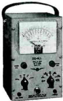
Quickly, accurately, the DO-ALL Model 655 gives a true reading measurement of complex and sinusoidal voltages with necessary peak-to-peak or RMS value read directly, for the analysis of waveforms in video, sync and deflection circuits.
