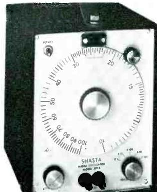
Audio oscillator which covers 10 cps to 1 mc in 5 steps. Will drive impedances from 600 ohms. Output level is  $\pm 1$  db from 10 cps to 1 mc. Power output is 160 milliwatts/10v open circuit. (Model 301A; Shasta Division, Beckman Instruments, Inc., P. O. Box 296, Station A, Richmond, Calif.)
