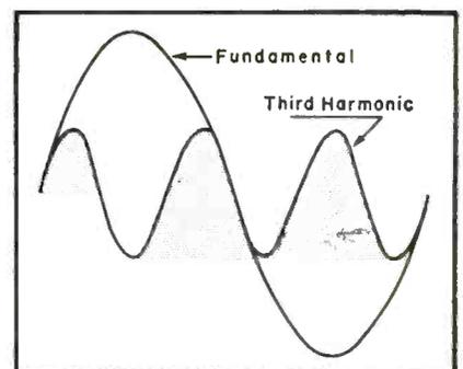
Fig. 4. In a square wave, phase relations are as important as the frequencies of the harmonics. An undistorted square wave displays harmonics going through zero at the same time as the fundamental goes through zero. If the 'scope amplifier shifts the phase of the harmonics, with respect to the fundamental, the reproduced square wave will show tilt.
