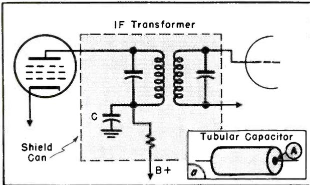
Fig. 1. Opening or shorting of capacitor C inside of an if transformer shield can is a common cause of intermittent operation. Poor connection at point A in capacitor can cause intermittent operation.
