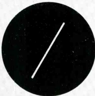
Phase shift between horizontal-vertical amplifiers, 0-100 kc-0°, to 1 mc within 2°; by internal adjustment with gain controls at max 0° phase shift possible on any specific frequency to 6 mc.
