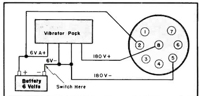
Fig. 2. Battery-operation plug and circuit.
