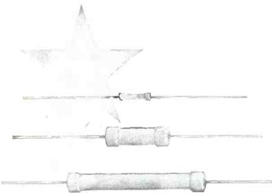
Notable performances of the Noblette resistors are—initial accuracy, excellent stability and moisture resistant. Available in 1/2, 1 and 2 watt; in resistance range of 1 ohm to 10 megohms. Standard tolerances of 1%.
