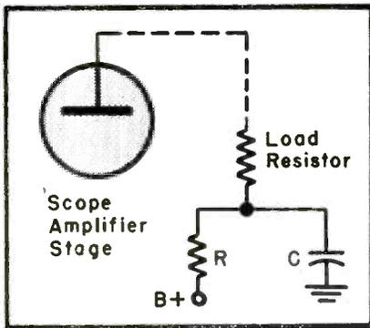
Fig. 10. Tilt, as seen in Fig. 5 (p. 21) can be compensated, and the 60-cycle square-wave response of the 'scope brought to the point shown in Fig. 2 (top—p. 20) by suitable adjustment of the values of R and C, the compensating resistance and capacitance in the 'scope-input stage.
