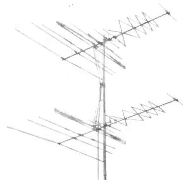
Helical yagi with front-end modification for peaking channel 13. Employs an added director and delta-matched helical section, and shortened stub at center of helix. Flat microwave helical section is composed of individual non-linear additive collectors, each tuned separately for one high band channel. Constructed of aluminum; preassembled. (Super-Star-Helix; JFD Manufacturing Co., Inc., 6101-16th Ave., Brooklyn 4, N. Y.)
