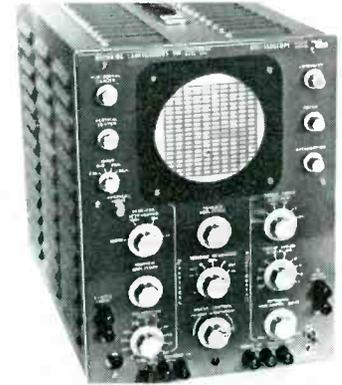
AC 'scope for 5 cps to 10 mc. Sweep circuits provide triggered or recurrent sweeps from 0.1 to 10,000 microseconds per centimeter. Internal 1-kc square wave is available for calibration and adjustment of attenuators and probes. Cathode follower outputs for external gate and sweep connections provide synchronization for auxiliary equipment. (Models 701 and 701-D; Browning Laboratories, Inc., 750 Main St., Winchester, Mass.)
