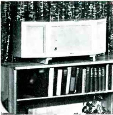
Three-way loudspeaker system with two tapered horn ports which load a coax-type low-frequency and mid-range reproducer from 70 to 3500 cps; very-high-frequency tweeter said to take over at 3500 cps to beyond audibility. Low-frequency and mid-range reproducer employs E-V Radax principle; large cone reproduces the lower frequencies and mechanical crossover is made to a smaller cone operating from approximately 1500 cps upwards. (Skyark; Electro-Voice, Inc., Buchanan, Mich.)
