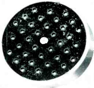
High impedance crystal tweeter that can be incorporated into plate circuit of output tube for wide-range response. Blocking capacitor in tweeter circuit is said to attenuate effectively the lower frequencies; frequency correction is in the form of a damping network tuned to resonant frequency of crystal, which damps resonance without decreasing sensitivity at other frequencies, is built into unit. Filter is an acoustic network. (Ronette Acoustical Corp., 135 Front St., N. Y. 5, N. Y.)
