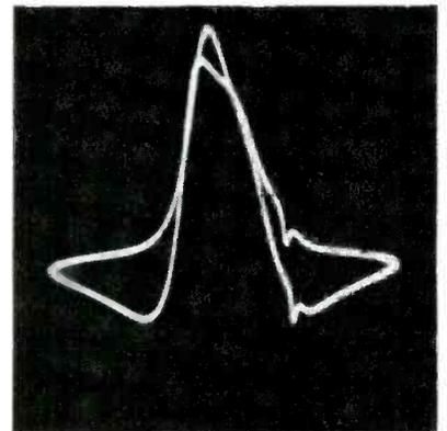
Fig. 6. If the 'scope amplifier introduces tilt into a reproduced 60-cycle square wave, it will introduce loop distortion into a reproduced response curve, as shown. Proper low-frequency compensation of the 'scope amplifier eliminates this difficulty. (From Technician's Timesaver.)
