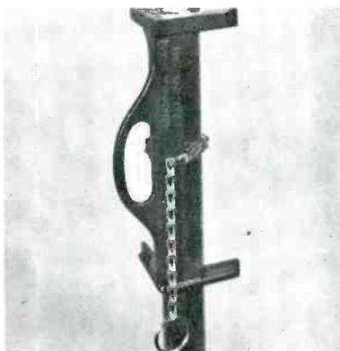
Bubble plumb for TV antenna-mast installations. Consists of two level vials mounted on right angle arms to enable operator to line any object vertically plumb. Right angle levels provide reference of all directions. Fastening devices permit attachment to objects 1/2" up to 4 1/2", round or square. Holds itself in place. Size is 4" x 10" overall; all-aluminum. (Clark and Newcomb, 305 Chapman St., Greenfield, Mass.)
