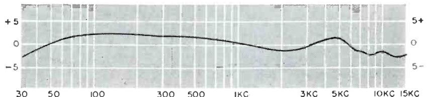
Response to new industrywide RIAA characteristic shows how 1P ceramic cartridge self-equalizes, because it works on "amplitude" rather than "velocity" principle. Here's startlingly improved performance for your customers' phonos!
