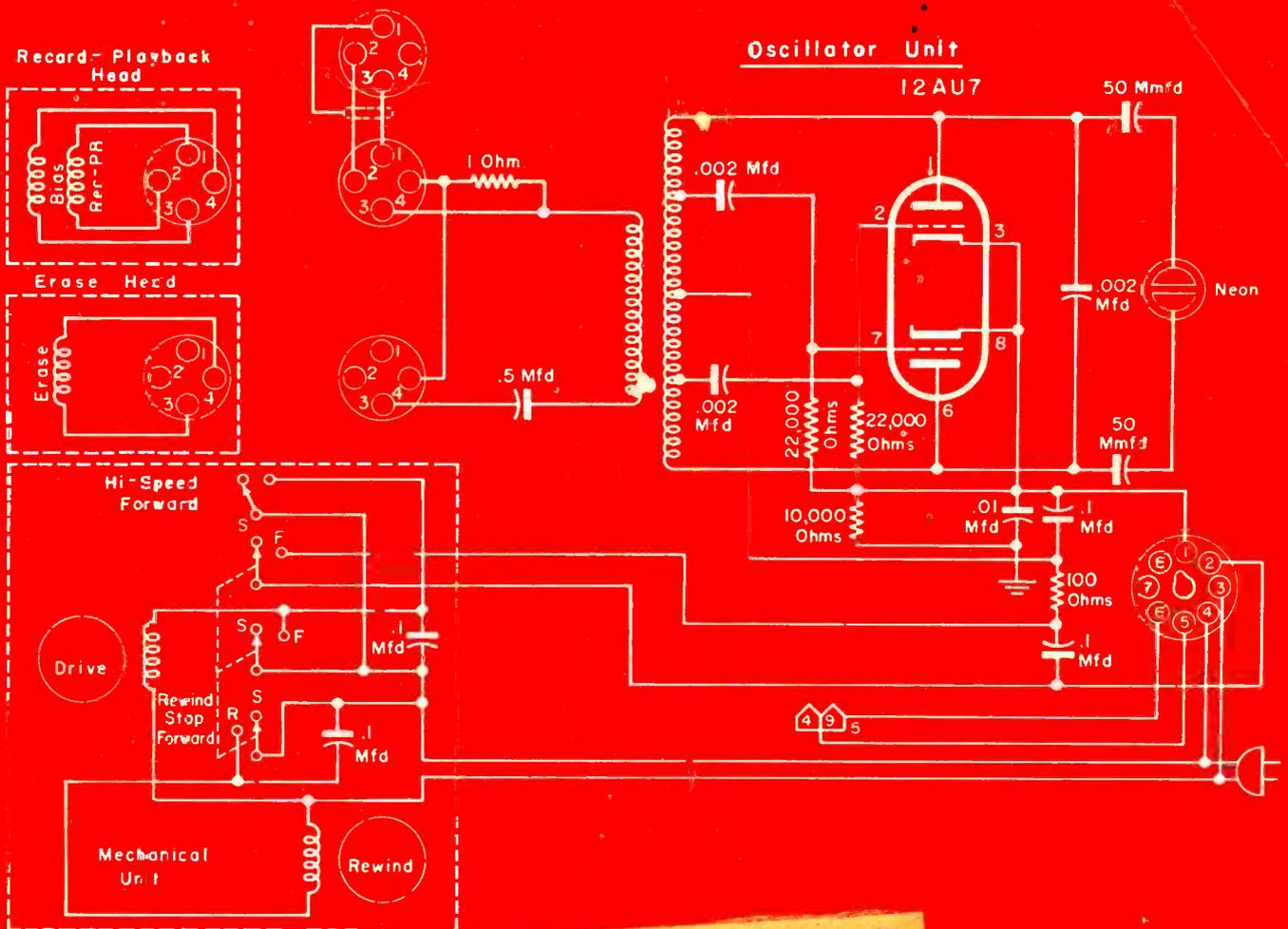
Oscillator section of two-speed tape recorder-playback unit. [See circuit analysis, this issue]
