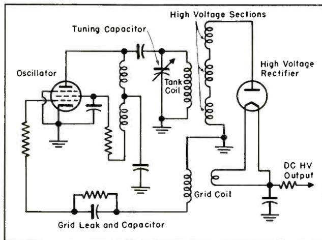
Fig. 2. Diagram of clamp type of feedback.
