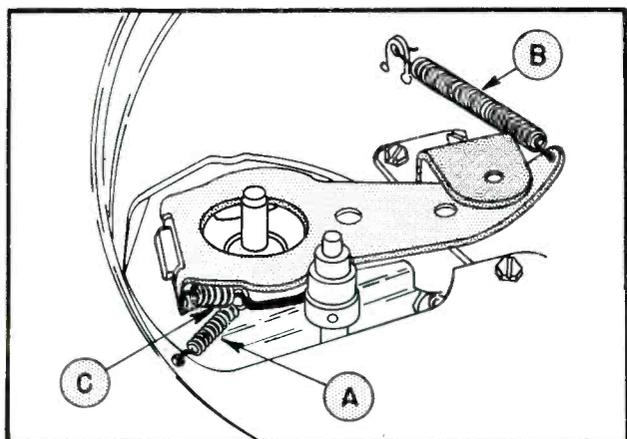
Cutaway view of Magnavox phono mechanism showing changes required to remove rumble and flutter. See illustration details on pages 55 and 76.
