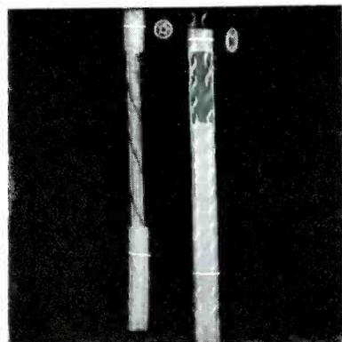
Transmission line designed for color-TV installations. Line has a star-shaped air-spaced former to equalize capacity of both conductors. (Twistube; Fenton Co., 15 Moore St., New York 4, N. Y.)
