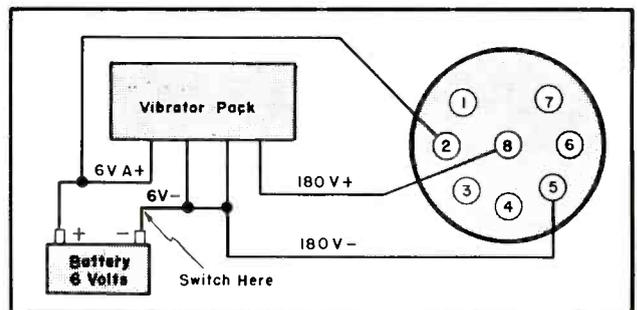
Fig. 2. Battery-operation plug and circuit.
