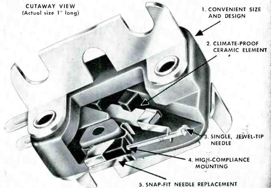
1. Easy to install. Just two models fit most arms now in use. Cartridge is less than 1" long, 8/10" wide with bracket. Time-saving hardware included.
