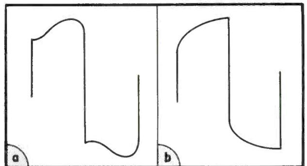
Fig. 8. Two typical examples of incorrect values of  $R$  and  $C$  in the low-frequency compensating circuit of the 'scope amplifier. When both  $R$  and  $C$  are properly chosen, the top of the reproduced square wave will be quite flat, and will exhibit no tilt.
