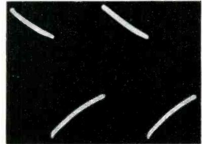
Fig. 5. Tilt in a reproduced 60-cycle square wave, due to shift in phase of the harmonics. A 'scope amplifier often shows this type of distortion, unless properly compensated. (From the Technician's Timesaver.)
