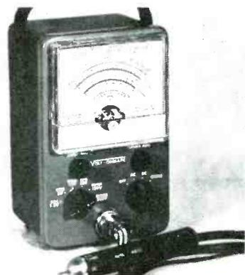
VTVM with automatic range switching said to eliminate manual selection of appropriate voltage or resistance range before use. Seven ac and dc ranges of 1.5, 5, 15, 50, 150, 500 and 1,500 v; seven peak-to-peak ranges of 4, 14, 40, 140, 400, 1,400 and 4,000 v; and ohmmeter ranges of X1, X10, X100, X1,000, X10K and X100K. Features 4 1/2" meter, 11-megohm input resistance (33 megohms on 1,500 v range). (Volt-Ohmatic; Bergen Labs, 11 Godwin Ave., Fair Lawn, N. J.)
