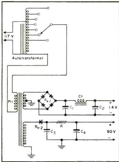
Fig. 1. Autotransformer and power supply used for testing battery radios.  $R_{x-1}$  is a bridge type selenium rectifier;  $R_{x-2}$  is a half-wave type.  $C_1$  and  $C_2$  are low-voltage filters, usually from 1,000 to 2,000 mfd, at 6 vdc.  $C_3$  and  $C_4$  are high-voltage filters running from 30-50 mfd at 150 v.
