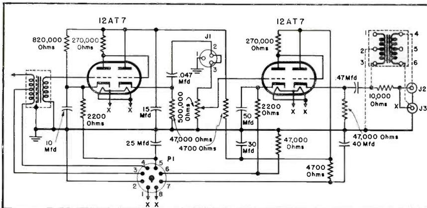
Fig. 1. Schematic of Stromberg-Carlson AV-52 preamp with a pair of twin triodes that serve as voltage amplifiers and cathode followers.
