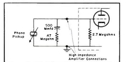
Fig. 2. Low-frequency equalization circuit for ceramic cartridge. The 2.7-megohm input resistance could be a volume control; in many high-impedance amplifiers such controls are employed.
