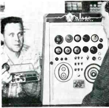
Assortment of phono and recorder drives included in a counter unit. Available too is a kit which includes 23 different drives, which it is claimed will serve to replace drives for 85% of changers now on the market. Some of the drives use neoprene rubber to negate losses due to hardening or cracking. (Walsco Electronics Corp., 3225 Exposition Place, Los Angeles 18, Calif.)
