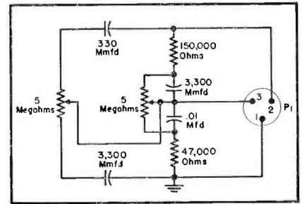
Fig. 2. Tone control developed for use with Fig. 1 preamp; Stromberg-Carlson AK-11.
