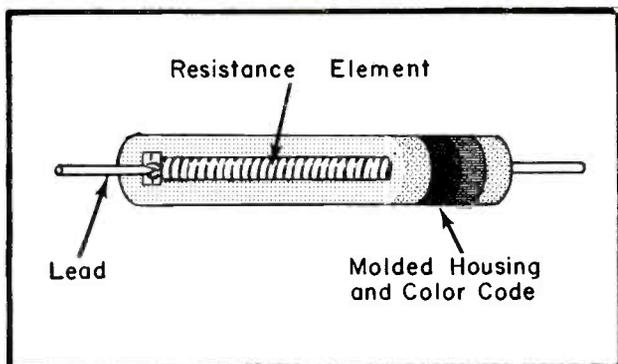
Fig. 1. Molded wire-wound resistor construction.
