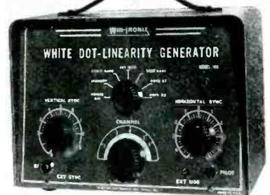
White dot linearity generator for black-and-white or color-TV. Features large and small dots for color receiver convergence and vertical and horizontal bars for sweep circuit alignment. Internally generated vertical sync pulses are locked to line frequency for stable operation. Has rf carrier output and external modulation. (Model 160; Winston Electronics, Inc., 4312 Main St., Philadelphia 27, Pa.)
