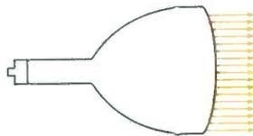
**MAGIC-MIRROR ALUMINIZED TUBE**—Aluminized reflector allows electron beam through. Blocks wasted light from backing up into tube. Reflects *all* the light into picture.
