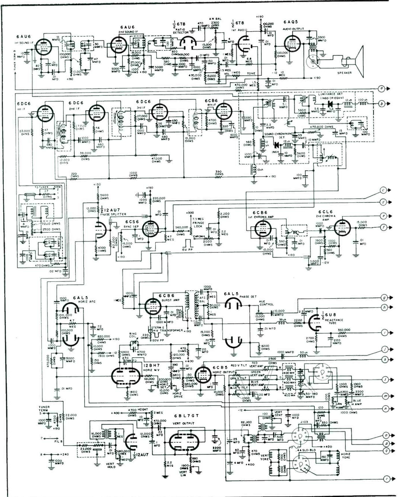
Complete circuit of the Capehart CXC-13 series color chassis. The cathode-coupled color demodulators in the chrominance-
