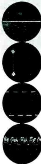
No signal... a stable sweep condition provides reference trace
