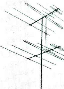
**Inline broad-band 2-bay antenna**, incorporating reverse-phase multiplex dipole system, and said to be custom tailored for areas with cochannel and cross-channel interference. Unit is wide stacked at a spacing of 68", and coupled with 68" hi-band rejection transformers; recommended for channels 7 to 13. (Model FB500S-68; JFD Manufacturing Co., Inc., 6101 16th Ave., Brooklyn 4, N. Y.)
