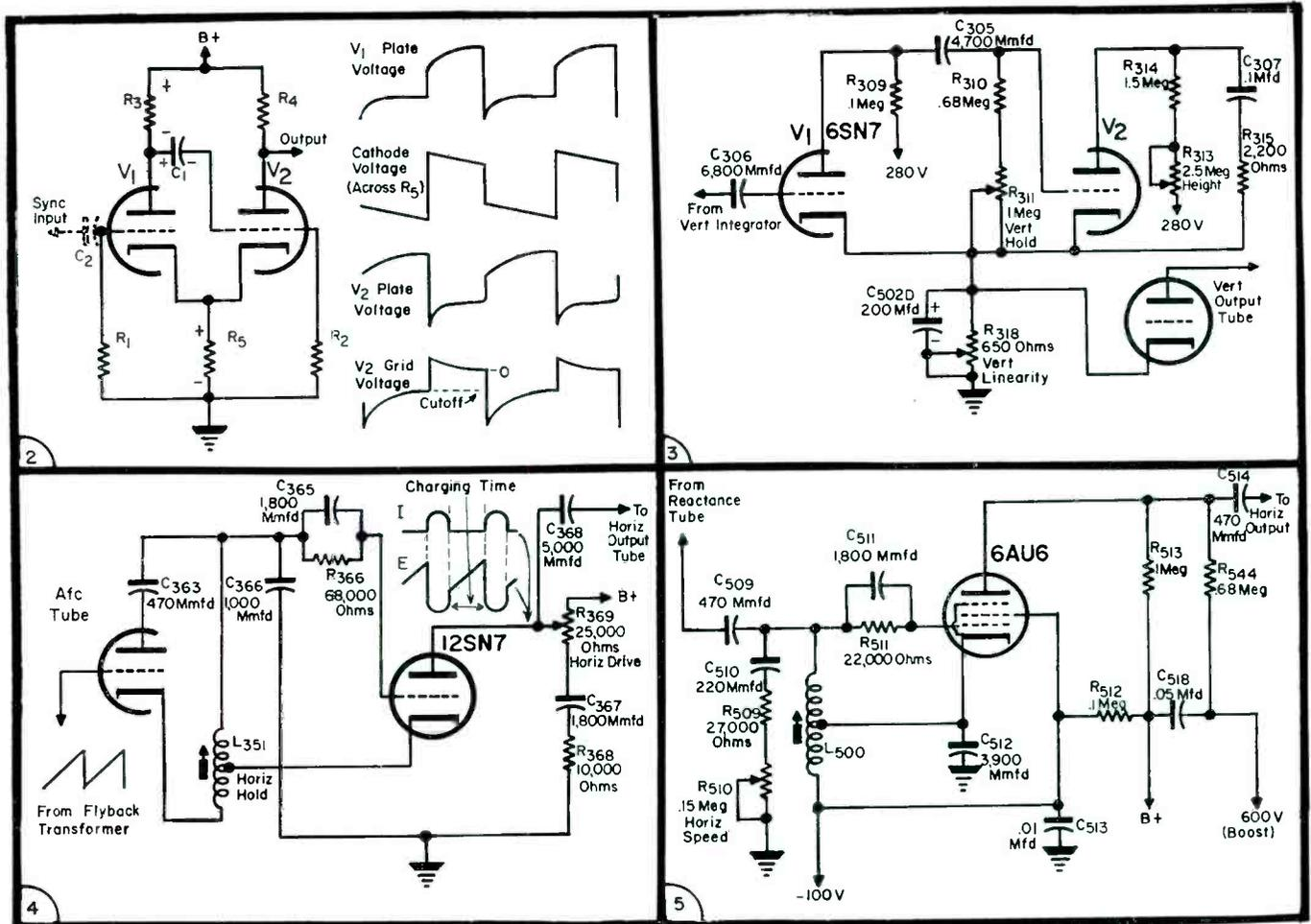
Figs. 2 to 5. The schematic of a cathode-coupled mv used for a vertical oscillator, with resultant plate voltage waveforms at right, is shown in Fig. 2. A typical vertical oscillator cathode-coupled mv circuit used in Magnavox 105L appears in Fig. 3. The Martley oscillator used in G.E. model 17C113 is diagrammed in Fig. 4, and in Fig. 5 we have another form of oscillator, the electron-coupled type, used as a horizontal oscillator in G.E. model 24C101.
