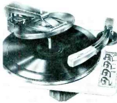
Record changer powered by a direct-drive motor utilizing a separate gear for each standard speed. Has dial-action control knob for selecting three standard speeds. Concentric with dial, is a fine-tuning knob, said to permit pitch adjustments within a 5% latitude above and below each of standard speeds during audition. (Model CD-43; Thorens Company, New Hyde Park, L. I., New York.)
