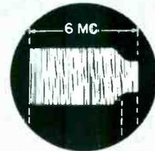
Note flatness throughout specified range; to 3.6 mc down 1.5 db, at 4.5 mc down 3 db, at 5 mc down 6 db.
