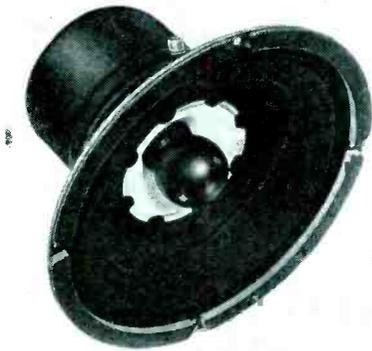
Eight-inch speaker featuring a phase-equalizing globe, and elliptical corrugation of cone. Has separate tweeter and woofer cones, coaxially mounted with a mechanical crossover. Spider is of coaxially-corrugated thin fiber. Voice coil is of aluminum. (Matsushita Electric Panasonic; R. I. Mendels, Inc., 41 E. 42d St., N.Y. 17, N.Y.)
