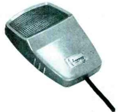
Tape recorder microphone, also said to be suitable for paging systems and general purpose work. Available with either shielded crystal or ceramic elements. Crystal type has a response of 100 to 7000 cps and an output of -55 db; ceramic type has a response of 100 to 6,000 cps and an output of -62 db. Impedance is high in both types; they are omnidirectional. Size: 3/4" x 2 1/8" x 15/16". (American Microphone Co., 370 S. Fair Oaks Ave., Pasadena, Calif.)
