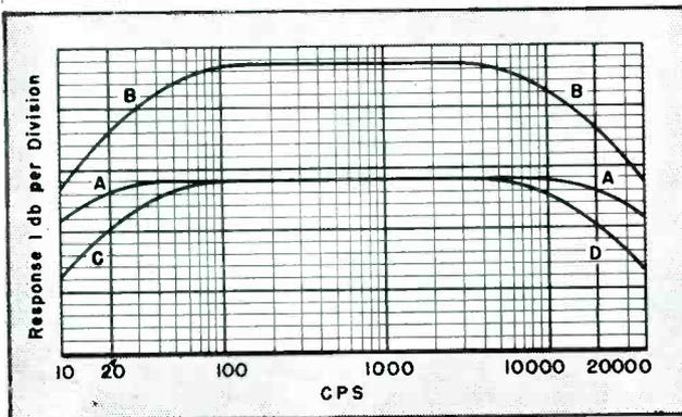
Fig. 2. Effect of different values of loading resistance in the input of a ribbon or moving-coil cartridge; A, correct value; B, no loading resistance, or value too high; C, value too low.
