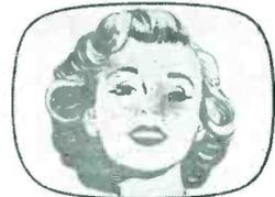
**RESULT**—A light background within the tube which reduces picture contrast.
