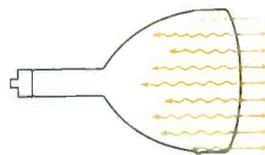
**ORDINARY TUBE**—Only *half* the light produced by the phosphor screen is utilized in the picture. Other half radiates wastefully back into tube.
