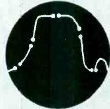
Response curves accurately displayed. Ideal for use with Weston intensity marker display. A fast, retrace sweep circuit with cathode follower output prevents pattern distortion.
