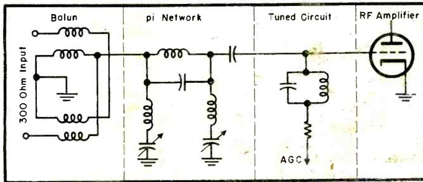
FIG. 1: ANTENNA matching network and its relation to tuner circuitry.
