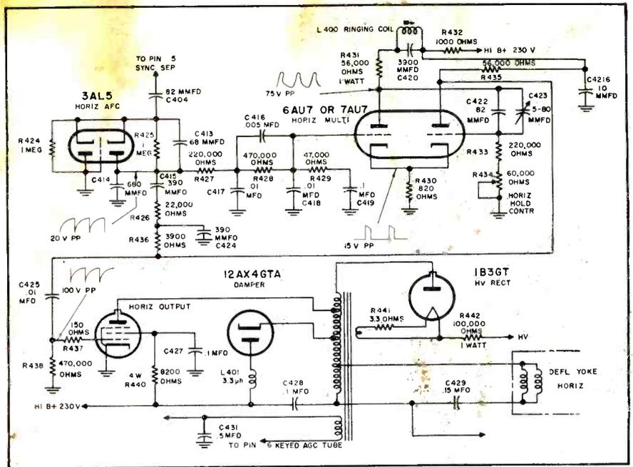
FIG. 2: WESTINGHOUSE horizontal sweep circuit.
