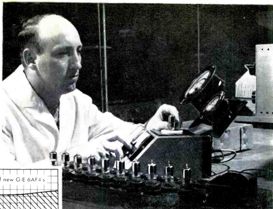
ABOVE: General Electric Design Engineer J. G. Tucker checks, for oscillator activity, new G-E 6AF4 tubes that are undergoing life test. LEFT: Effect of tube operation over long periods on new vs. standard 6AF4's is shown by the chart. Tests of many thousand tubes are represented. Note that the oscillator activity of new G-E 6AF4's averages a straight horizontal line, whereas standard 6AF4's show a sharp, sudden drop . . . meaning rapid loss of picture quality.
