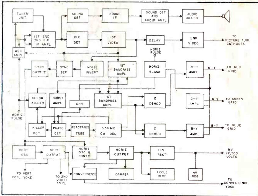
FIG. 1: BLOCK DIAGRAM of the complete RCA CTC7 color-TV chassis.
