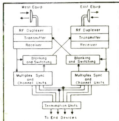
**REPEATER** with multiplex and termination units. Additional equipment required for this phase of operation is a blanking and switching unit.
