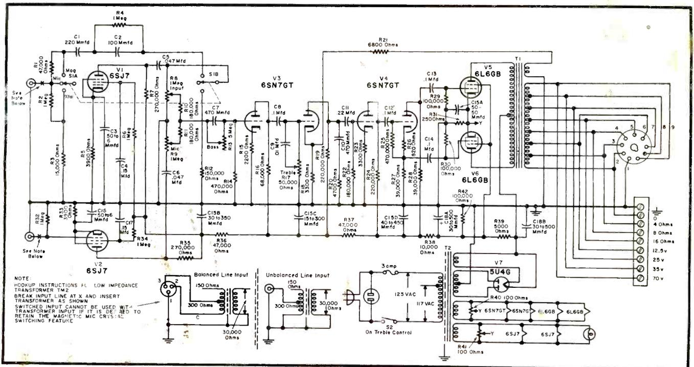
**SCHEMATIC OF STROMBERG-CARLSON amplifier included in Trenholm sound-system installation.**
