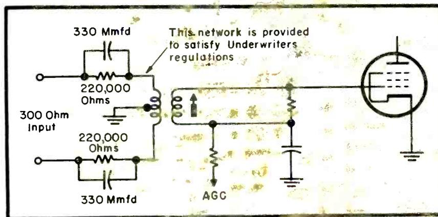
FIG. 2: TYPICAL TUNER input circuit using a matching transformer.
