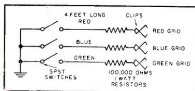
FIG. 1: SWITCHING CIRCUIT designed to permit biasing off of one or two guns in the color tube, when adjusting purity or convergence.
