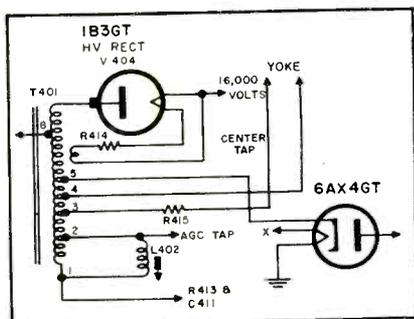
FIG. 3: MODIFIED HIGH-VOLTAGE TRANSFORMER connections in Magnavox chassis. The *agc* keying pulse is now obtained from the top of the horizontal width coil.
