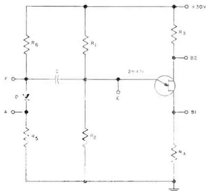
**BASIC CIRCUIT** for silicon unijunction transistor. Values of  $R_1$  may vary from 2200 to 390,000 ohms;  $R_2$ , 820 to 5600 ohms;  $R_3$ , 330 to 47,000 ohms;  $R_4$ , 10 to 250 ohms; and  $R_5$ , 10 to 100 ohms, depending upon function.
