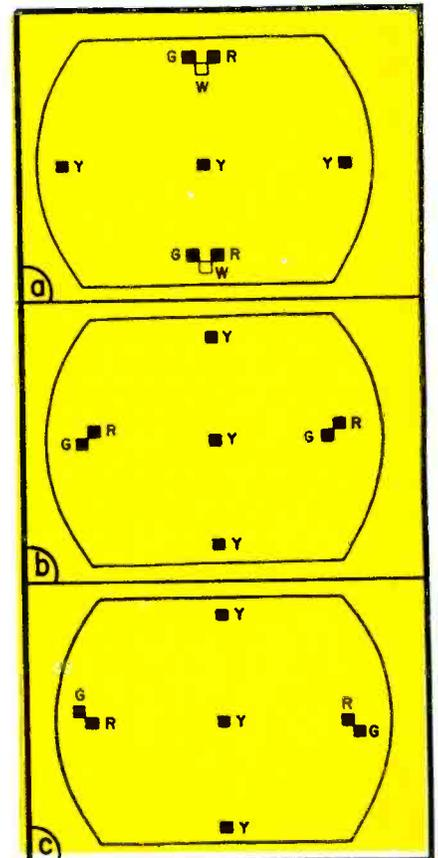
FIG. 3: CONVERGENCE RESULTS when (a) the green and red vertical amplifier is off (red and green are not crossed), (b) red horizontal amp is off and (c) green horizontal tilt is off.
