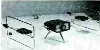
**INDOOR TV antenna with a disappearing dipole to boost low-band performance and a parasitic reflector to aid high-band performance. Features a 12-channel variable inductance tuning system for channel selectivity. Rotates in all directions on a tripod. Total height is 6'. — Super Showman; Channel Master, Ellenville, N.Y.**
