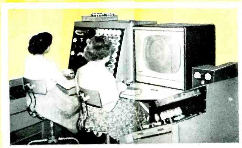
New heater-cathode design helps Sylvania damper types pass this dynamic arc test with flying colors. Dynamic tests such as this have now been instituted by Sylvania on all important types in every
