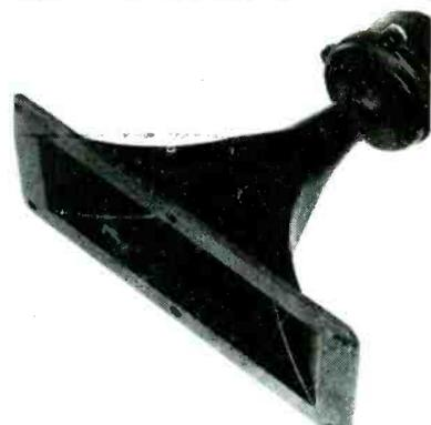
**TWEETER**, with a program-capacity power of 35 watts, said to provide a wide angle distribution pattern throughout 2,000 to 17,500-cps range. Diaphragms are checked for weight and compliance to assure functional uniformity in production. Impedance is 12 to 16 ohms. Cabinet opening required is 6" x 2".—Model HR-3; Atlas Sound Corp., 1451 39th St., Brooklyn 18, N. Y. [SERVICE]
