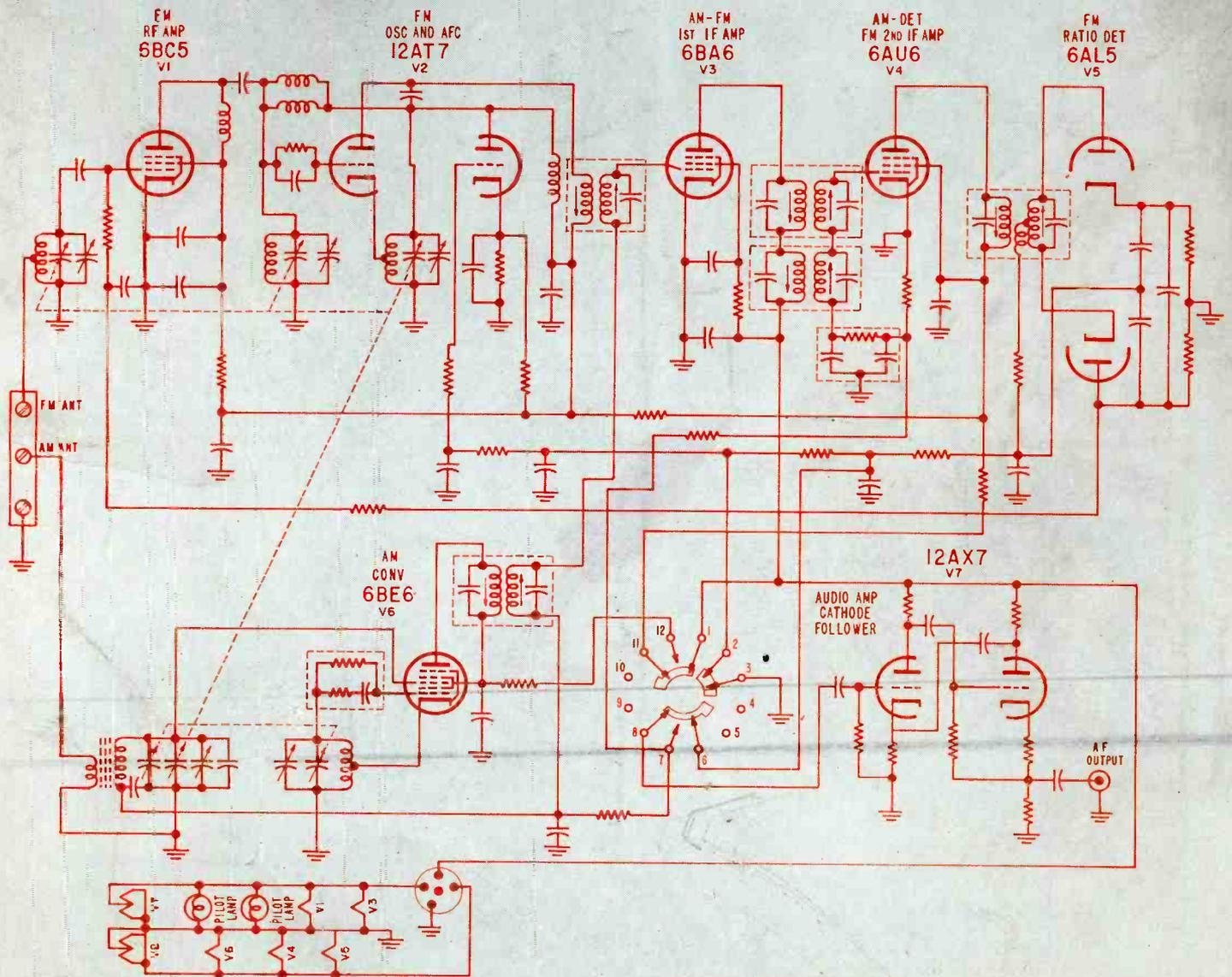
AM-FM tuner designed for remote-control 3-speaker radio-phon consolette.
