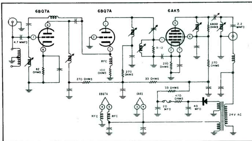
**CIRCUIT** of FM antenna preamplifier.
