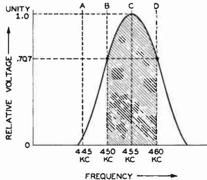
Fig. 3. The shaded area under this selectivity i-f transformer curve indicates portion where full reproduction of sidebands occurs.
