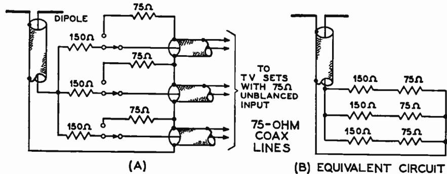
Fig. 3. Connections for two, three, or four television sets with 75-ohm unbalanced inputs to a dipole. Note that the value of the series resistors changes with the number of sets used.
