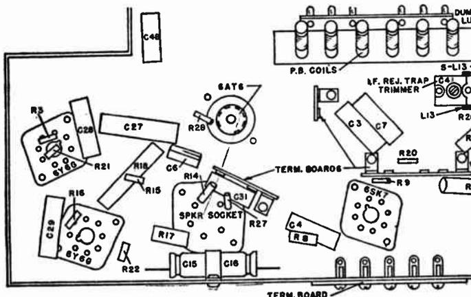
Changes in the tone control circuit, above, and in the parts layout, left, of the Westinghouse Chassis V-2102-2.
