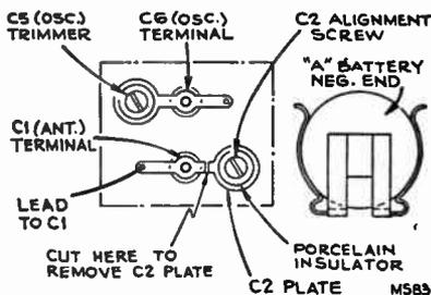
Before aligning the RCA model 54B with a "cemented" loop, C2 is removed, as indicated.
