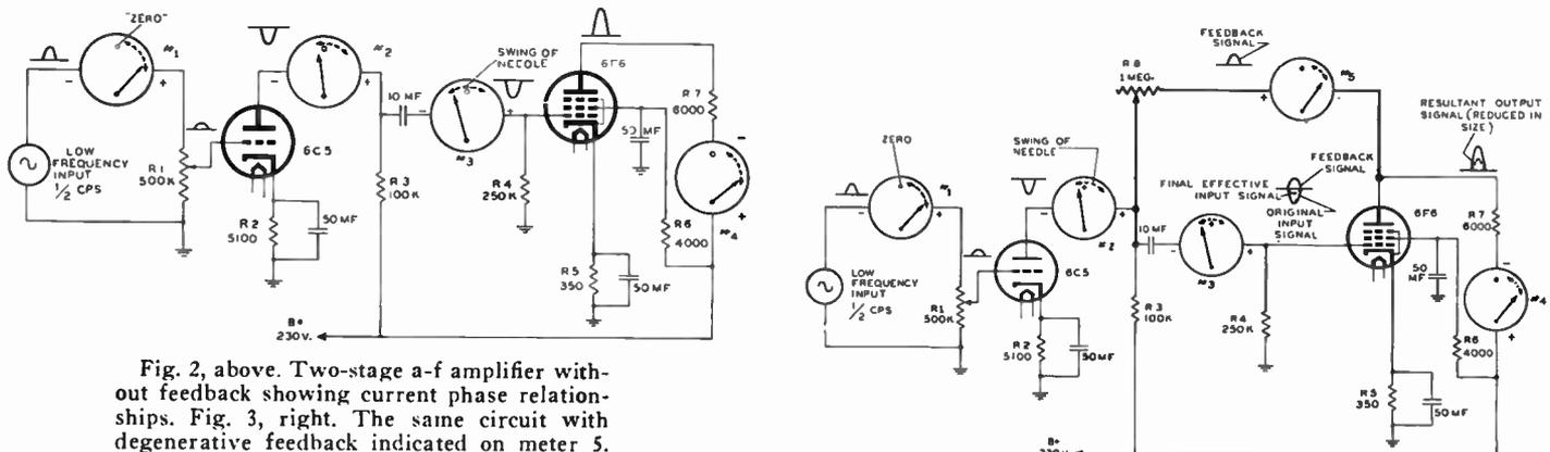
Fig. 2, above. Two-stage a-f amplifier without feedback showing current phase relationships. Fig. 3, right. The same circuit with degenerative feedback indicated on meter 4.
