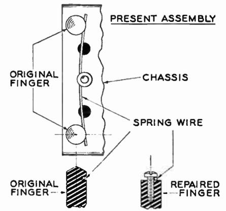
A machine screw can be substituted for the broken head of the finger which catches the spring wire holding chassis of Satchell Carlson 427 in cabinet.
