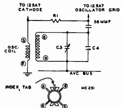
Alternate oscillator coil in RCA 65X.
