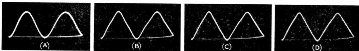
**TRIANGULAR WAVE.** A cosine wave (A) of fundamental frequency  $F$  and an amplitude  $V$ , can be made into a triangular wave by adding its odd harmonics all in phase having amplitudes equal to the reciprocals of the square of the harmonics.
