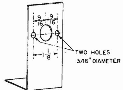
The holes that must be drilled in the speaker bracket of the Crosley 307TA to accommodate a p-m speaker.
