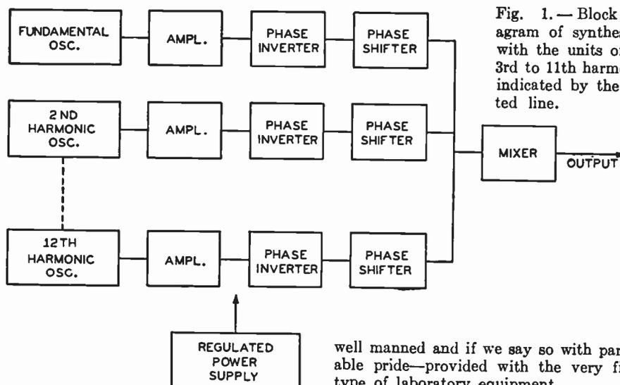
Fig. 1.—Block diagram of synthesizer, with the units of the 3rd to 11th harmonics indicated by the dotted line.
