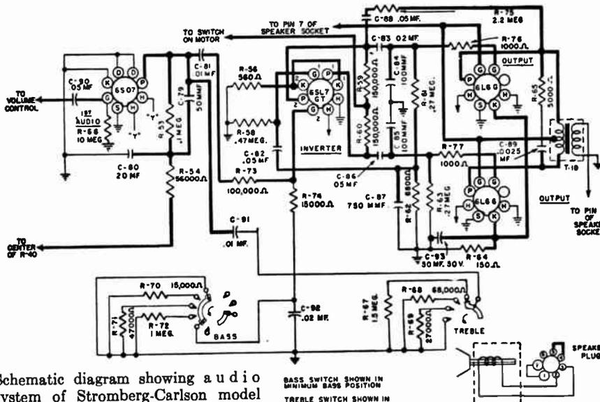
Schematic diagram showing audio system of Stromberg-Carlson model 1235 in which it differs from 1135.
