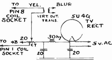
The change in the power supply of the Remington 80 and 130 to produce the necessary centering voltages.
