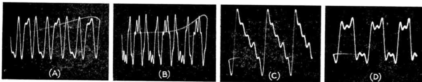
**COMPLEX WAVES.** The composition of a complex wave consists of a fundamental frequency with the addition of certain harmonics of various amplitudes which are in certain phase relationships to the fundamental.
