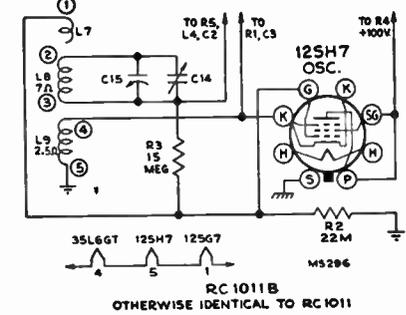
Changes in the oscillator circuit of RCA Chassis RC1011A, above, and Chassis RC1011B, below.
