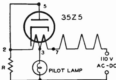
Burnout of pilot lamps is sometimes caused by the burnout of a portion of the 35Z5 in ac-dc sets.
