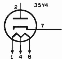
Correct pin numbers for the 35Y4 tube in the Teletone Model 117 schematic.
