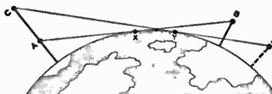
Fig. 1. The line of sight is shown between the antennas at *A* and *B*. If *A* were raised to position *C*, the line of sight would be increased to *D*.
