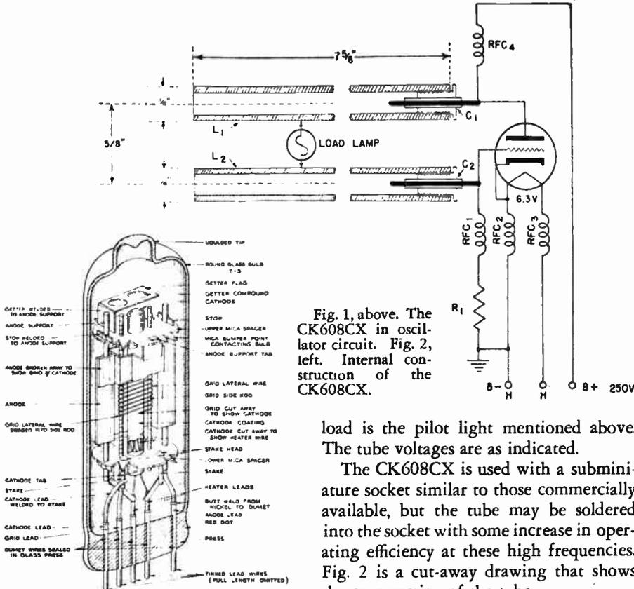
Fig. 1, above. The CK608CX in oscillator circuit. Fig. 2, left. Internal construction of the CK608CX.
