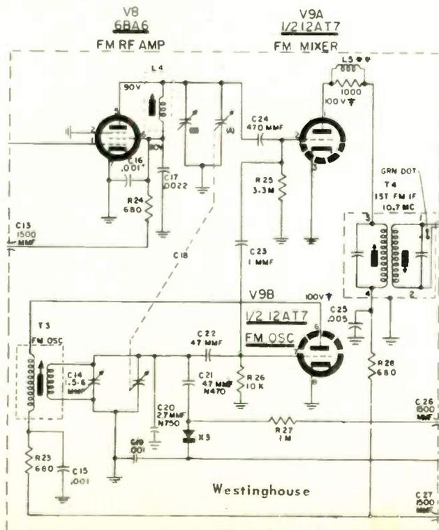
both AM and FM by using a double IF coil in the plate circuit. One will respond to the AM IF, and the other to FM IF. Fig. 5 shows such a circuit.
