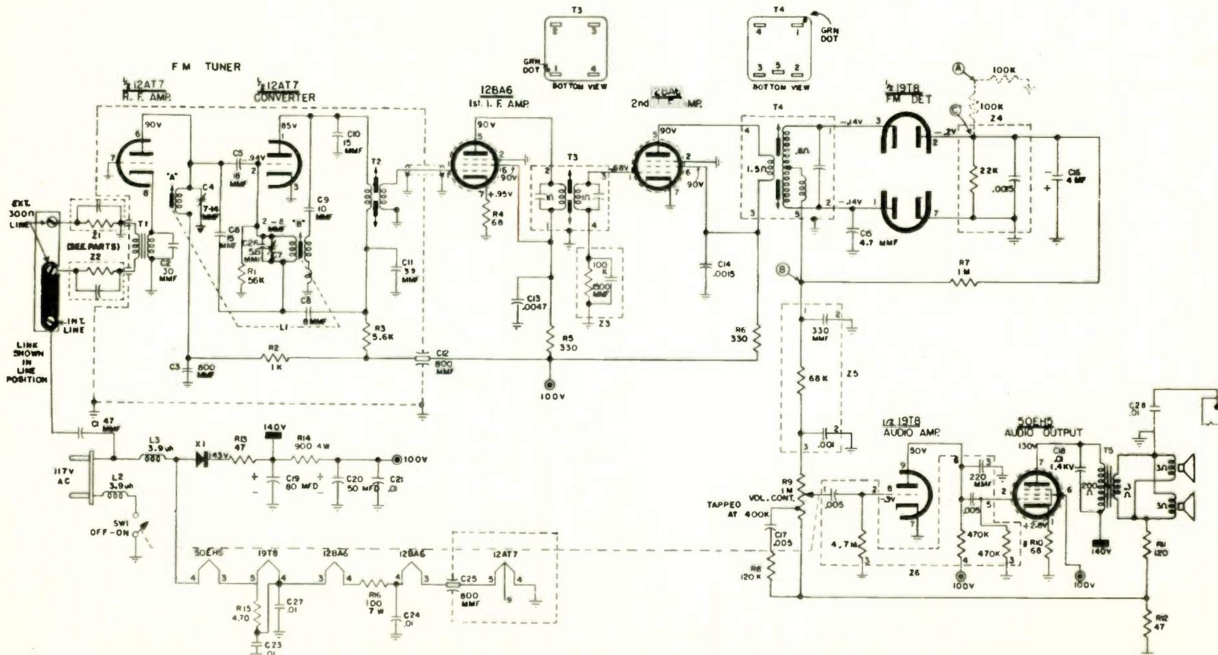
1. VOLTAGES TAKEN WITH A VTVM FROM POINTS INDICATED TO B. TUNING INDUCTANCE AT MAXIMUM. VOLUME CONTROL AT MINIMUM. LINE VOLTAGE AT 117V AC. NO SIGNAL INPUT.
