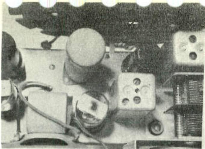
WHEN SOME TUBES LIGHT AND OTHERS DO NOT IN AN AC/DC RECEIVER, THE TROUBLE MUST BE DUE TO SOME SHORT IN THE FILAMENT LINE. MOST COMMON IN THIS TYPE OF TROUBLE, IS A HEATER TO CATHODE SHORT INSIDE ONE OF THE TUBES. THIS SHORTS OUT PART OF THE FILAMENT LINE, SINCE THE TUBES ARE ALL IN SERIES, AND SOME OF THE TUBES WILL NOT LIGHT. THE REMAINING TUBES IN THE SET WILL BE OVERHEATING DUE TO THE EXTRA VOLTAGE ON THEIR FILAMENTS.
