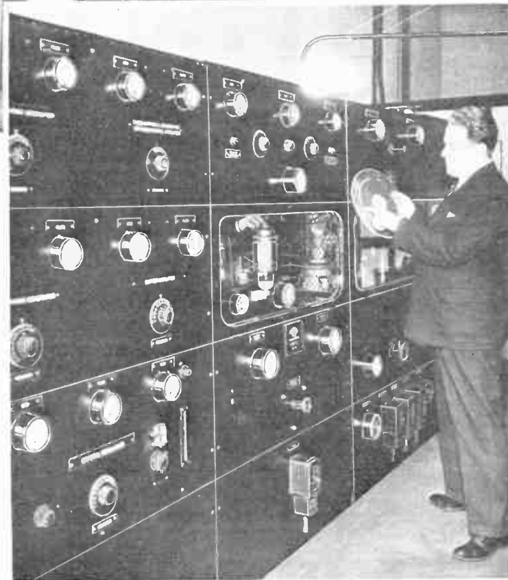
Above—a view of the 5,000 watt short-wave transmitting equipment installed at station WIXAL, from which the new and very ambitious "higher education" programs are being broadcast. Mr. Lemmon is shown at right of the picture, inspecting an electrical transcription record.
