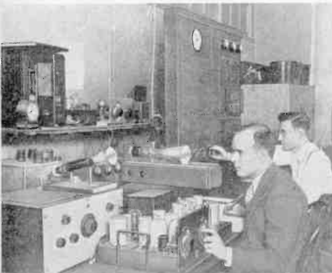
Fig. 3—Keeping a visual check on the program by the use of Cathode-Ray Tubes.
