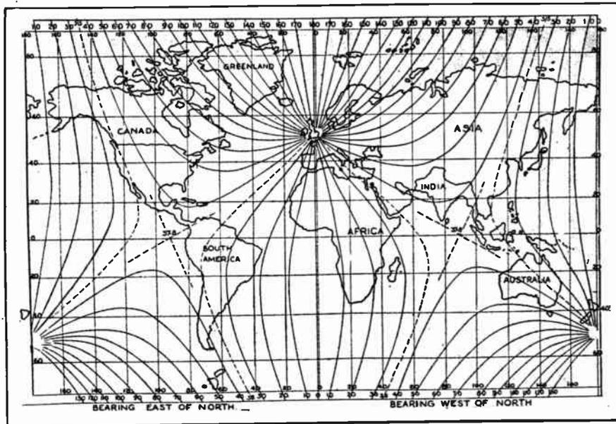
A map of the world, the curved lines on which show the bearing or the direction of the Daventry (England) short-wave broadcasting station from any point.
