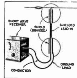
Shielded lead-in in many cases reduces man-made interference.
