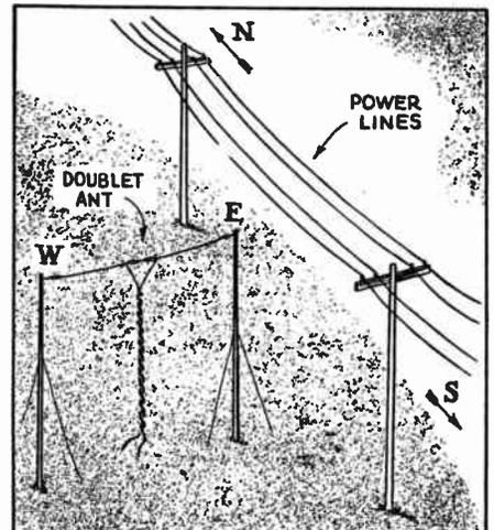
The doublet should be at right angles with power lines.
