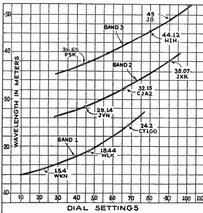
Calibration curves plotted on a cross-section paper enable you to quickly find stations when only their frequency is known.
