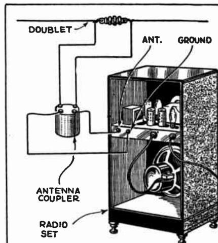
The doublet antenna can be connected to any set, providing the proper transformer or coupler is used.
