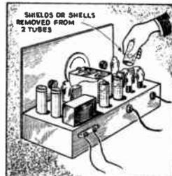
Removing one or two tube shields makes set more sensitive.
