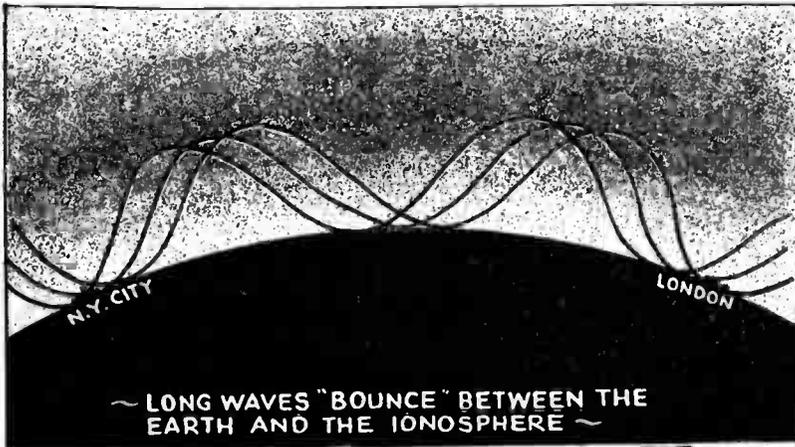
Long waves are transmitted over great distances, such as between New York City and London, by being constantly reflected back and forth between the surface of the earth and the highly ionized upper atmosphere.
