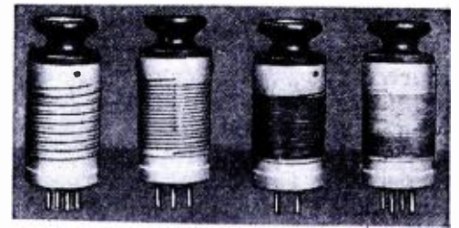
Photograph of the set of coils used by the author with the Super Dynatron receiver. They are wound on Isolantite forms for high efficiency.
