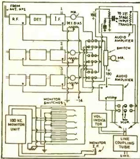
Below (Left)—Diagram of heterodyne tuner unit used in picking up transatlantic rebroadcast high frequency waves.
