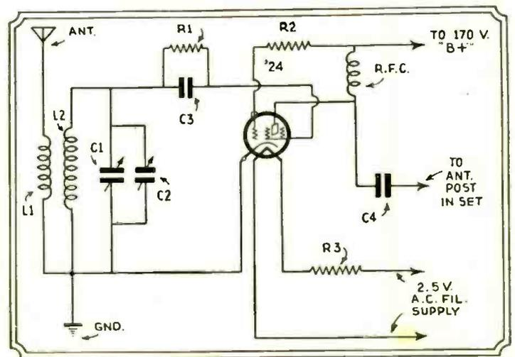
Wiring diagram for the "third-prize" short-wave converter.
