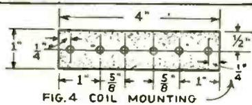
FIG. 4 COIL MOUNTING
