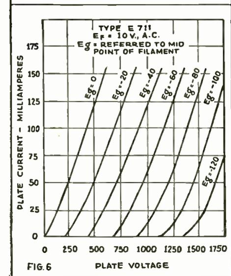
Fig. 4 shows socket connections for the Arcturus tubes; Fig. 5 (center) shows curves for the E703A tube and lower graphs, Fig. 6, show performance of the E711A.
