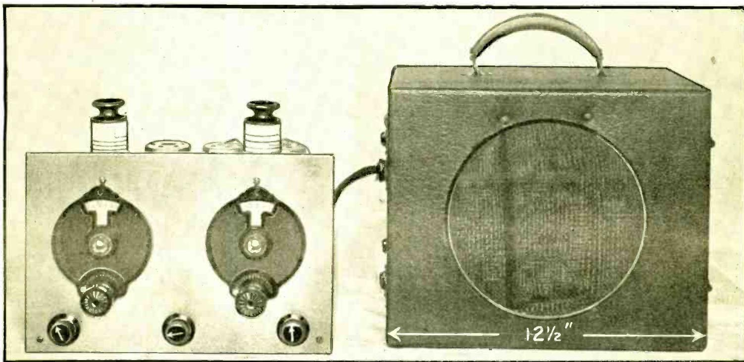
This portable 8-tube superhet has the weight divided into two cases, one containing the batteries and loud speaker.
