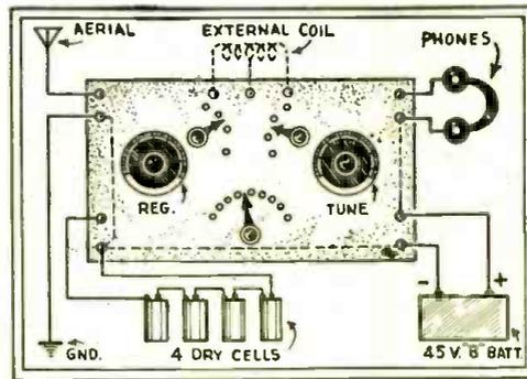
Fig. 2—Front panel view of amateur's short-wave receiver with vacuum tube, batteries and phone hook-up.
