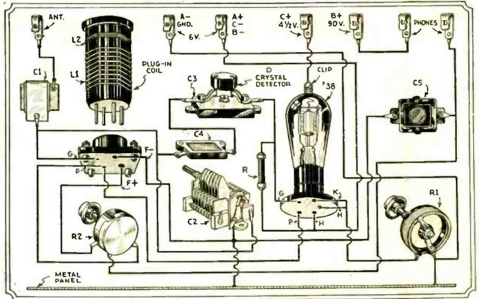
space-charge regenerative detector; that is, the control grid is connected to a plus potential of 6 to 10½ volts with respect to the negative side of the filament or cathode and the screen-grid is then used as a control grid. The plate potential may be 90 volts, although as low as 45 gives satisfactory results. These voltages may vary when other types of tubes are used.
