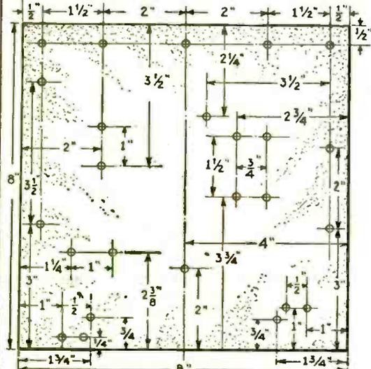
FIG. 3 BASE BOARD LAYOUT (ALL HOLES 1/8" DIA.)
