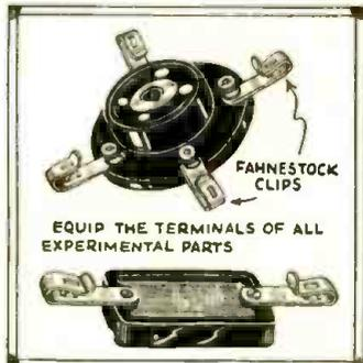
connections from one point to another by screwing and unscrewing thumb-nuts (in the life of an experimenter about every ten seconds) try the following kink: Equip the terminals of all your experimental parts (sockets, coils, rheostats, etc.) with Fahnestock clips. The parts thus equipped may be mounted bread-board fashion and minor circuits or complete circuit changes may be made quickly and without trouble.—M. C. Alexander, Jr.
