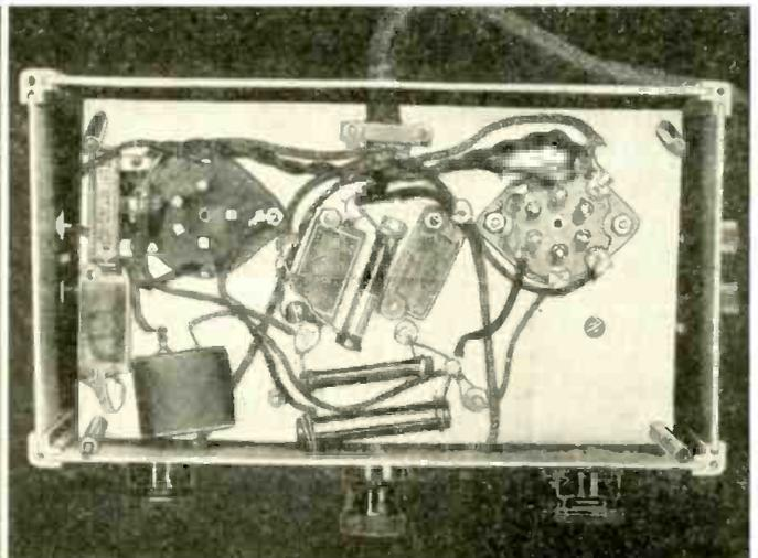
The photos above show interior as well as bottom views of Mr. Shuart's very neat receiver job—a 2-tube "high gain" A.C. operated set, with "band-spread" features. It employs a 58
