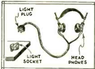
Use an electric light plug for a phone jack and a light socket of the prong type. I find it just as good. Solder one end of the lead from the plug to one of the screws of the phones to one of the other lead. Using a double-throw, single-pole switch makes a good way to switch the aerial to the ground, when not using the aerial for the set.—Warren W. Smith, Jr.
