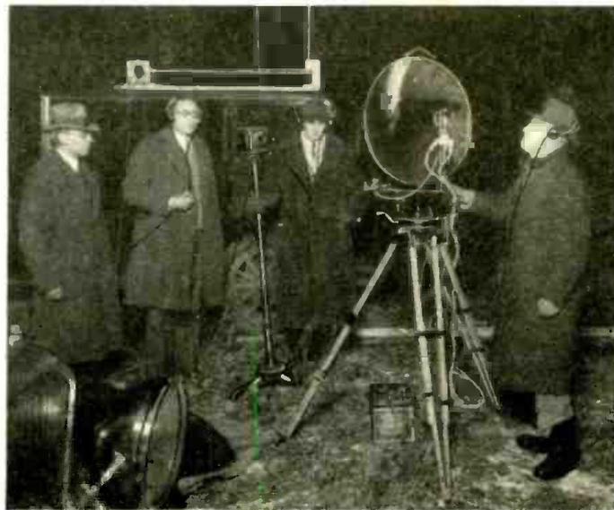
other scientists of the General Electric Company. They had a 36-inch reflector, at the focus of which was mounted a light-sensitive phototube. Accurate adjustments of the beacon and receiver established the contact. The phototube equipment, responding to the
