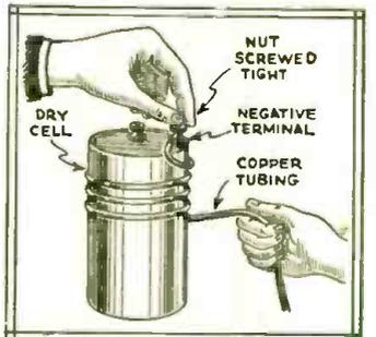
Wind your copper tubing coils on an old dry-cell. First flatten the end of copper tubing, drill a hole through it and slip over binding post. Wind the required turns while the other end is pulled tight in a vise or held by someone.—Floyd Gribben.
