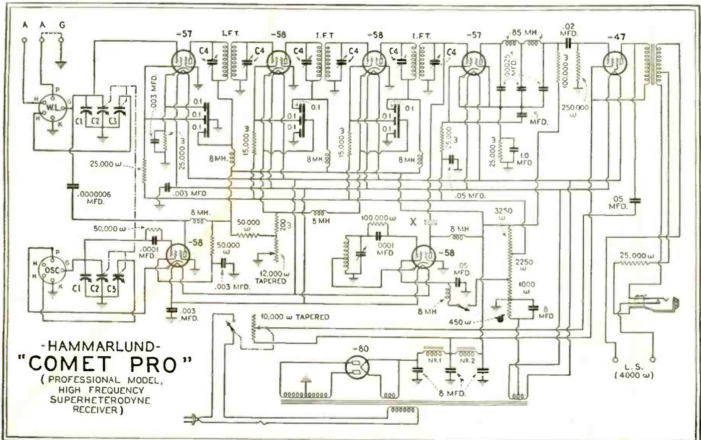
Diagram of connections as used in the latest "revised" model of the Hammarlund Comet "Pro" short-wave superheterodyne receiver. This set uses 8 tubes, including an 80 type rectifier. Fig. 1.
