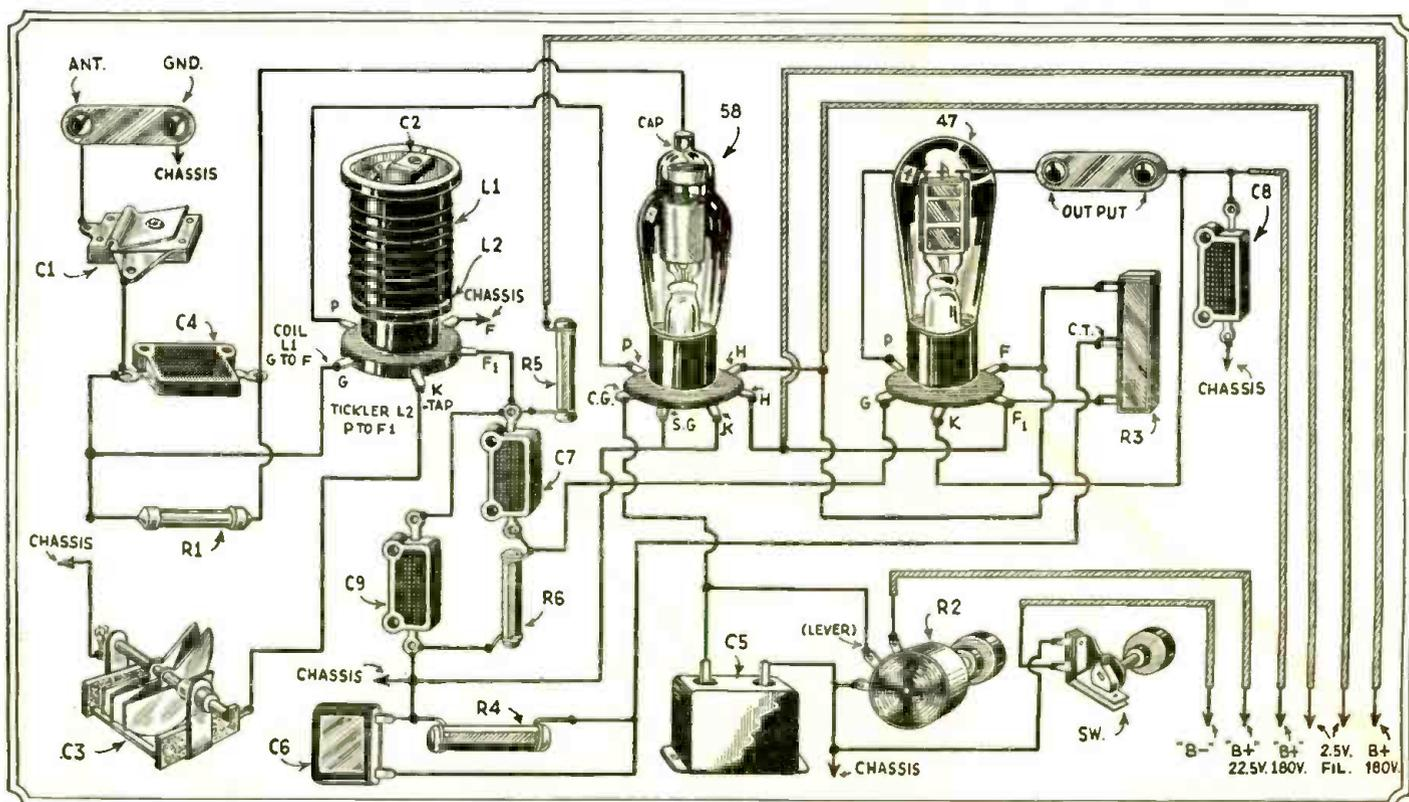
Picture diagram especially suited to the lay reader, who is not so familiar with schematic wiring diagrams. The cost of building this 2-tube receiver is very nominal indeed.
