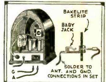
cord tips on the leads instead of the bare wire. The two baby jacks were put onto a small strip of bakelite as shown in sketch above and soldered to the antenna and ground connections in the set. Now it is a simple matter to yank these connections out of one set and plug them into the other.—J. T. Watkins.
