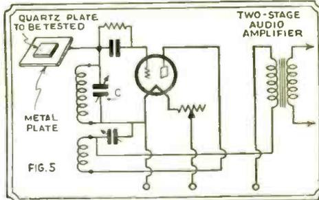
Arrangement for testing quartz crystals.
