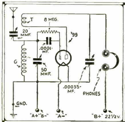
Wiring diagram for the 1-Tube battery-operated S-W Receiver.
