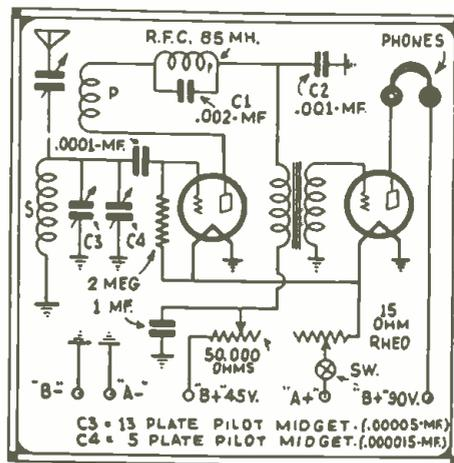
● This two-tube instrument, operated by batteries, was designed to provide a compact, portable, smoothly operating short wave automobile or station receiver.
