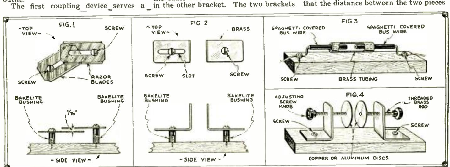
Fig. 1, at left, shows how to make an antenna coupling condenser from old safety-razor blades. Fig. 2—Another simple and practical design involving the use of two right-angle brass or other metal members, one of which is slotted for adjusting
