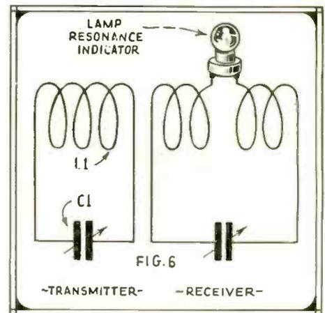
Fig. 6—Experimental receiving circuit employing a small lamp as the resonance indicator.
