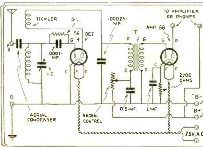
Wiring diagram showing schematically how the new A.C. heater circuit is applied to the short-wave "Beginners' Receiver," previously described for battery operation.
