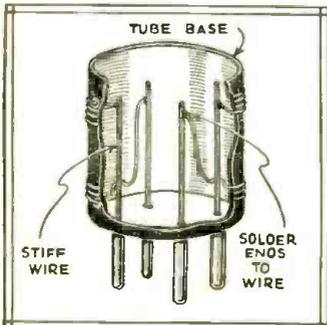
In making short-wave plug-in coils I have found an easier method of fastening the ends of the coils to the prongs of the coil form or tube base. For UX bases take four pieces of stiff wire (as tall as necessary) just large enough to fit tightly into the prongs of the form and solder the ends of the coils to the wire. For UY use five wires, etc.—Hurry F. Steber.
