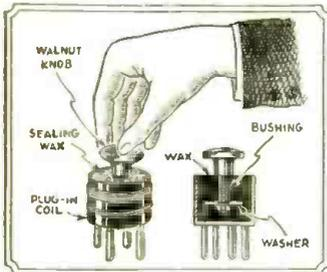
A very good handle for tube base coils can be made from a common walnut knob, the variety sold in the Five-and-Ten-Cent stores; a flange washer and a brass bushing. Remove the nut on the knob and slip on the bushing, which should be about 1/2" long; next, the washer, and finally the nut. Tighten the whole thing and the handle is ready for use.
